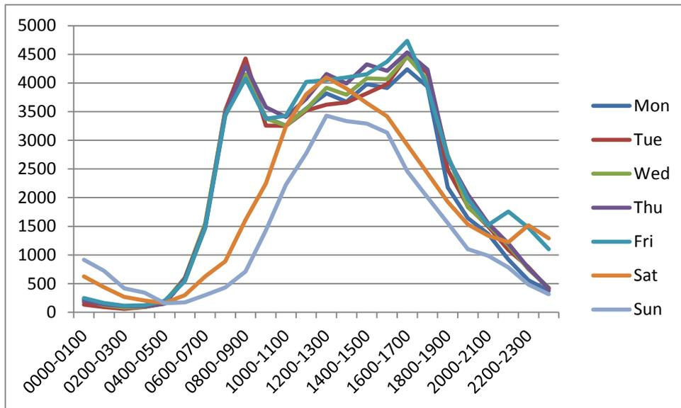
68 The graph shows the hourly traffic volume on the Y axis and the time-of-day on the X axis with a line for each day of the week. This is useful for determining a range of aspects;
