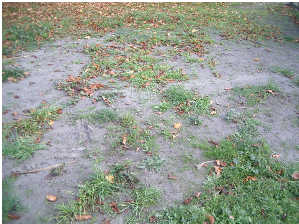
■ Figure 17 - Ejected sand
