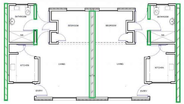
Figure 7: Walls used for bracing in the longitudinal direction.
