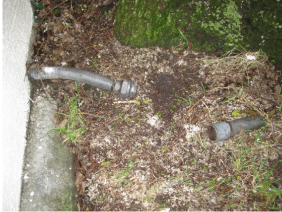
Photo 21: Disrupted connection on east side of pumphouse.
