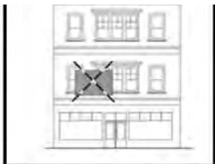
3. Sign conflicts with architectural features
