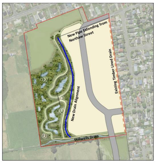
Figure 10. Realignment of Timer Lined Drain
