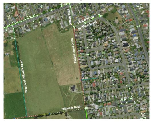
Figure 6. Timber Lined Drain and DN300 & DN450 RCRRJ Pipes
