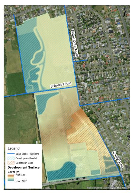
Figure 1: Modelled ground levels, base using LiDAR and development using design surface
