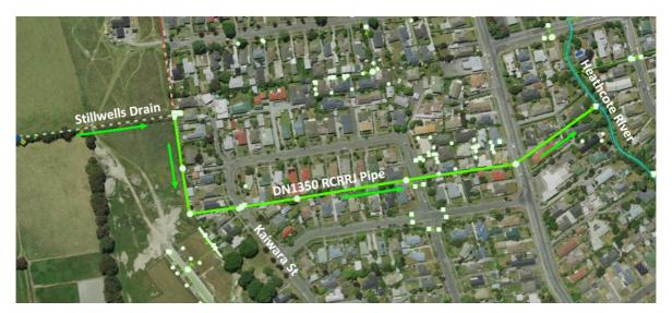
Figure 5. Stillwells Drain and DN1350 Concrete Pipe
