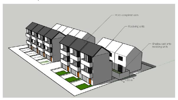
Figure 8: 3 storey MDRS development casting shadow on adjacent two storey model
