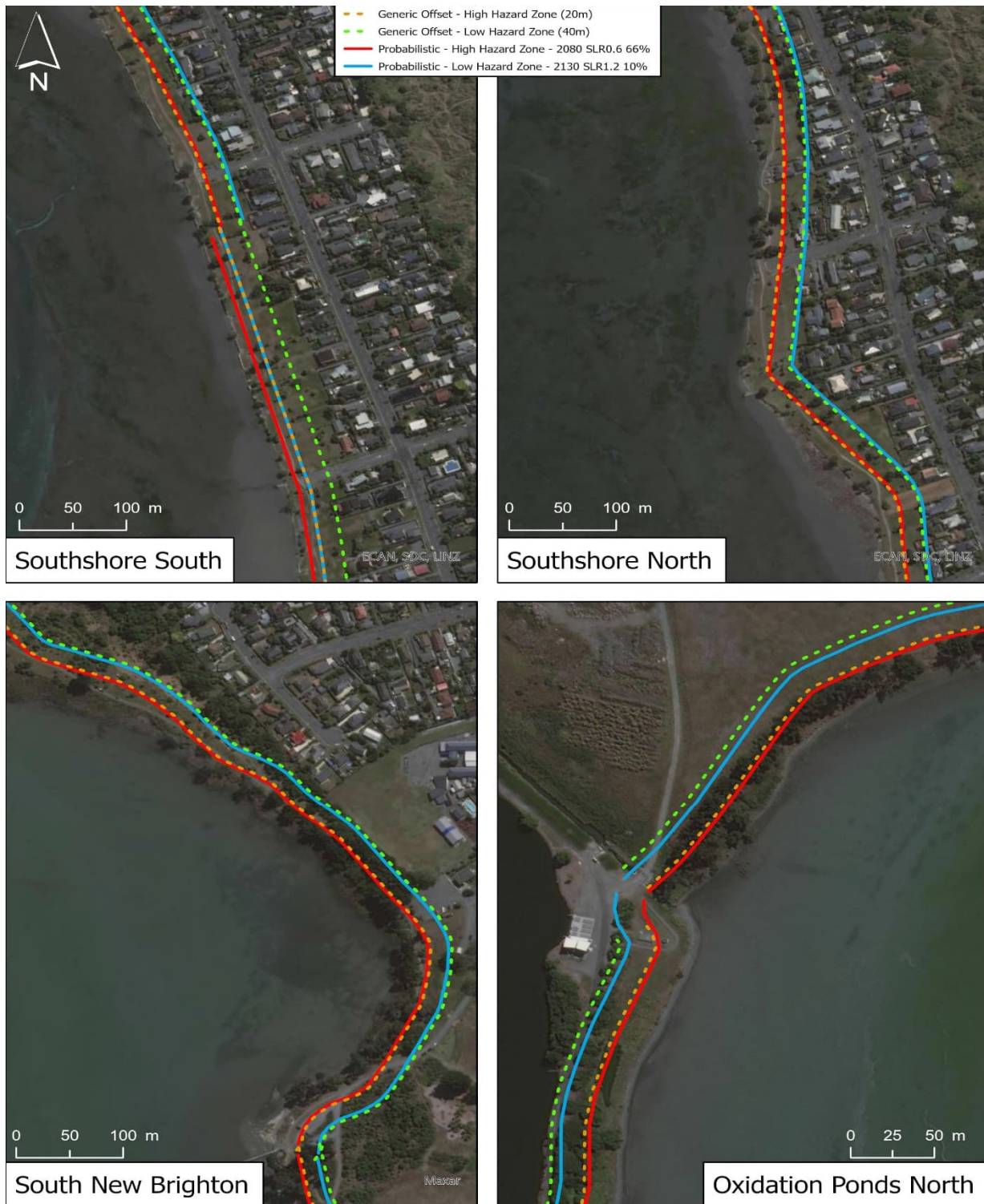
Figure 4-9. Recommended High-Medium and Low Coastal Erosion Hazard Categories at Southshore (left) and Oxidation ponds (right) around the Avon-Heathcote Estuary.
