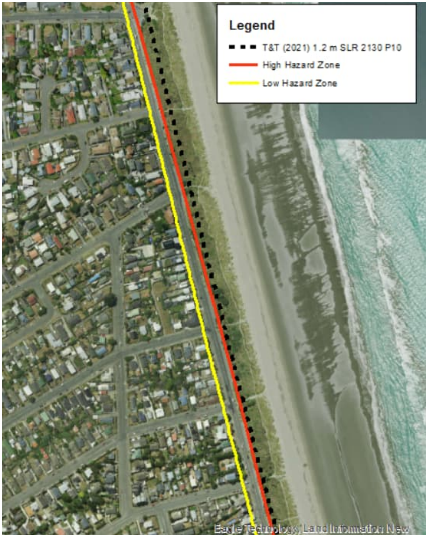
Figure 4-7. High and low hazard zones in North New Brighton/Waimairi Beach relative to the 1.2 m SLR 2130 erosion projection lines from T&T (2021).
