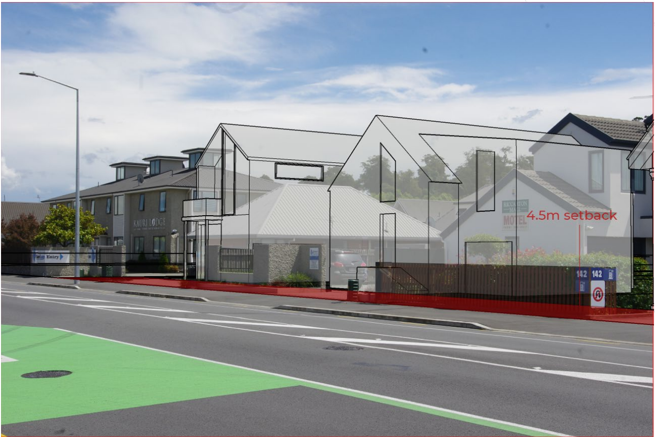
Figure 27: View along Riccarton Road looking northwest towards Pūtarīngamotu Riccarton Bush, with graphic overlay showing possible apartment configuration and height limit (8m) under the existing CDP .
