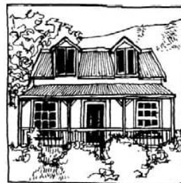
Verandah and simple gable with roof domers
