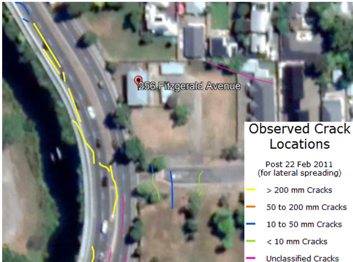
Figure 4-1 Ground cracks as recorded for EQC (from NZGD)
