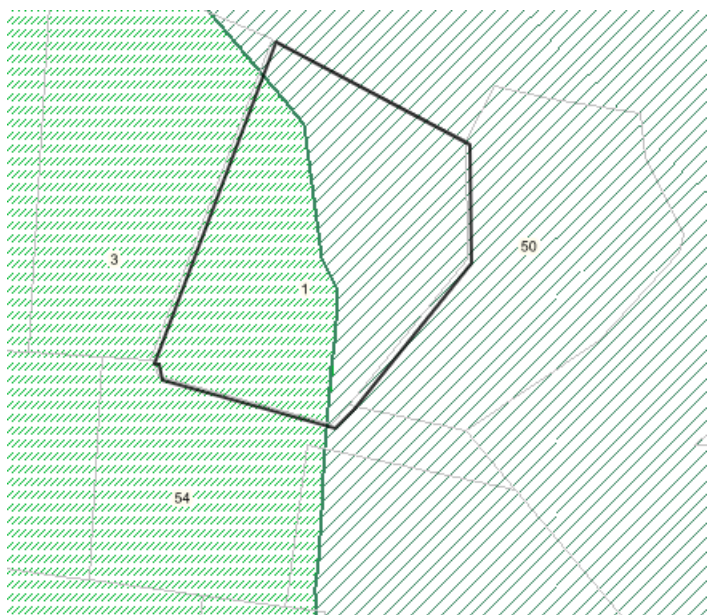
Figure 5: A zoomed view of the Natural Hazards Overlay, showing the boundary for the respective sites, noting that the cracking of the Villa on [REDACTED] followed the boundary between the two Areas.
