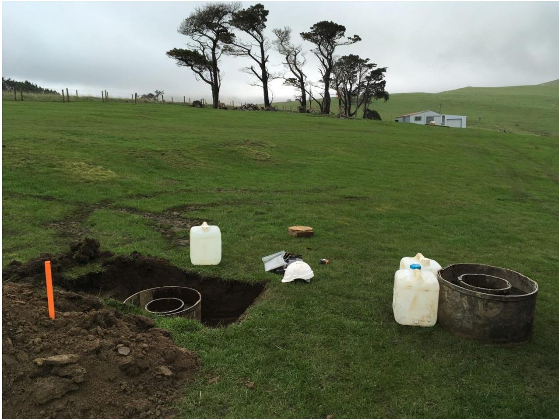
Photograph 13: Infiltration Test IT10 surface and sub-surface tests within Pompeys Pillar (Site 10).
