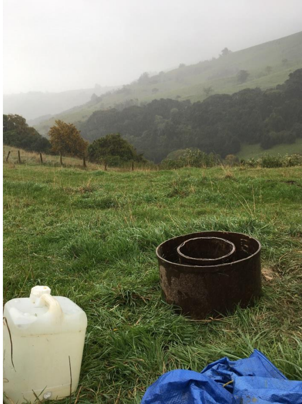
Photograph 7: Infiltration Test IT5 surface within Robinsons Bay (Site 5).
