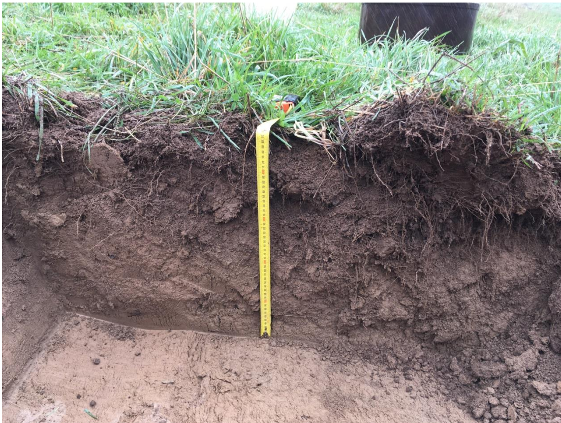
Photograph 8: Infiltration Test IT5 sub-surface pit within Robinsons Bay (Site 5).
