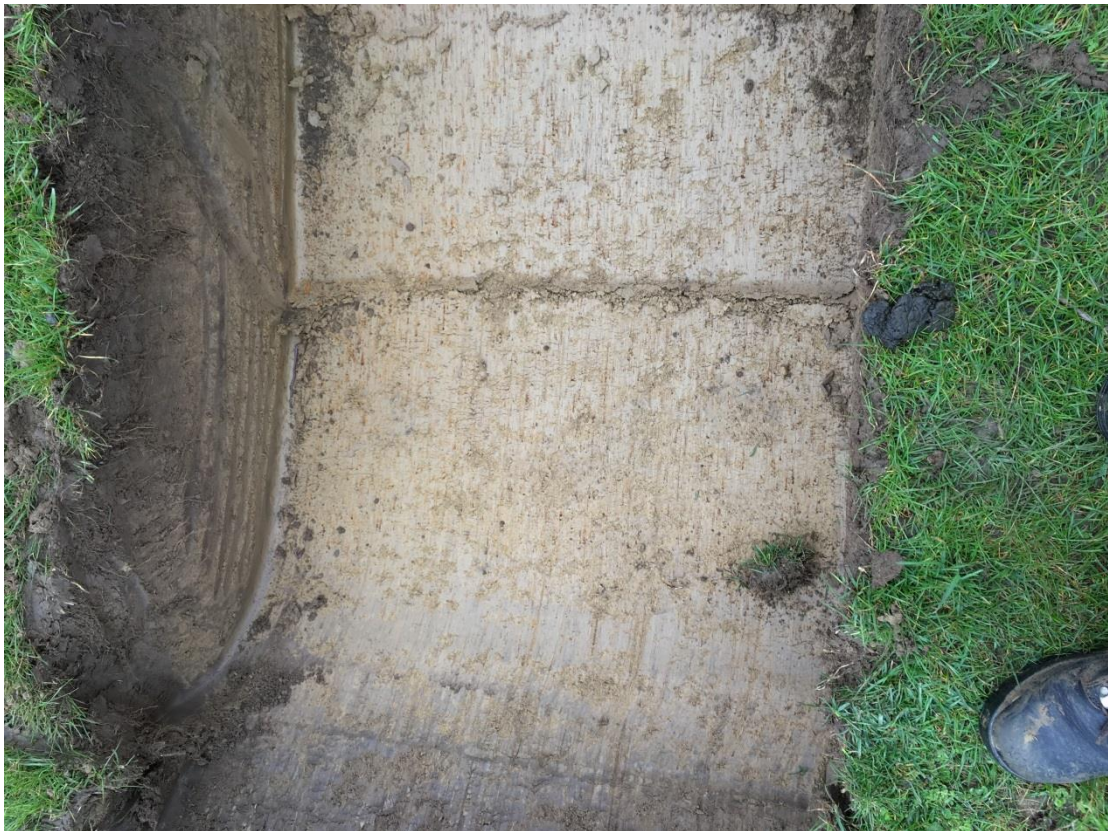
Photograph 12: Infiltration Test IT9 sub-surface test pit within Pompeys Pillar (Site 9).
