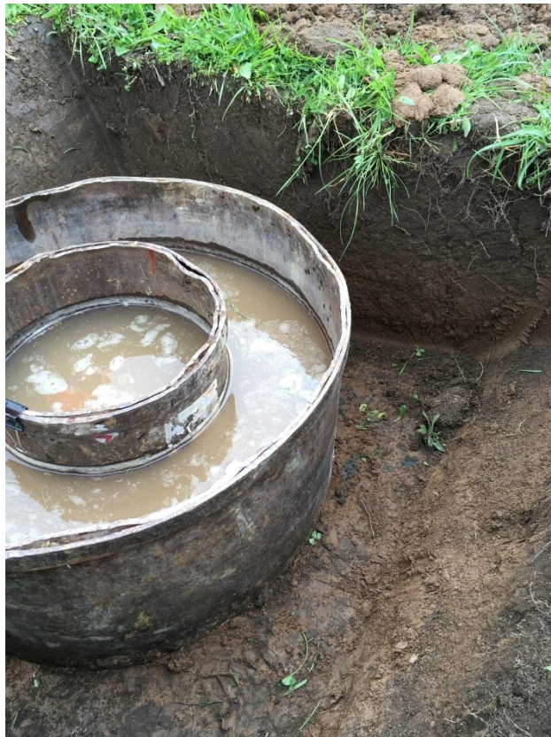
Photograph 2: Infiltration Test IT1 sub-surface infiltration test within Robinsons Bay (Site 1).
