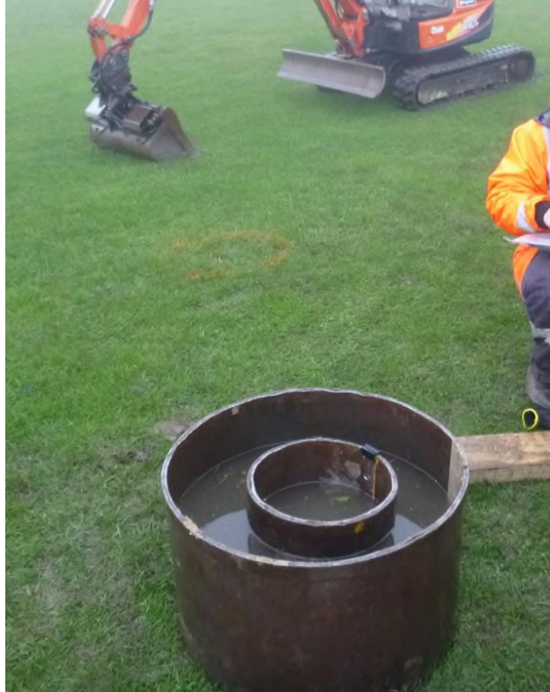
Photograph 9: Infiltration Test IT8 surface test within Pompeys Pillar (Site 8).
