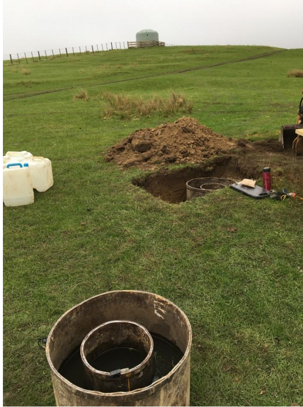
Photograph 11: Infiltration Test IT9 surface and sub-surface test within Pompeys Pillar (Site 9).
