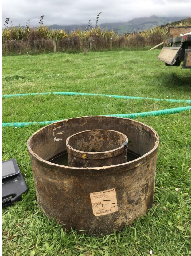
Photograph 1: Infiltration Test IT1 surface infiltration test within Robinsons Bay (Site 1).
