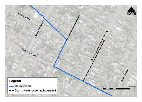
The work will include the removal and replacement of stormwater pipes along the road on Mackworth Street, and across some private property in the area.
