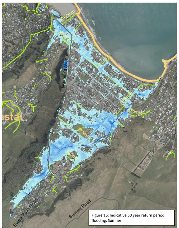
[Map: SurfaceWaterModels:\04\_ROG\Southshore MF D1 50yrCC1hr pt5SLR PostEQ ROG Depth]
