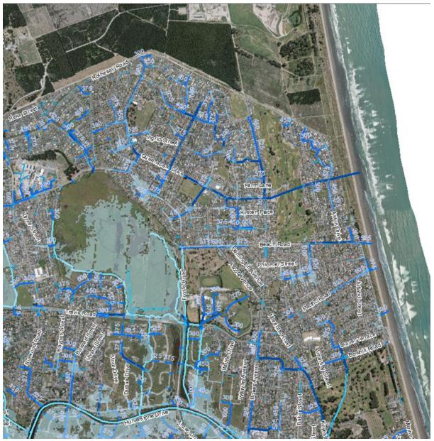
Figure 12: 50 year average recurrence interval flooding extent (pale blue) – from model results.
