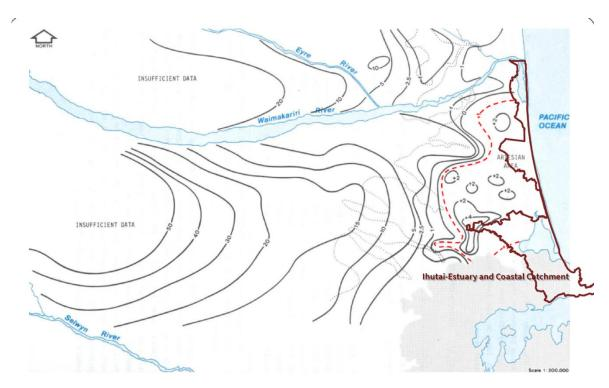
Figure 7: Piezometric surface contours: indicating positive aquifer pressure
