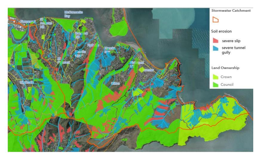
Figure 11: Areas on the Port Hills highly susceptible to erosion
