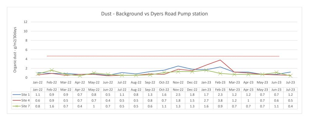
Offsite dust monitors 4 and 7 located along Dyers Road and downwind of the site. We can see the expected low levels of dust during the wetter winter months.
