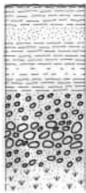
Underlayers: Clay & sand alternating on silt over greywacke river stones (2-100mm rounded) with some peat.
