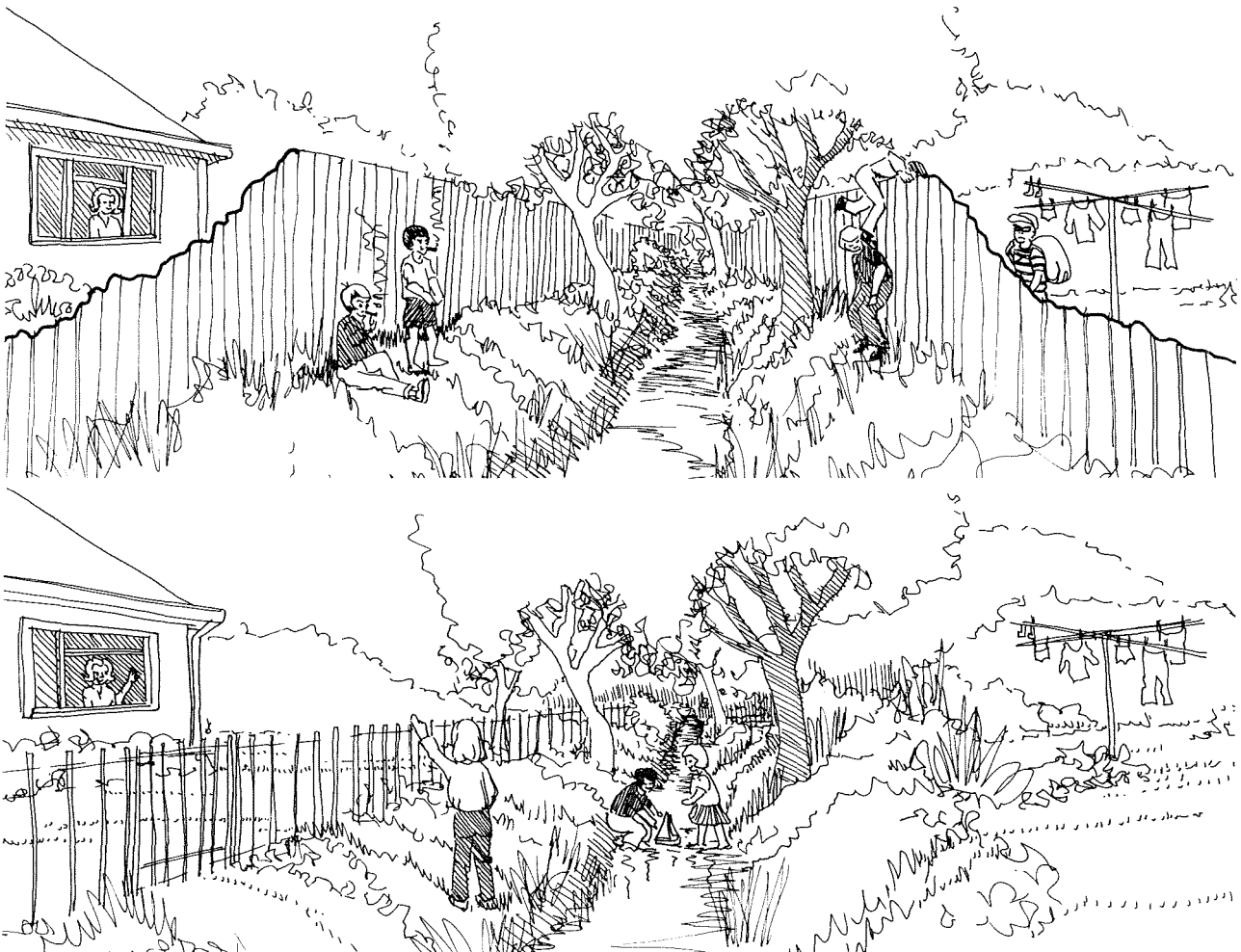
Figure 15-1: Solid fencing reduces visibility and can encourage unwanted behaviour (top). Where fencing is a necessity, the use of low, see-through open fences between waterways and private property create a safer environment, with greater visibility and communication (above). Increased communication can also help foster a sense of neighbourhood.
