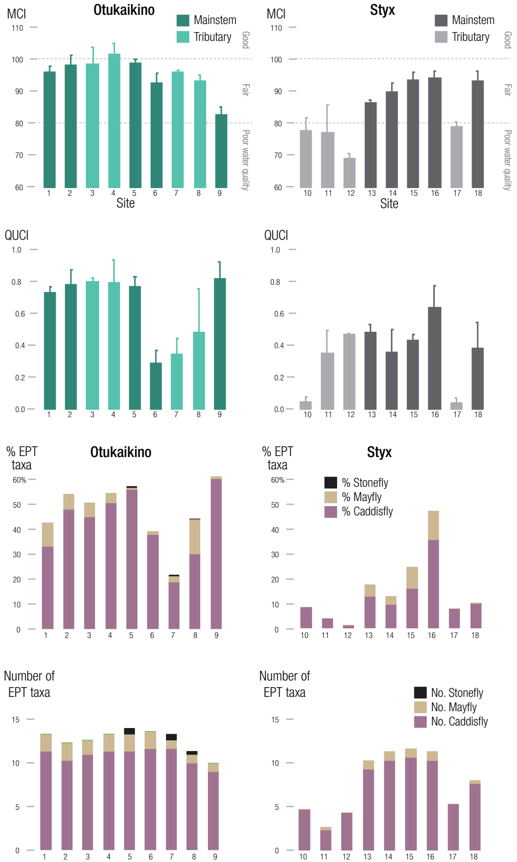
Figure 7 Biotic indices of invertebrate community health at nine sites within each of the Otukaikino and Styx catchments, sampled between the 12th and 27th March 2008. Sites 1 and 10 are the most downstream sites in the Otukaikino and Styx catchments, respectively. The dotted lines on the QMCI and MCI graphs indicate the probable level of organic pollution (Stark, 1985; Stark, 1998). Good water quality conditions (with only possible mild organic pollution) are indicated by MCI and QMCI values from 100–120 and 5–6, respectively. Poor water quality conditions (probable severe organic pollution) are indicated less than 80 for the MCI and less than 4 for the QMCI.
