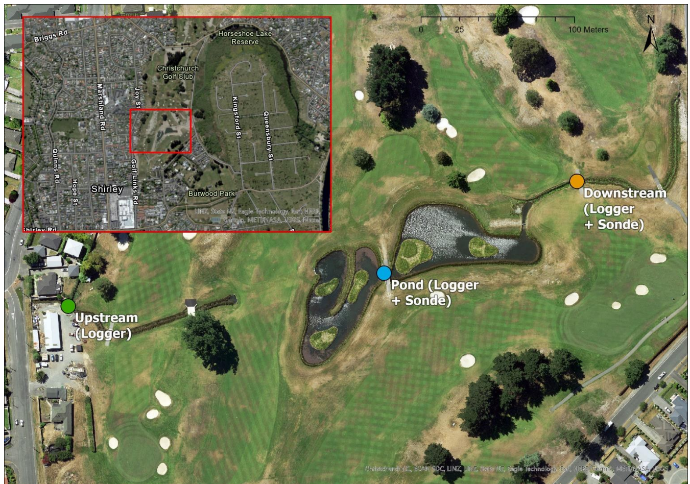
Figure 2. No.1 Wetpond and sensor locations
