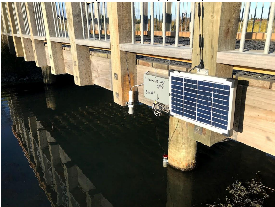
Figure 1. Custom logger system deployed in the pond location.
