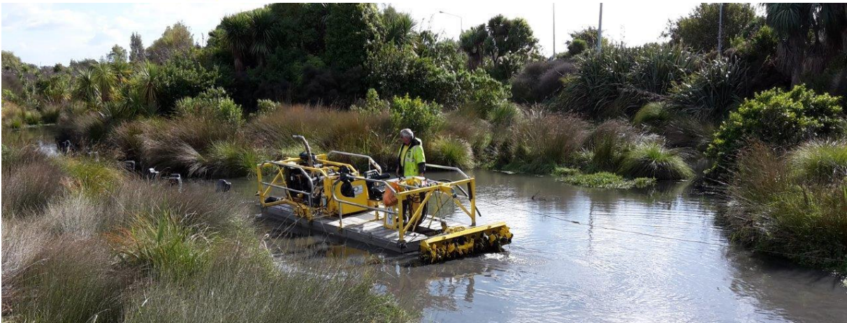
Figure 5-3: Dino-6 vacuum dredge. Images from https://geoforinternational.com/products/dino6/ and CCC.
