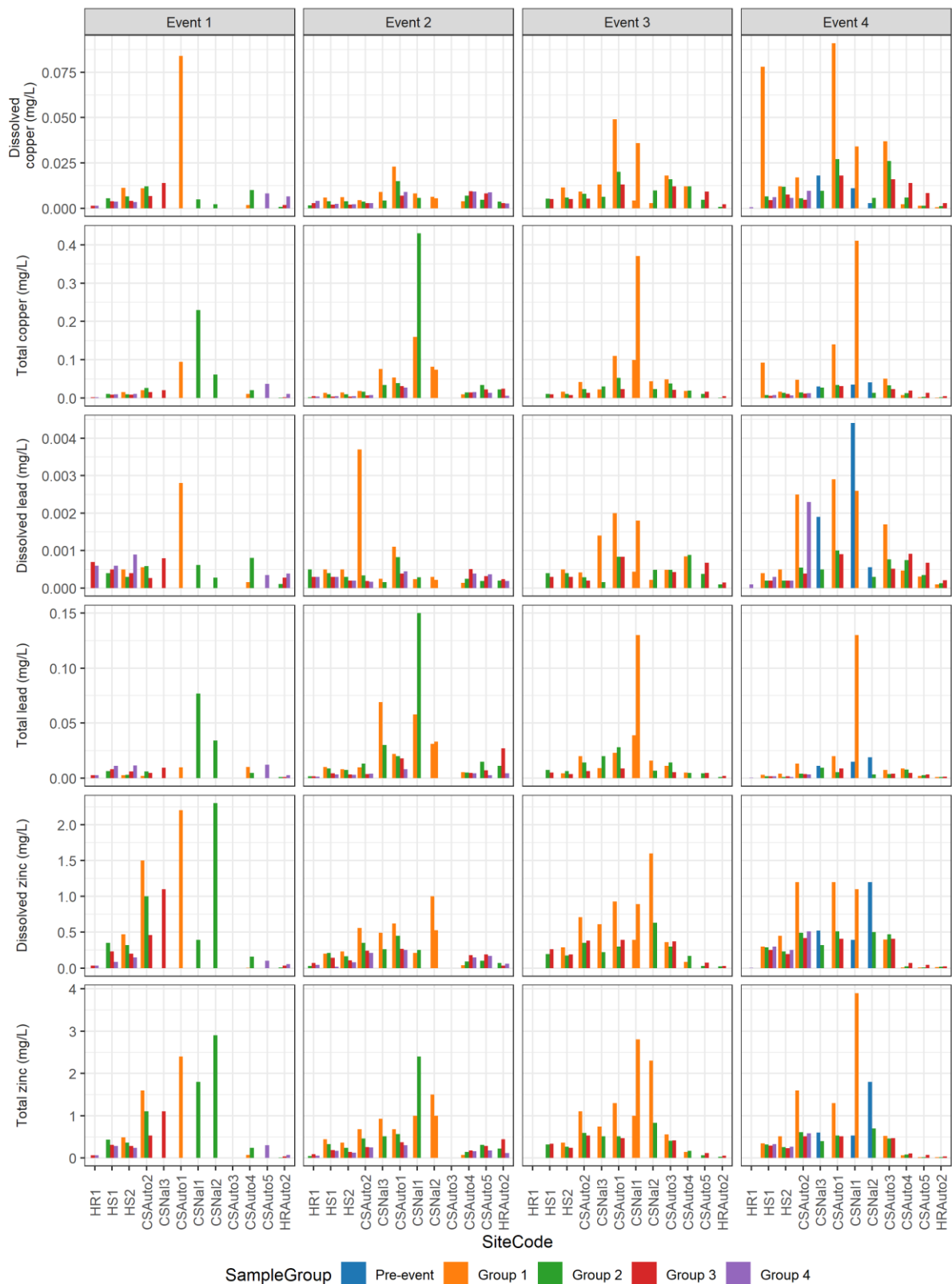
Figure 3-8: Copper, lead and zinc concentrations for each site, each event and sample group. Colour of bar represents the sample group (i.e., the composite group made of multiple samples collected by the autosampler). Reduction in height of bar from group 1 to 4 represents a declining concentration, i.e., a first-flush effect.
