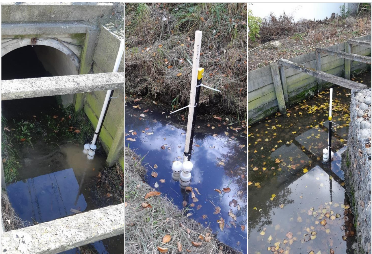
Figure 2-2: Waratah with two Nalgene sampling bottles installed at the three sampling sites. From left to right: CSNa1, CSNa2 and CSNa3.
