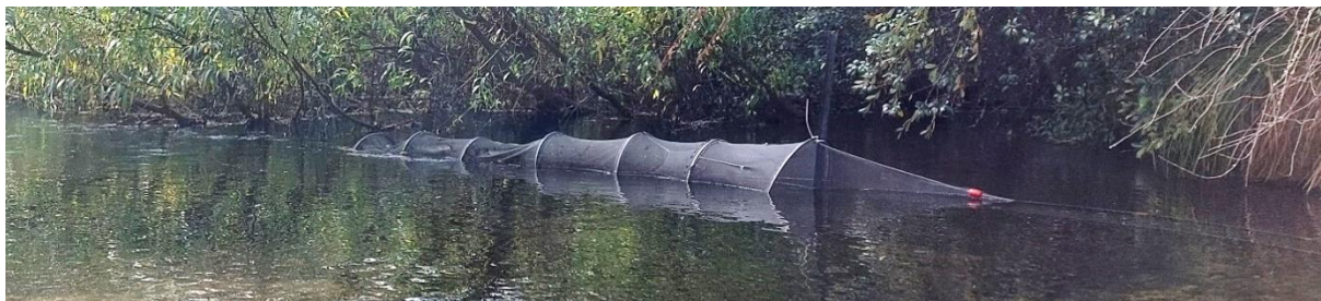
Figure 2: Hīnaki/fyke net in situ at OTU04. The leader was staked upstream in low flow conditions and downstream in high flow conditions.
