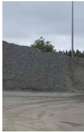
Hardfill that has been dug up and stockpiled for reuse © Copyright
