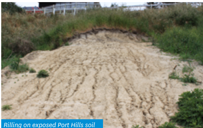
Rilling on exposed Port Hills soil
