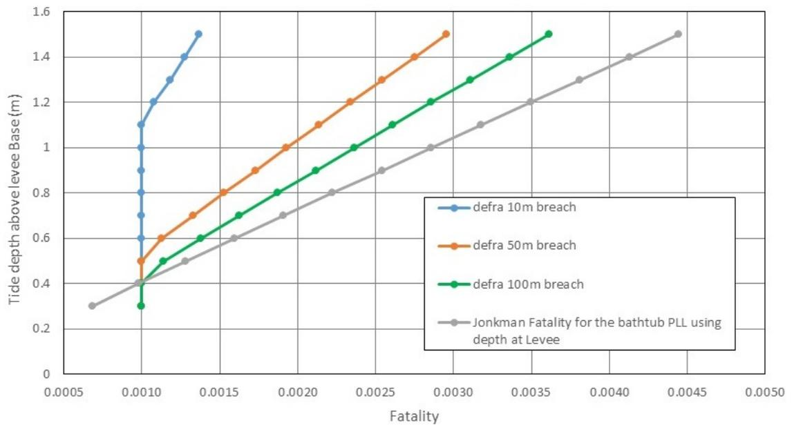
**Figure 3-4 Tide depth above stopbank base versus fatality using “defra” Figure 2-7 and Jonkman “Bathtub”**
