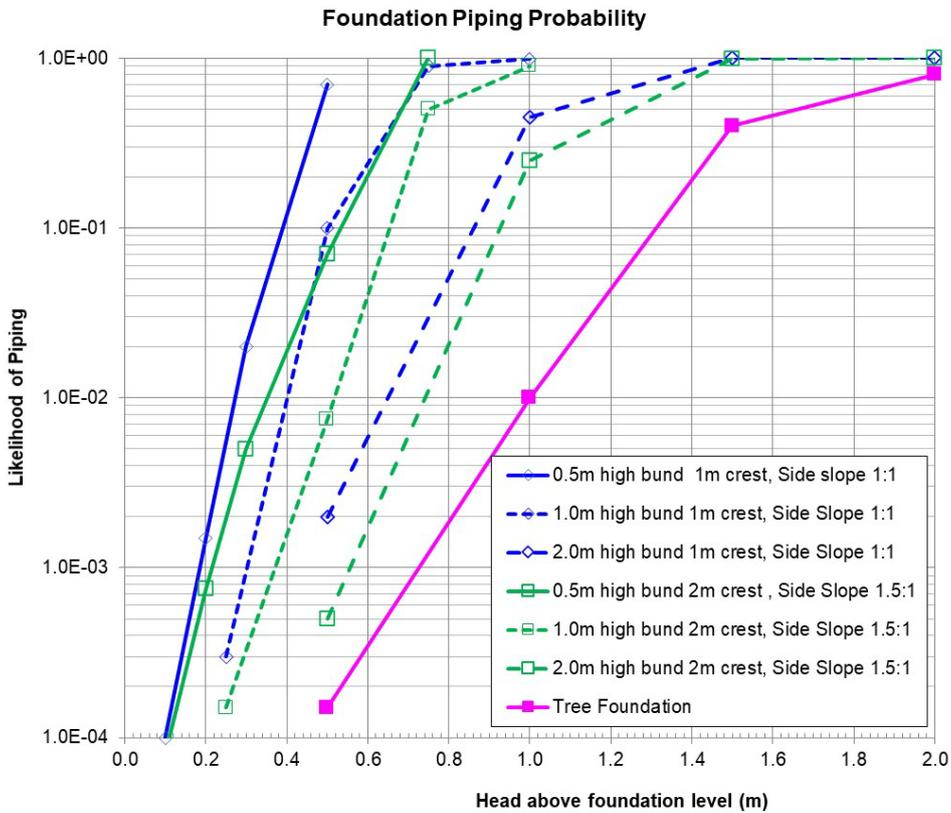
**Figure 4-3 Estimated probability of foundation piping versus head above foundation level for various stopbank configurations**
