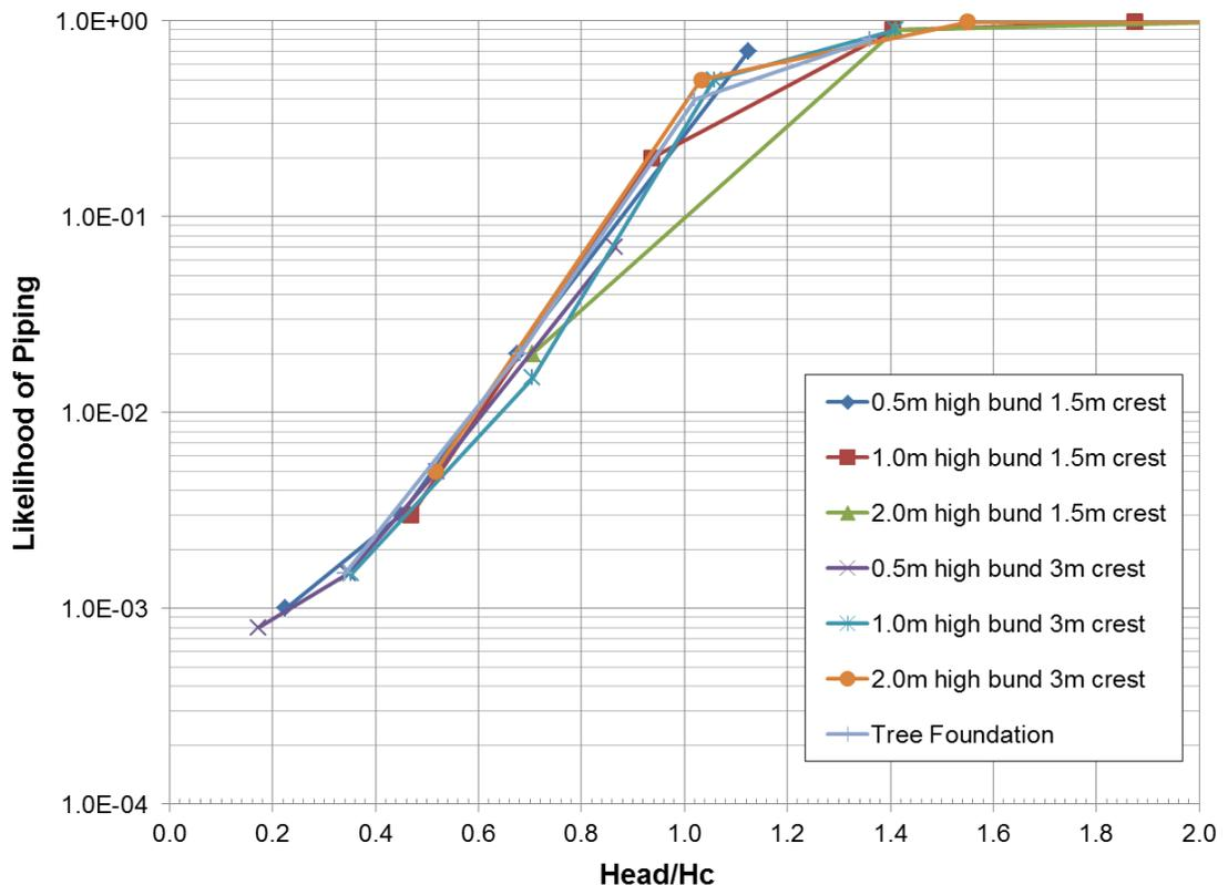
**Figure 1-12 Estimated probability of foundation piping initiation for several bund geometries**
