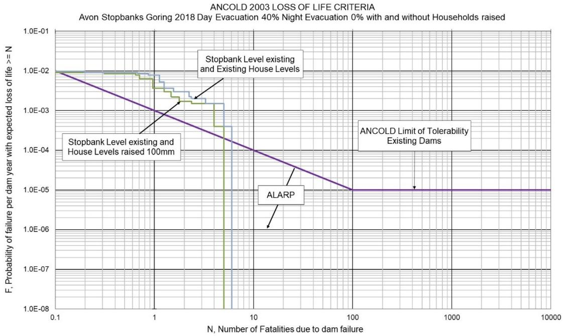
**Figure 6-3 Avon Stopbanks comparison of societal risk with floor levels raised by 100 mm compared with the original analyses (Section 1 level at 11.4 m and others 11.2 m)**
