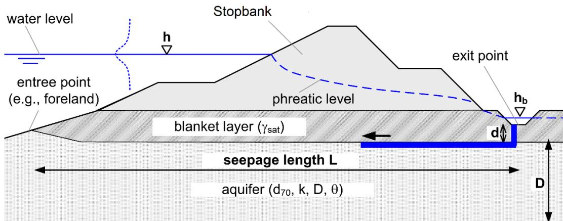
**Figure 1-11 Geometry of backward erosion piping model**
