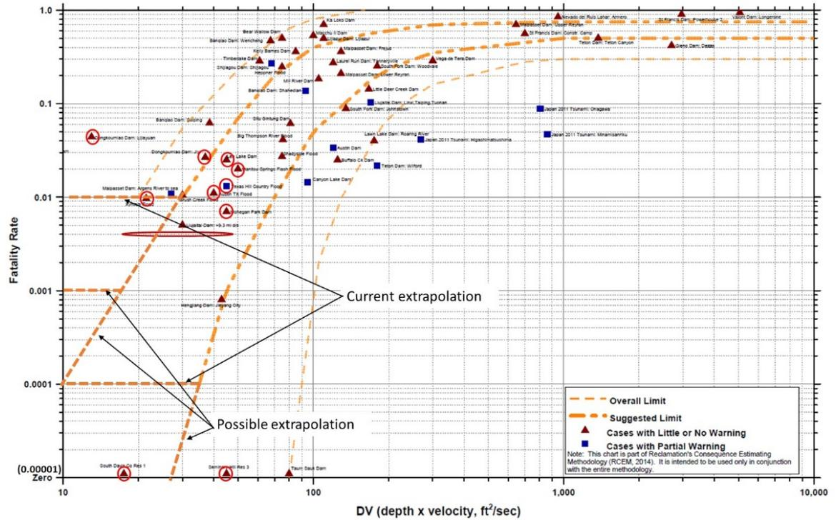
**Figure 2-5 RCEM Figure 1 - Fatality rate vs DV for cases with little or no warning and partial warning (Showing existing and potential extrapolations to the original lines)**
