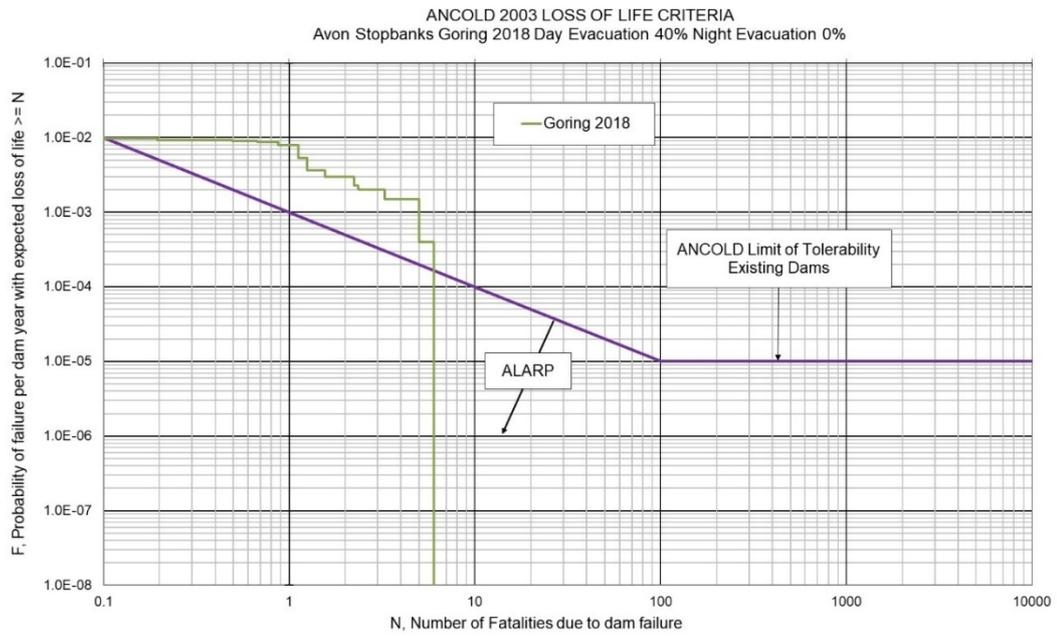
**Figure 5-2 Avon Stopbanks societal risk – current stopbank levels (generally 11.2 m, Section 1 at 11.4 m)**
