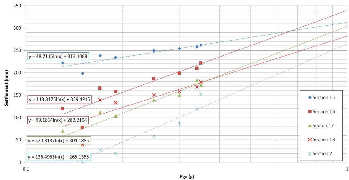
**Figure 1-3 Avon Stopbanks typical deformation analysis results**
