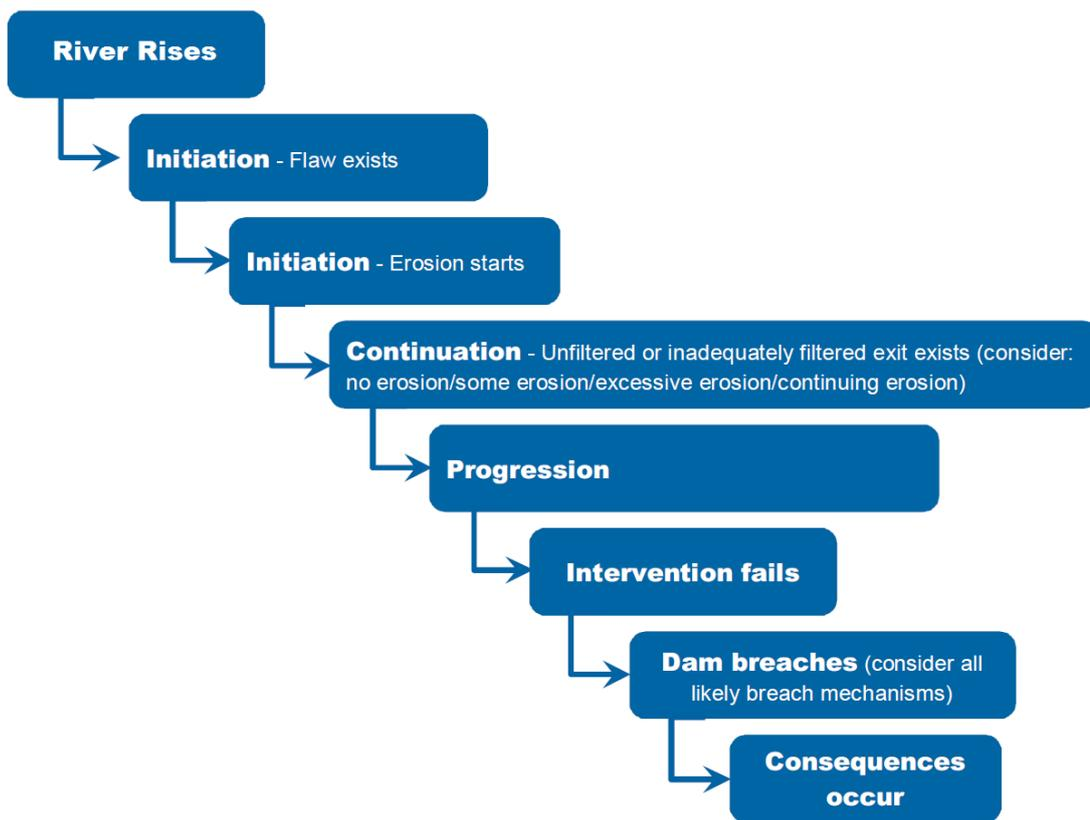
**Figure 1-5 Generic Sequence of Events for Piping Failure Modes Analyses**
