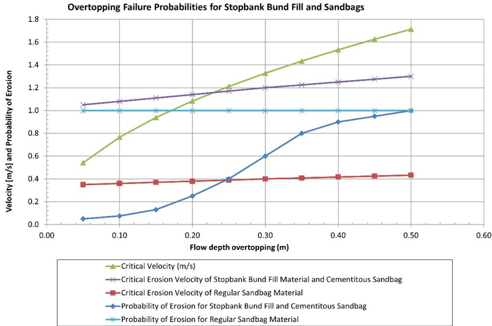
**Figure 1-15 Estimated Probability of Overtopping Failure for Range of Overtopping Flow Depths**
