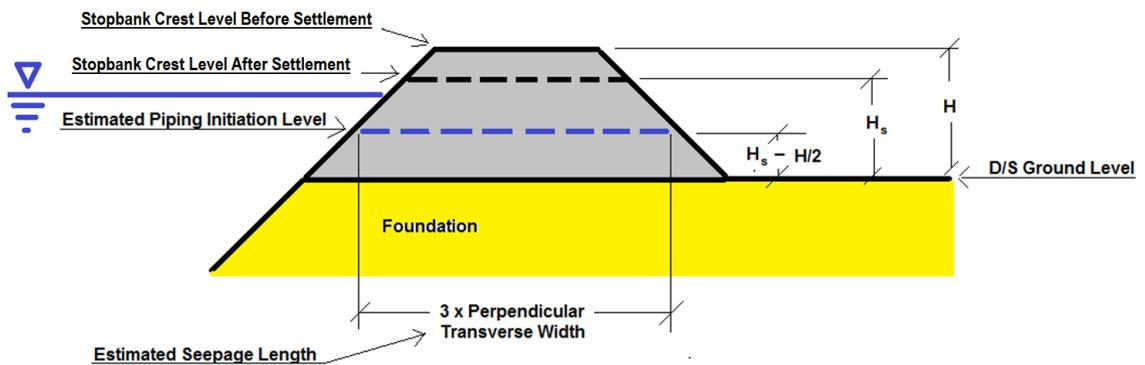
**Figure 1-10 Schematic section showing the estimation of Hydraulic Gradient Initiating Piping**
