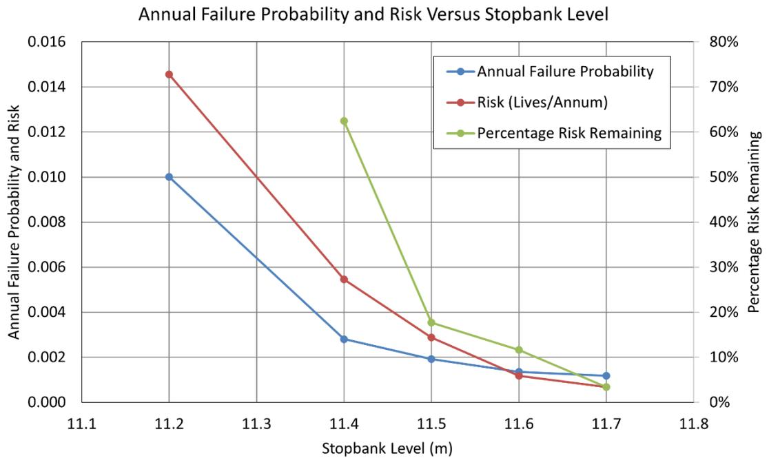
**Figure 6-4 Avon Stopbanks comparison of societal risk with floor levels raised by 100 mm compared with the original analyses (all levels at 11.5 m)**
