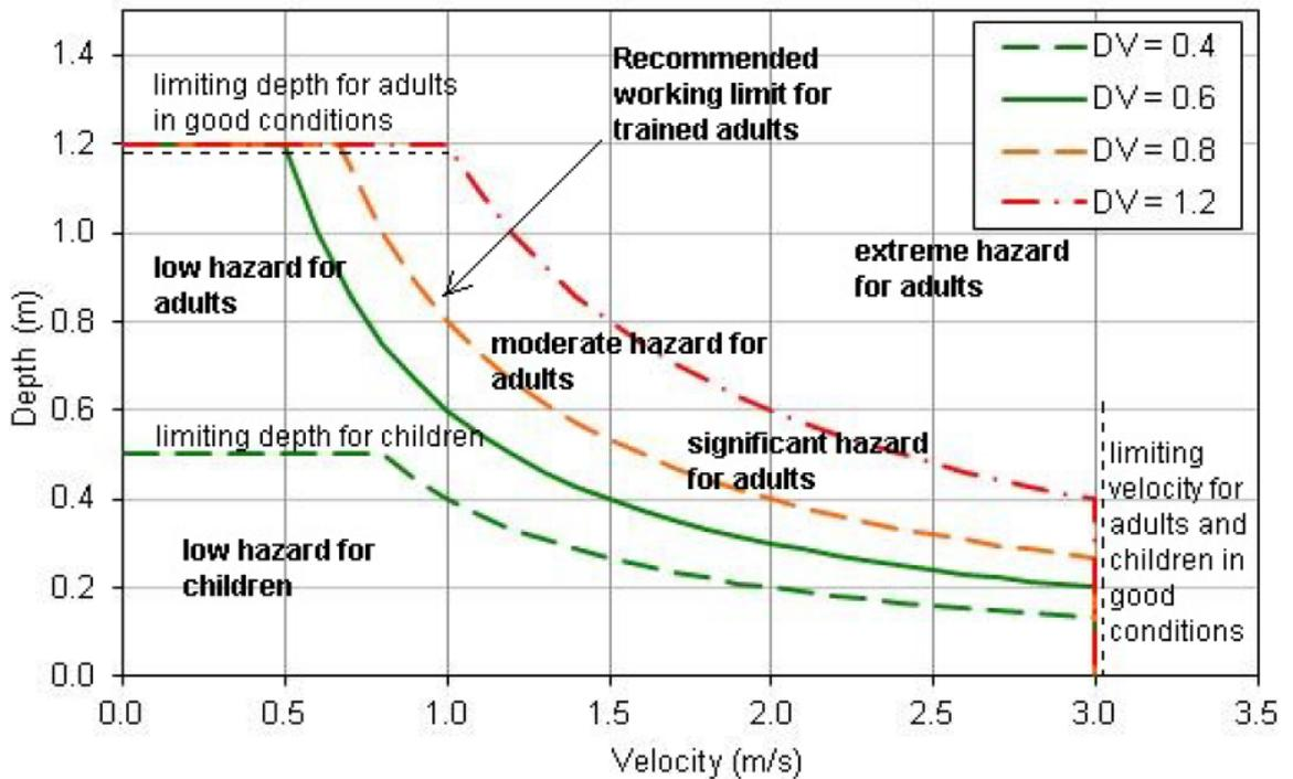
**Figure 2-3 Safety criteria for people in variable flow conditions (after Cox et al, 2010)**
