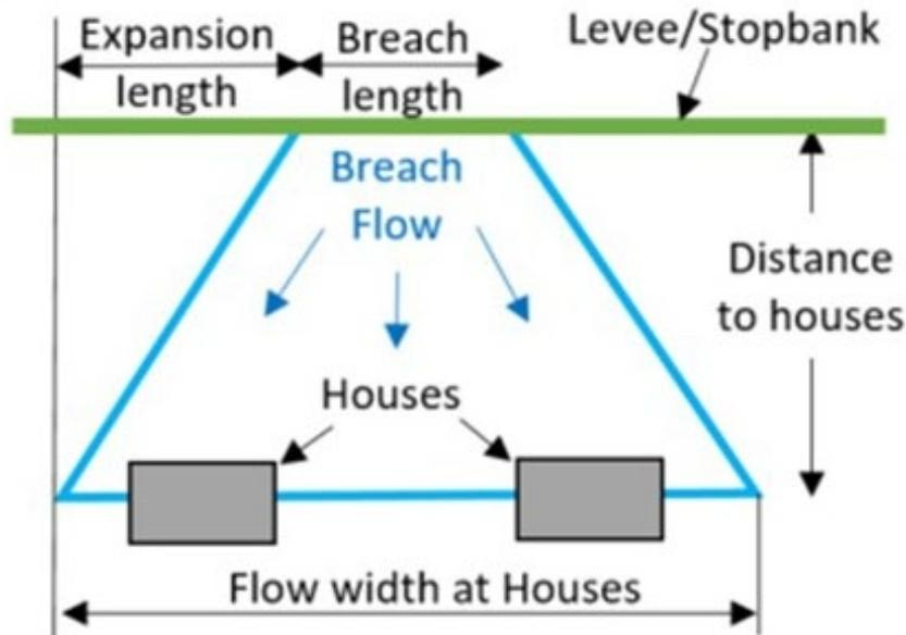
**Figure 4-8 Schematic of the breach expansion from the stopbank to the closest houses**
