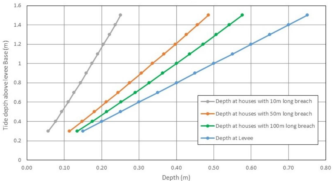
**Figure 3-3 Tide depth above stopbank base versus depth at the stopbank and 25m from the stopbank with various breach lengths**
