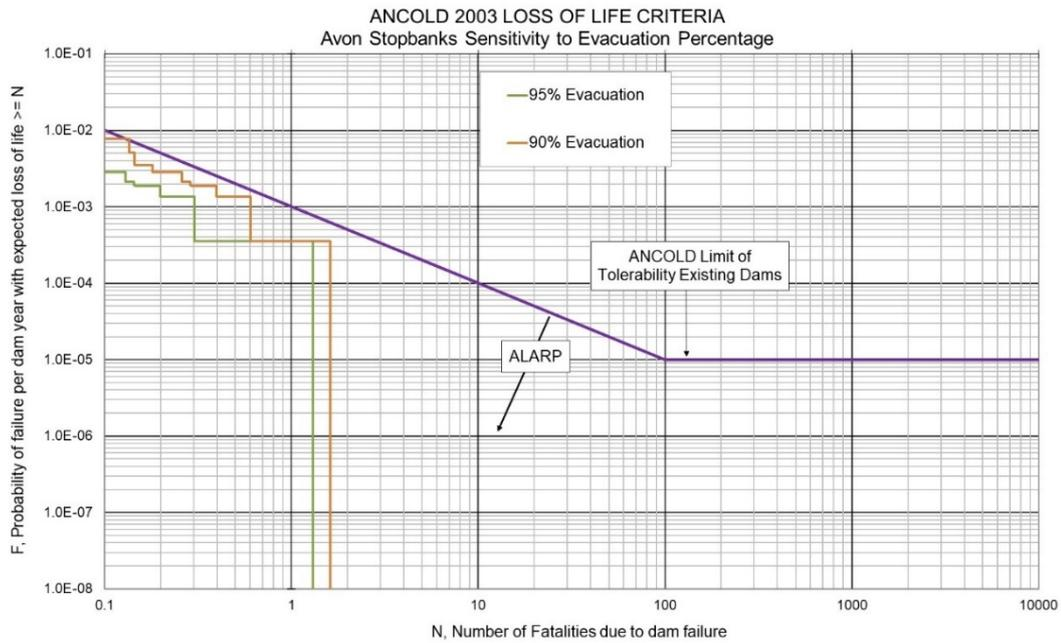
**Figure 7-6 Avon Stopbanks societal risk section 1 level at 11.4 m and others 11.2m with 90% and 95% evacuation of PAR**
