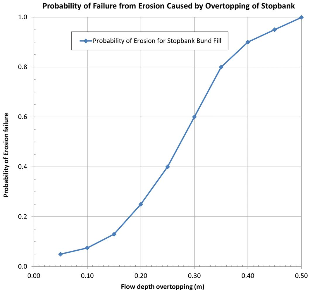
**Figure 4-1 Stopbank failure probabilities versus overtopping depth**
