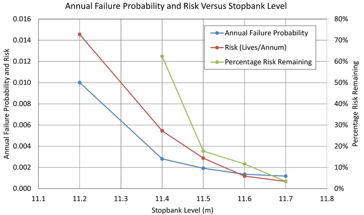
**Figure 7-4 Avon Stopbanks annual failure probability and risk versus stopbank level**
