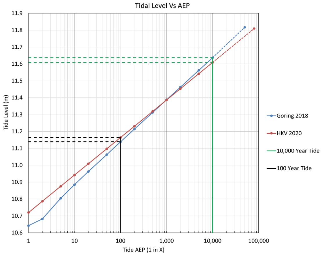
**Figure 3-2 Avon Stopbank tidal level versus AEP**
