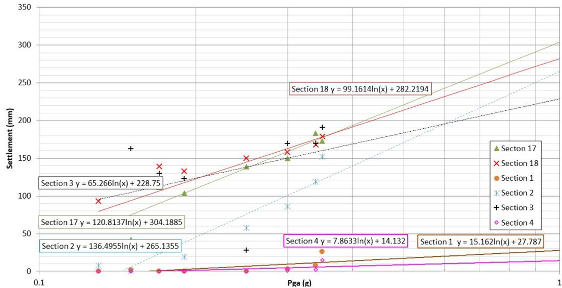
**Figure 4-4 Stopbank settlement versus peak ground acceleration**
