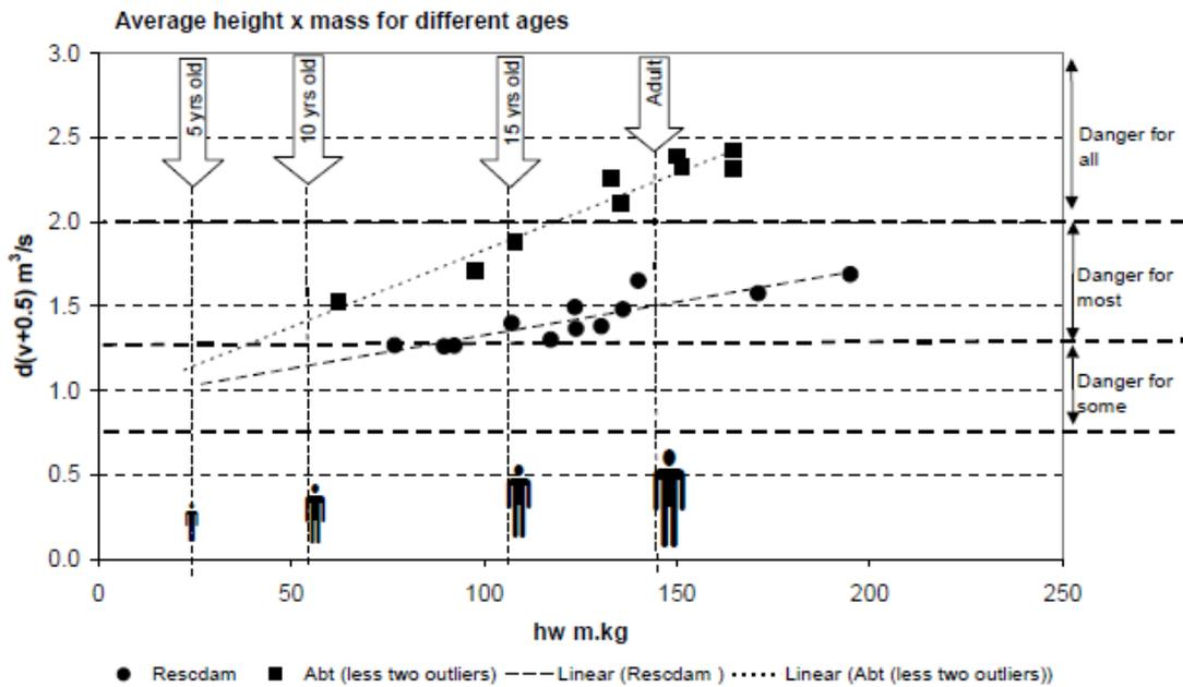
**Figure 2-8 The interpretation of the data sets to derive flood hazard thresholds (from DEFRA Supplementary 2008)**
