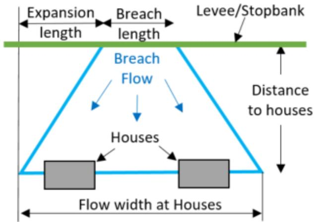
**Figure 3-1 Schematic of the breach expansion from the stopbank to the closest houses**
