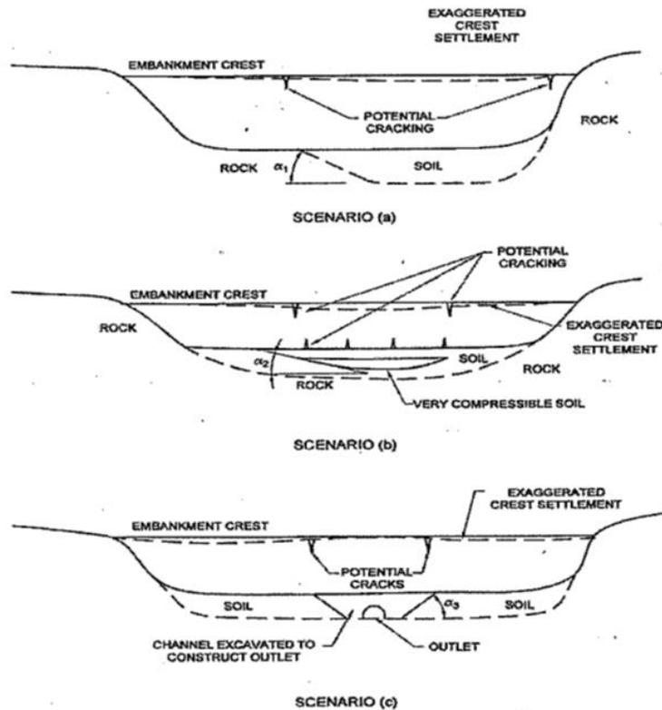
**Figure 1-8 Typical scenarios which may lead to differential settlement in foundations**
