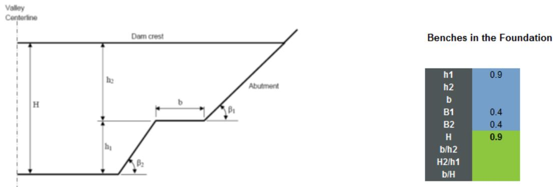
Figure 1-6 Piping Toolbox Figure 5.1 for benching
