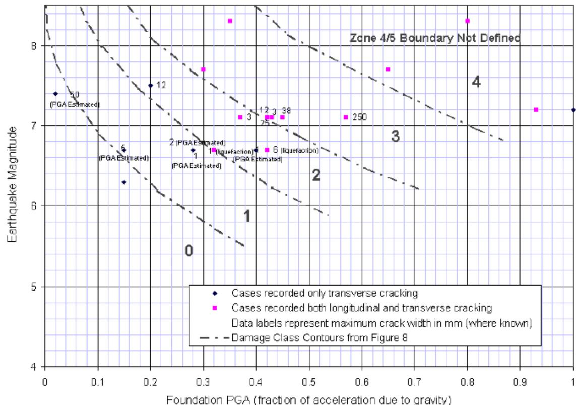
**Figure 1-9 Incidence of transverse cracking versus seismic intensity and damage class contours for earthfill dams (Piping Toolbox Fig 5.8)**
