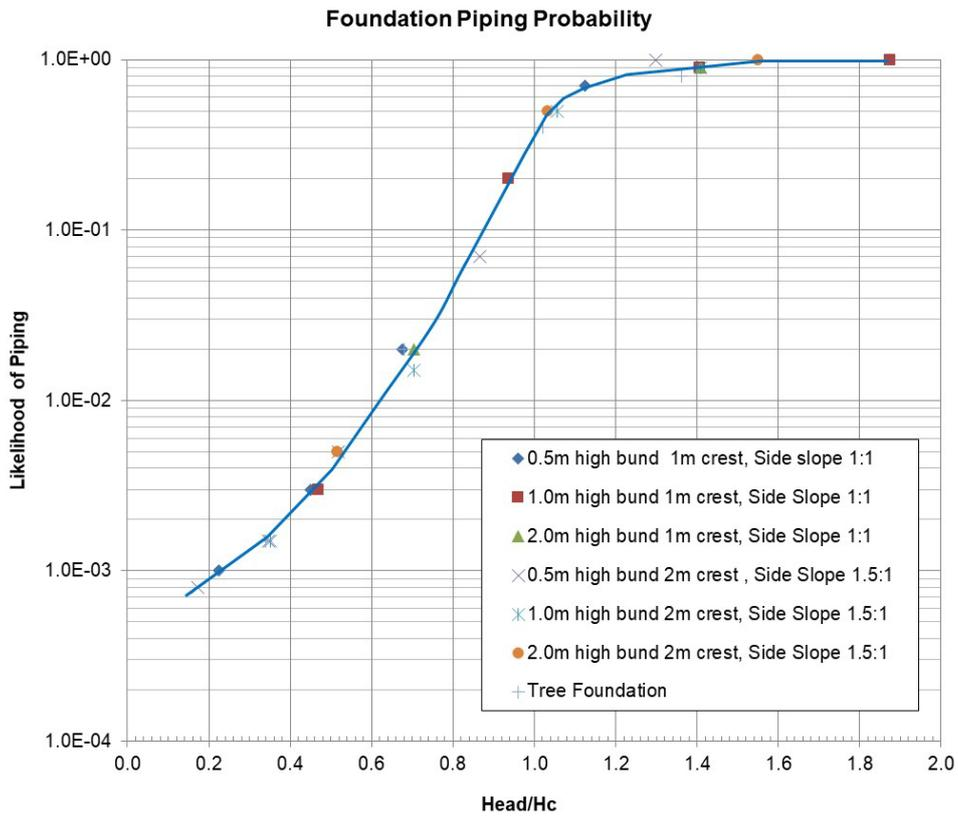
**Figure 4-2 Estimated Probability of Foundation Piping versus ratio of head above foundation level to critical head**
