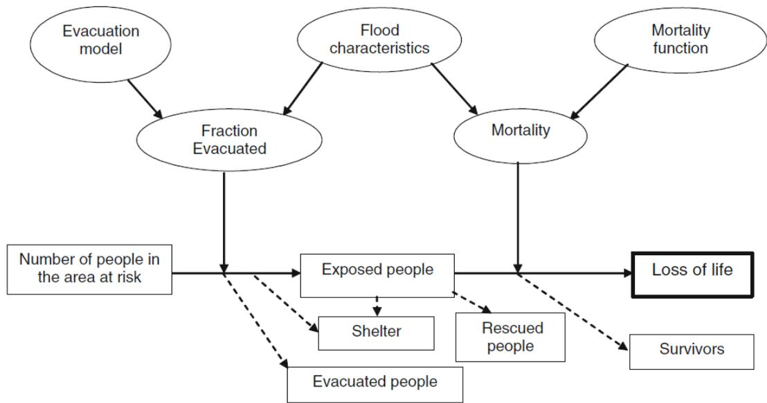
**Figure 2-9 General approach for the estimation of loss of life due to flooding**
