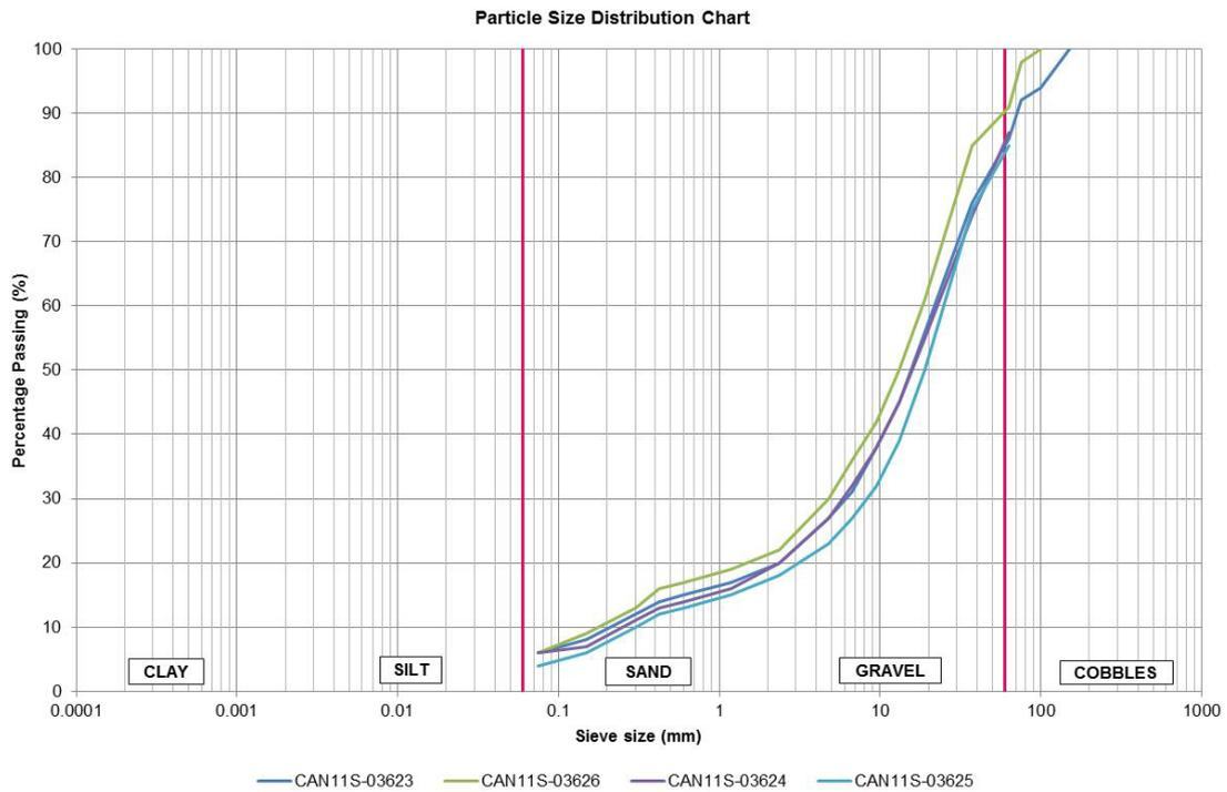
**Figure 1-2 Avon Stopbank material gradings**
