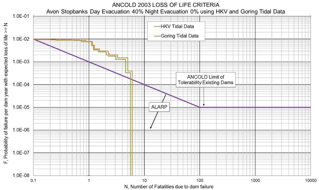
**Figure 6-2 Avon Stopbanks comparison of societal risk using Goring and HKV tidal data with current stopbank levels (general levels at 11.2 m and Section 1 level 11.4m)**
