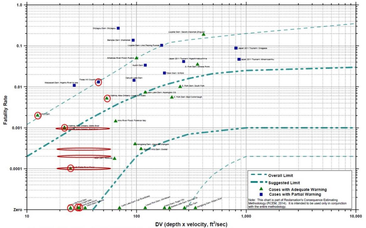
**Figure 2-6 RCEM Figure 2 - Fatality rate vs DV for cases with adequate warning and partial warning**
