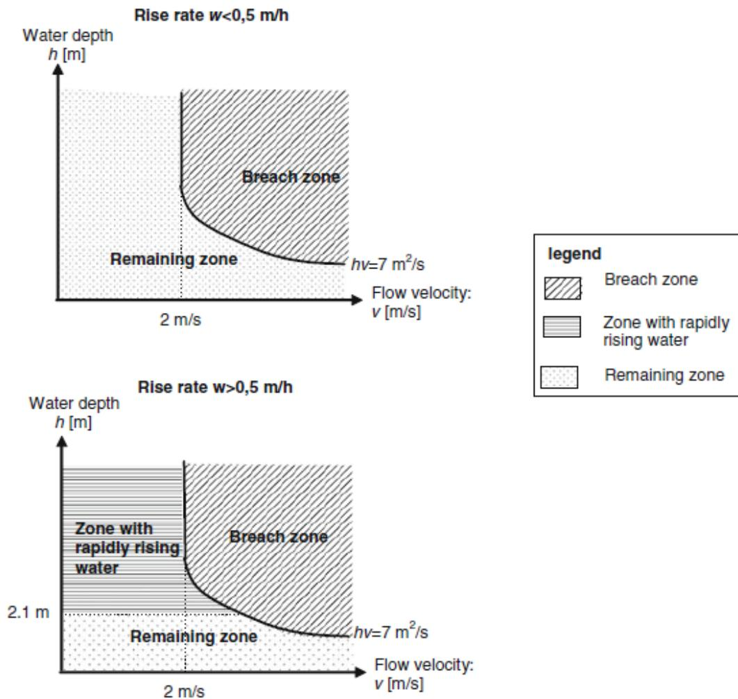
**Figure 2-11 Area of application of mortality functions, as a function water depth, rise rate and flow velocity (Jonkman Sep2008 Figure 16)**
