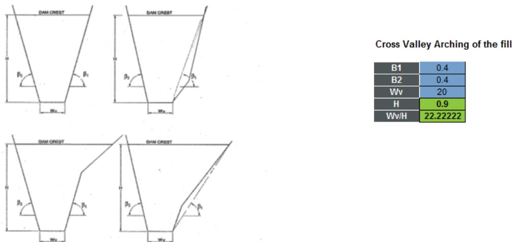
Figure 5.3 – Longitudinal profiles of the dam showing the definition of terms for cross valley arching.
