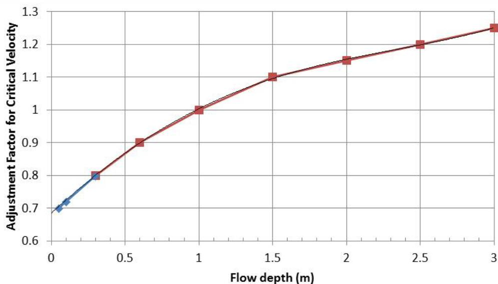
**Figure 1-14 Adjustment factor for critical velocity of flow**
