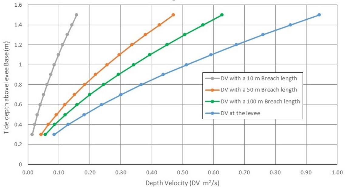
**Figure 3-2 Tide depth above stopbank base versus DV at the stopbank and 25m from the stopbank with various breach lengths**
