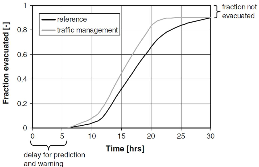
**Figure 2-10 Example of estimation of the time required for evacuation for the area**
