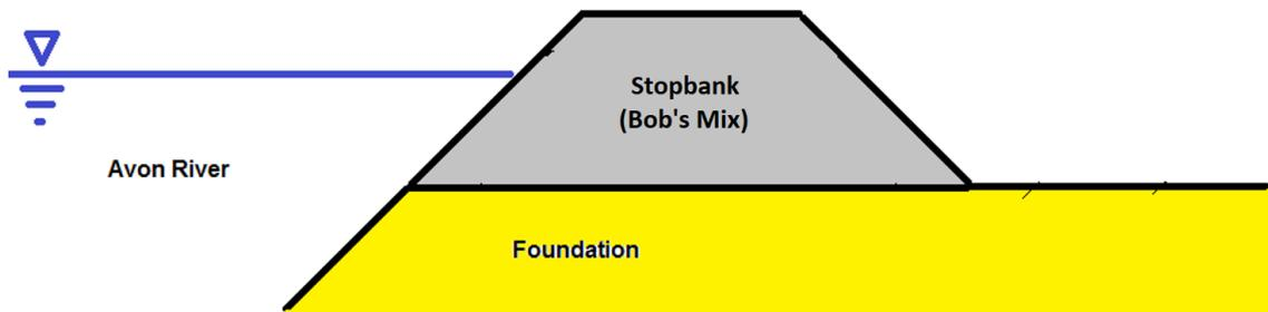
**Figure 1-1 Generalised Schematic Section of River – Stopbank Interface**
