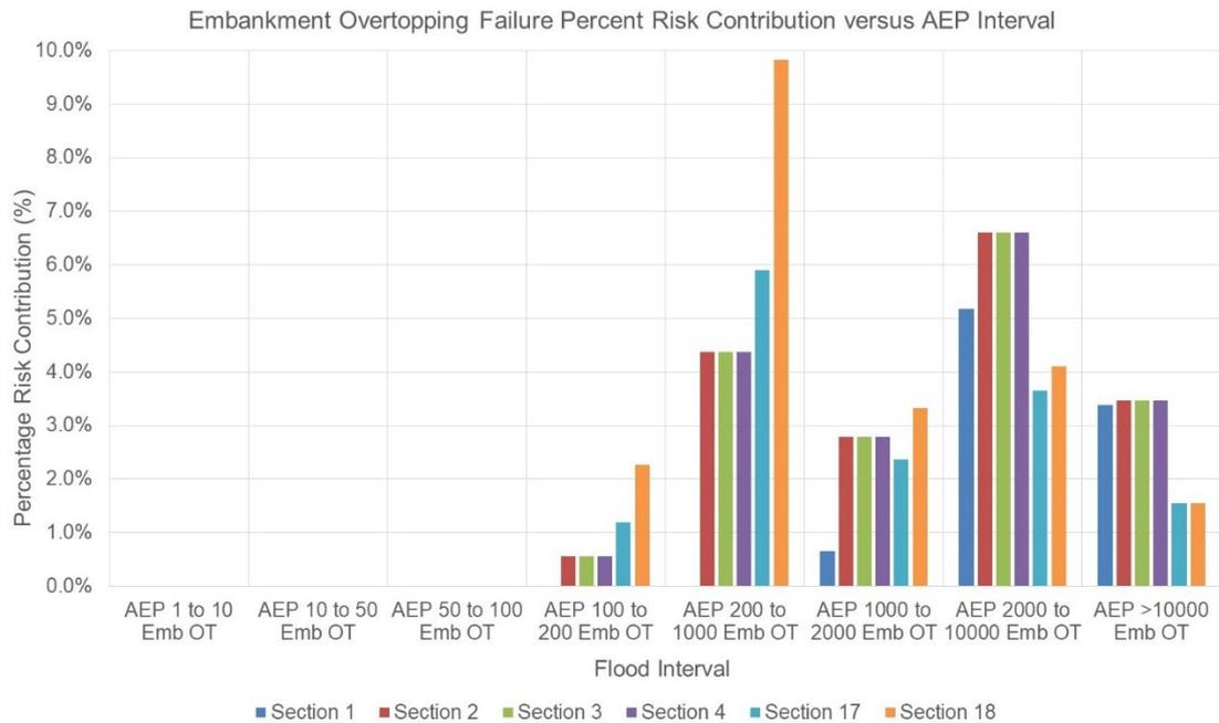
**Figure 4-9 Embankment overtopping failure mode – risk contribution versus AEP interval for each stopbank section**
