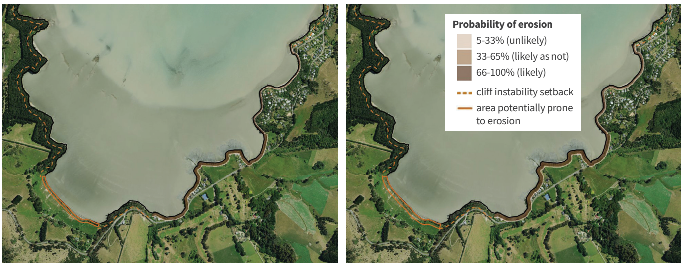
Coastal storm erosion distances sourced from Coastal Hazard Assessment 2021 (Tonkin & Taylor). The images show erosion distances with 40cm (left) and 1.5m (right) of sea level rise. The dashed orange lines represent the area of cliff prone to future instability. The solid orange line shows an area potentially prone to erosion. The brown areas are where a more detailed assessment has been undertaken and show the probability of short-term storm erosion.
