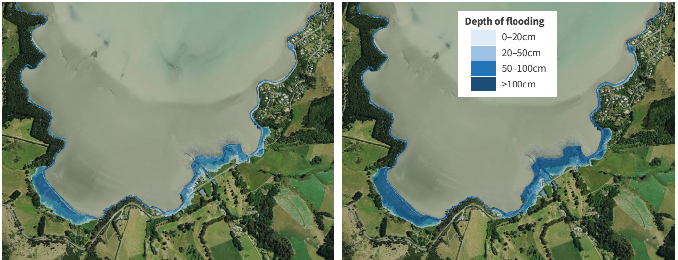
Coastal flooding extent and depths with 40cm (left) and 1m (right) of sea level rise during a rare (1 in 100 year) storm event – sourced from Coastal Hazard Assessment 2021 (Tonkin & Taylor).
