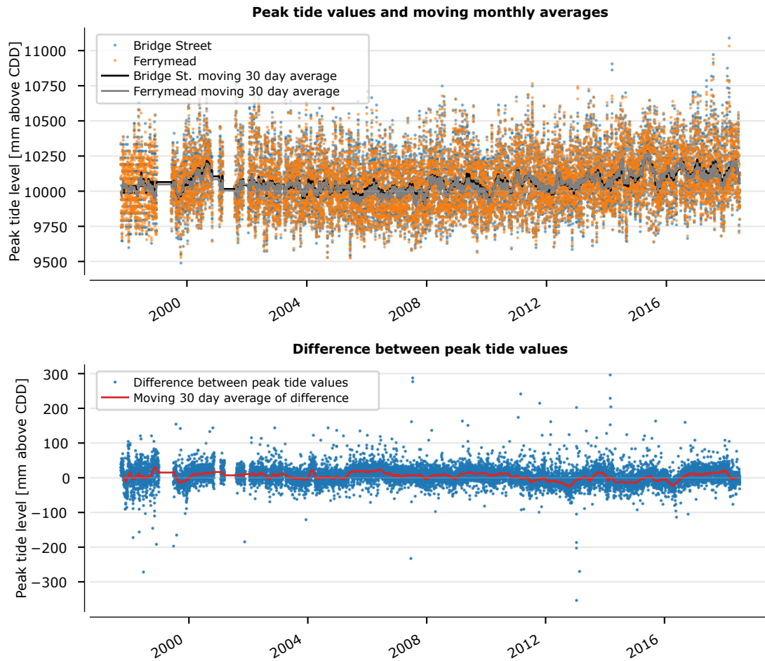
Figure C.5: Above: Moving average of high tide values with a monthly (30 day) moving window. Below: The difference between the high tide values with a moving average of this difference.
