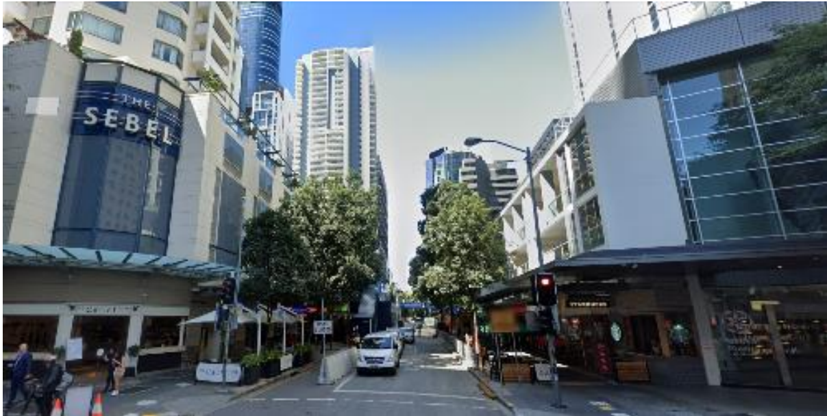
Figure 8: Charlotte Street, Brisbane, Australia. Street wall created by requiring a 3-storey podium with setbacks beyond this (source: Google Streetview).
