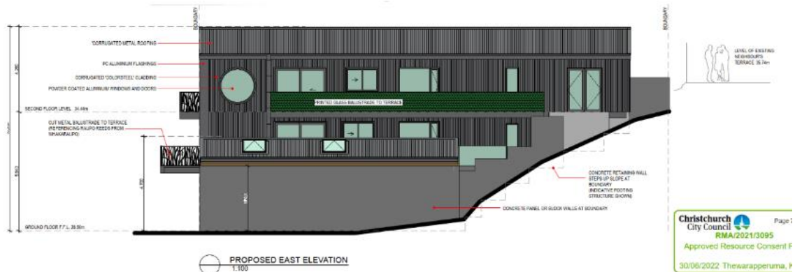
Figure 7: Side elevation (east elevation) RMA/2021/3095 illustrating the relationship of development to the north of London Street and the proposed Residential Heritage Area located above (right). The full height of the proposal is 10.6m from street level but both gable roofs and a 1.5 storey section provide for sunlight access from the north (hills) and sightlines from above to the south (harbour).
