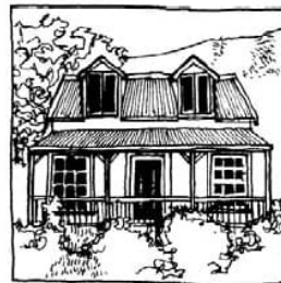
Verandah and simple gable with roof domers
