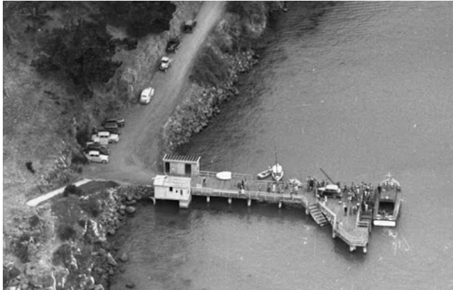
Source: V.C. Browne & Son (Note: Photograph has been cropped). Aerial view of Diamond Harbour 1949. The two shelters at the landward end of the wharf are visible in their original form. The photo pre-dates the construction of the Sea Scout's boat canopy and the dinghy shelter. The current small crane can be seen behind the car on the wharf.
