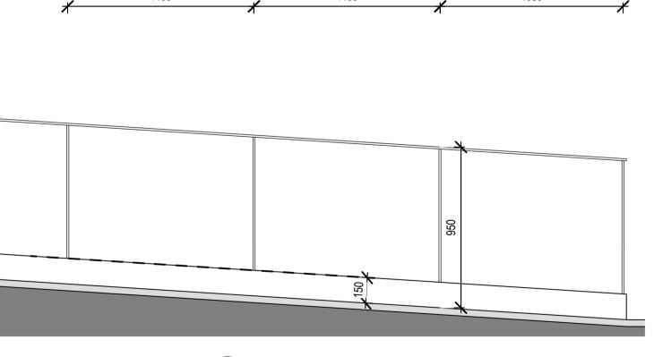
6 Hand rail on ramp A1 sheet scale = 1 : 20 A3 sheet scale is twice scale shown above ☐ All dimension to be verified on site before producing shop drawings or commencing any work.
