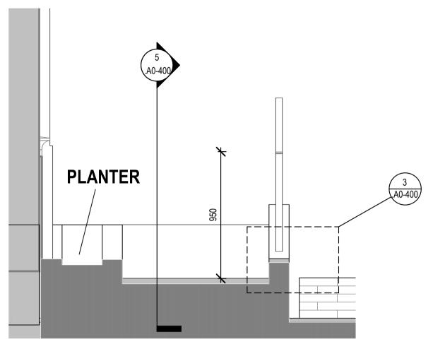
4 Cross Section through Ramp A1 sheet scale = 1:20 A3 sheet scale is twice scale shown above
