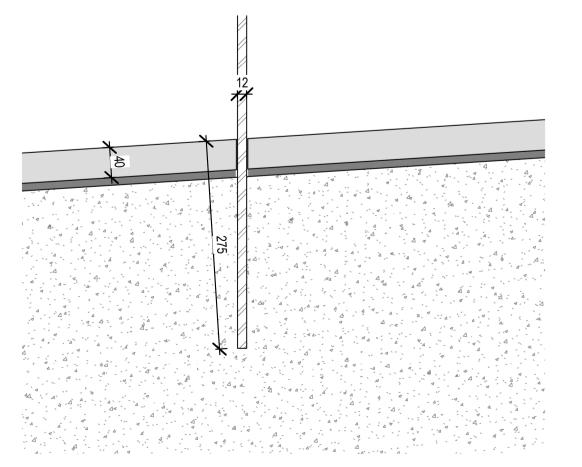
8 Detail Handrail Base .A0-400 A1 sheet scale = 1:5 A3 sheet scale is twice scale shown above
