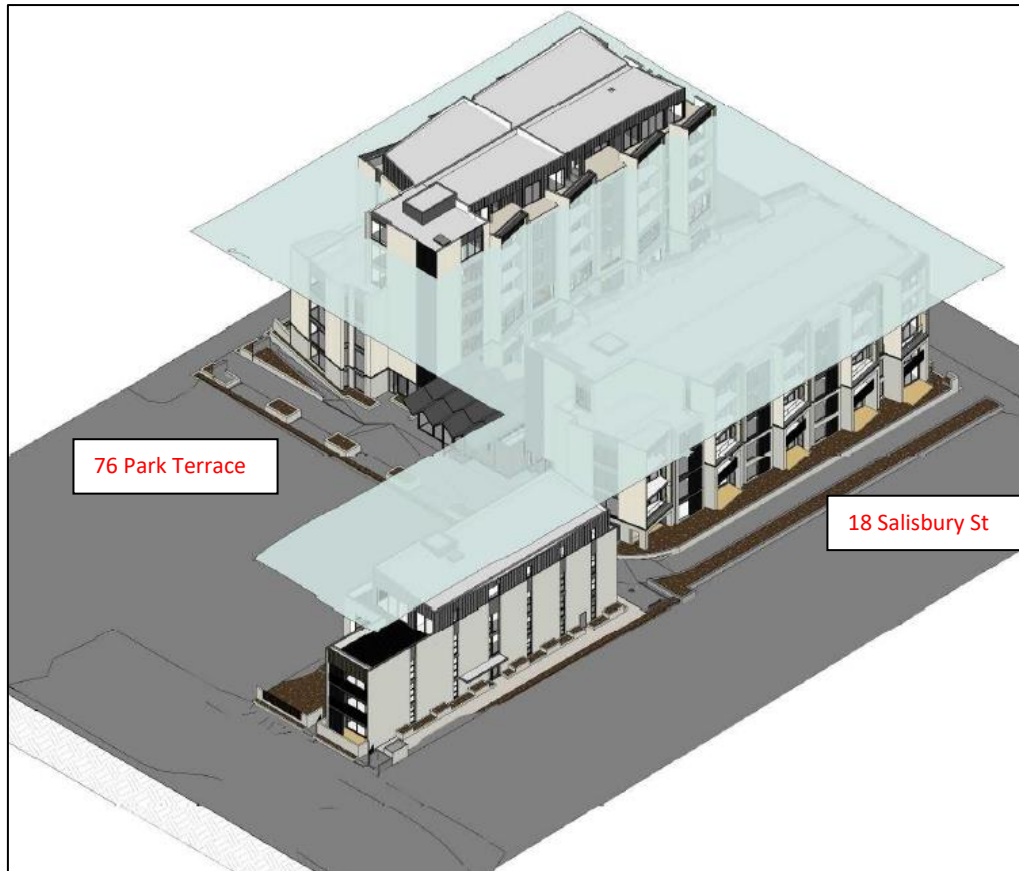
Figure 3: View looking northwest showing extent of the breach of Building 7's western wing through the 20m height limit.
