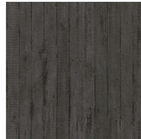
vertical 'off the form' precast concrete charcoal
