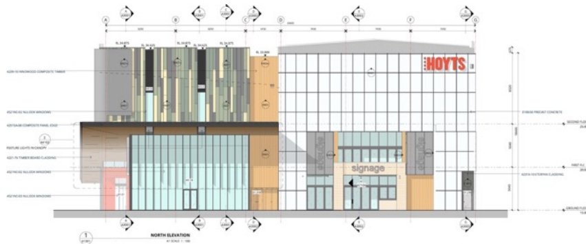
Figure 16: The north elevation of the EntX building, currently under construction. The size and corner location of the digital screen on this elevation is indicated by the grey panel in the top left hand corner of the elevation.
