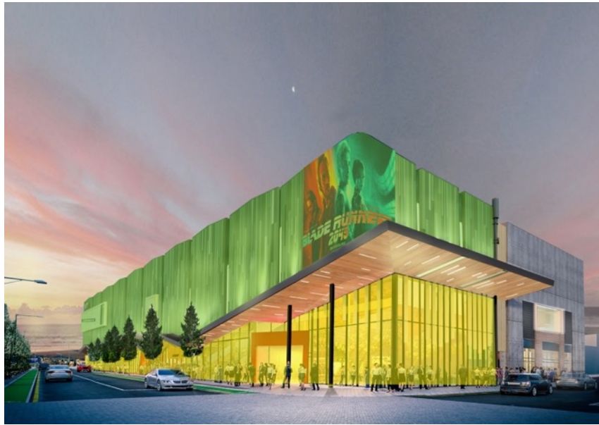
Figure 31: The two main components of the EntX building form. The highly glazed lower level (shaded yellow) is visually distinct from the largely enclosed upper two floors (shaded green). The variously sloping veranda mediates between these two main components of the building form.
