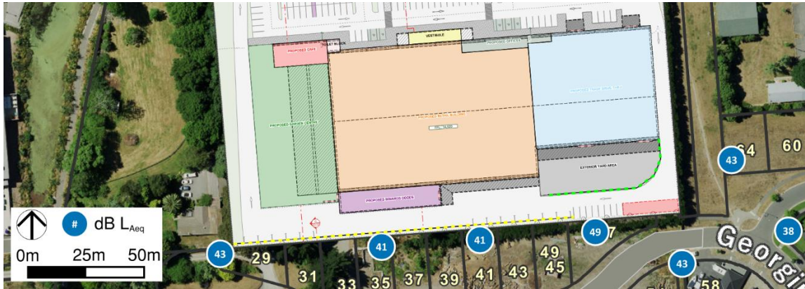
Figure 6: The predicted noise levels (dB L Aeq ) at adjacent single level property boundaries
