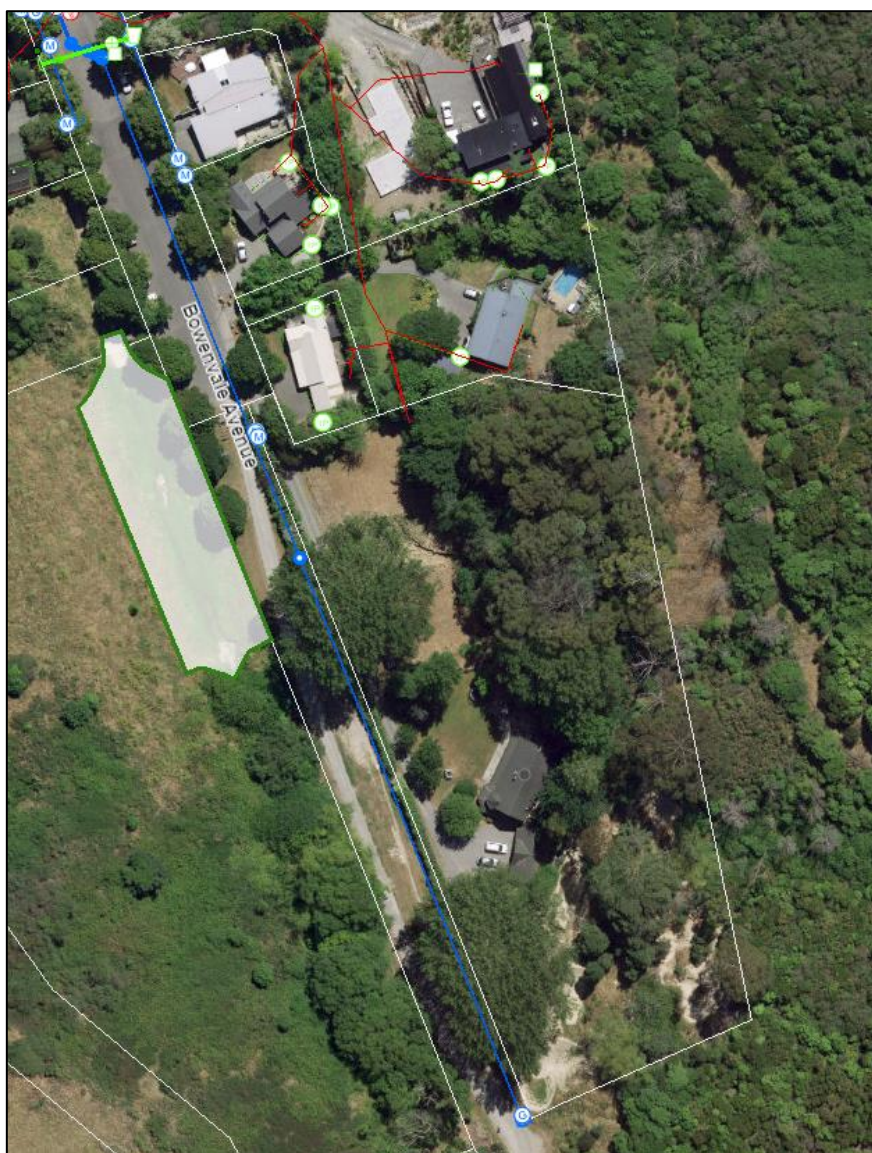
Figure 2: Existing services at 169 Bowenvale Ave. (Source: Christchurch City Council three waters advanced asset network map).
