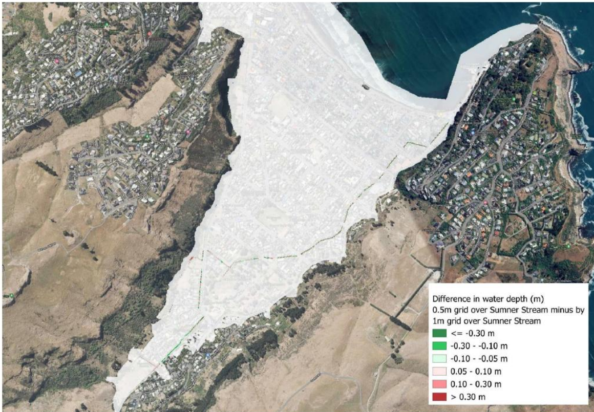
Figure 3 Difference in water depth (0.5m grid over Sumner Steam minus by 1m grid over Sumner Stream) under March 2014 event
