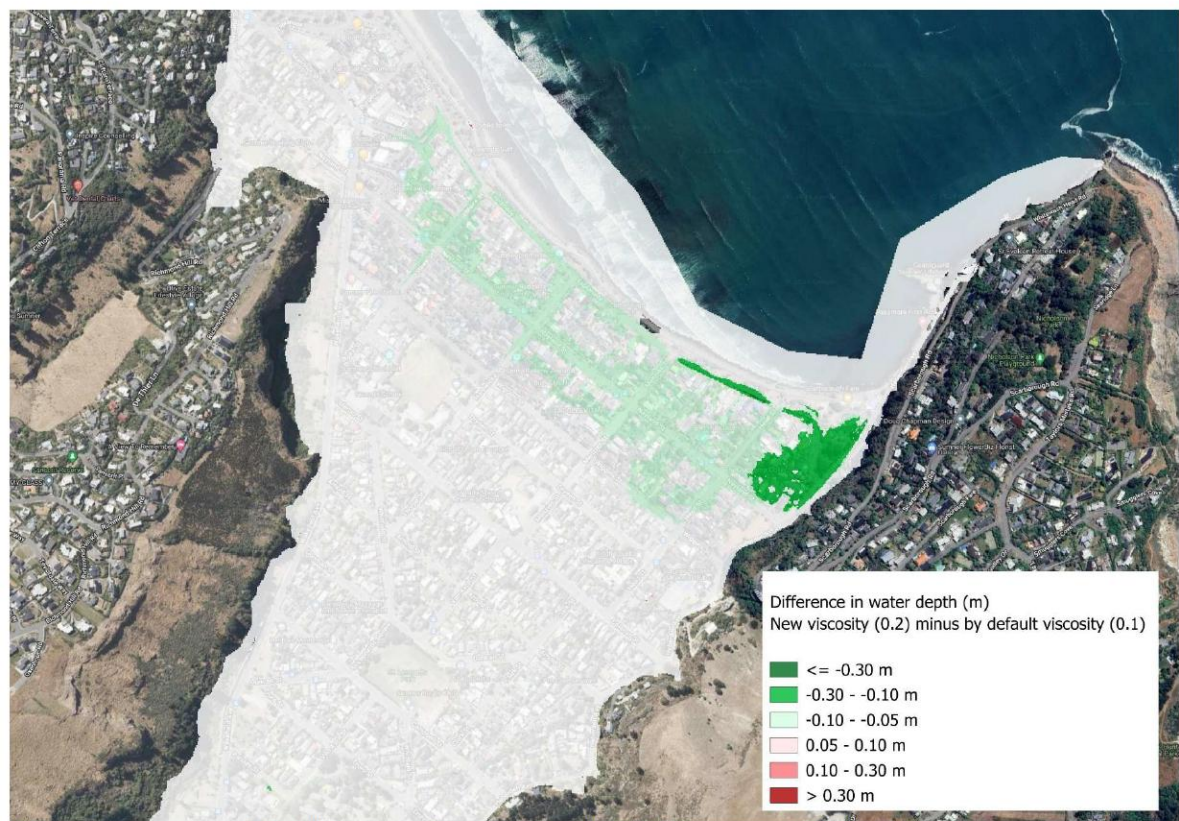
Figure 2 Difference in water depth (Viscosity coefficient = 0.2 minus by default viscosity) under March 2014 event
