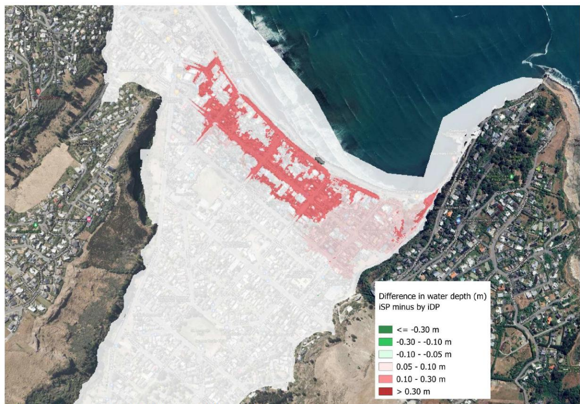
Figure 1 Difference in water depth (iSP minus by iDP) under March 2014 event
