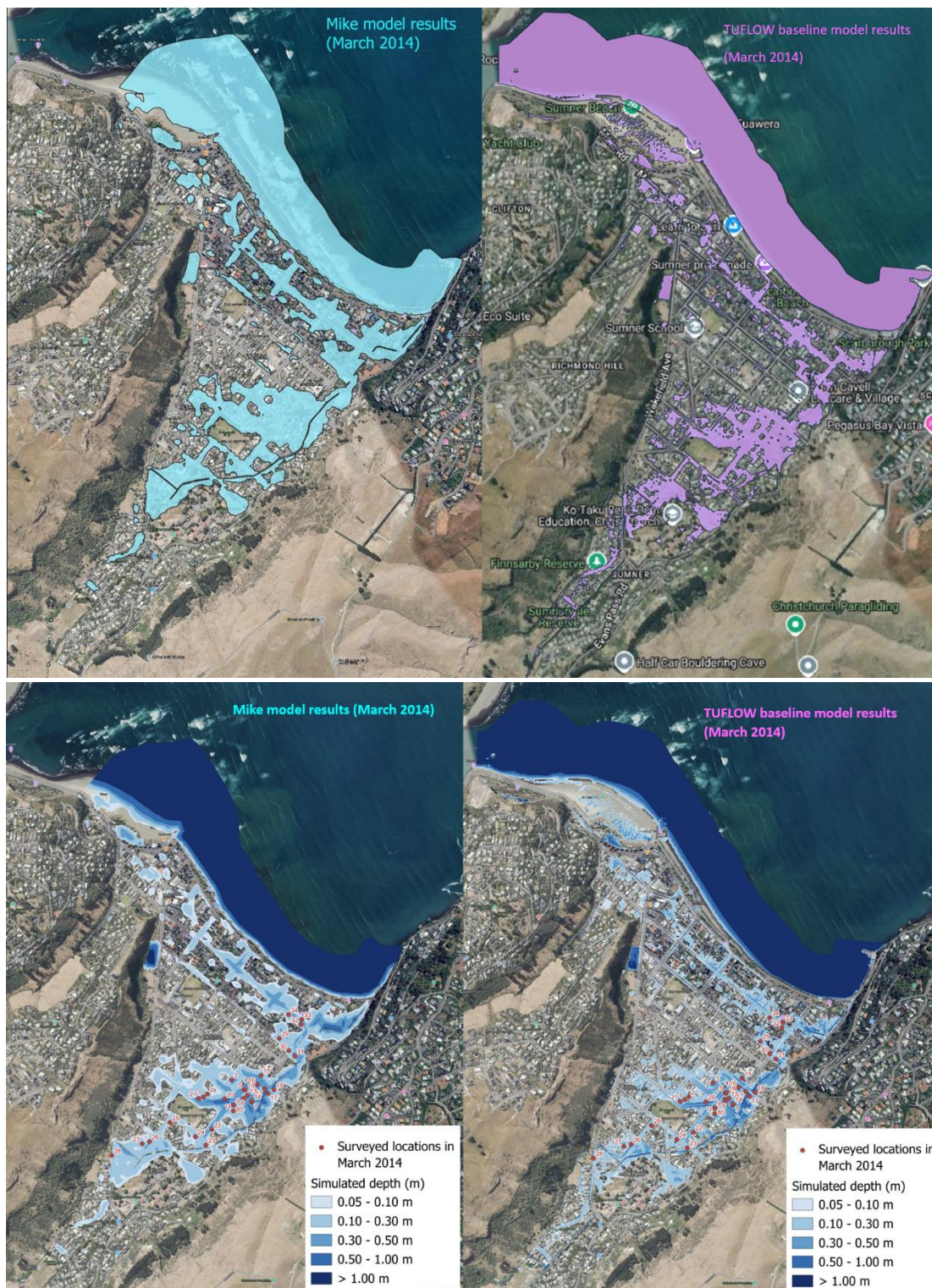
Figure 12. Comparison between TUFLOW baseline model results and MIKE model results for the March 2014 storm event - flood extent (top) and flood depth with surveyed locations (bottom).
