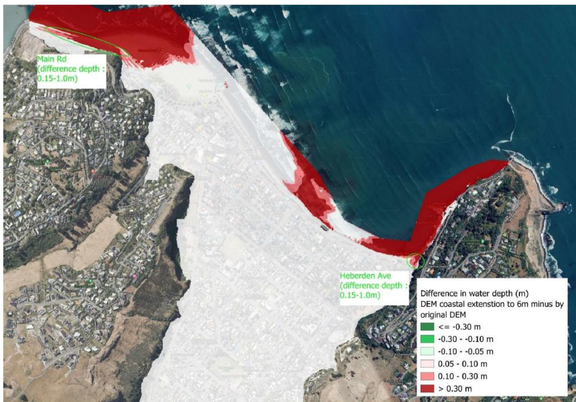
Figure 4 Difference in water depth (DEM coastal extension to 6mRL minus by original DEM) under March 2014 event
