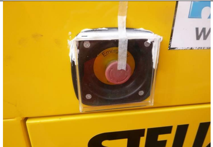
Figure 34: Emergency STOP button with Perspex
