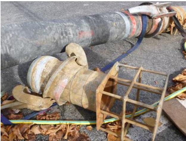
Figure 10: Layflat Pipe: Strainer for suction hose
