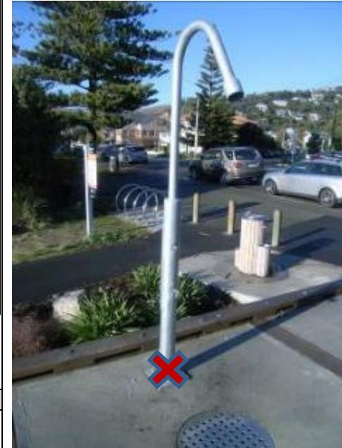
Steel shower, galvanised surface finish, one shower head, and a tap, and a grate to the wastewater system.
