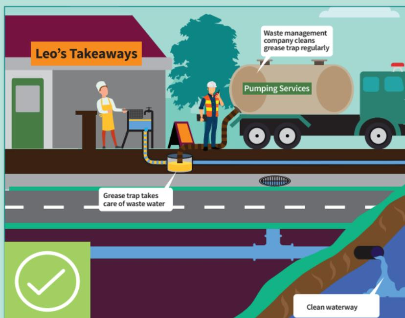
Leo's Takeaways have a standard grease trap which takes care of their waste water. They also engage a waste management company to regularly clean and maintain the grease trap. This system takes Leo's waste water straight from their kitchen to Christchurch's treatment plan, without any problem, leaving Leo to get on with business.
