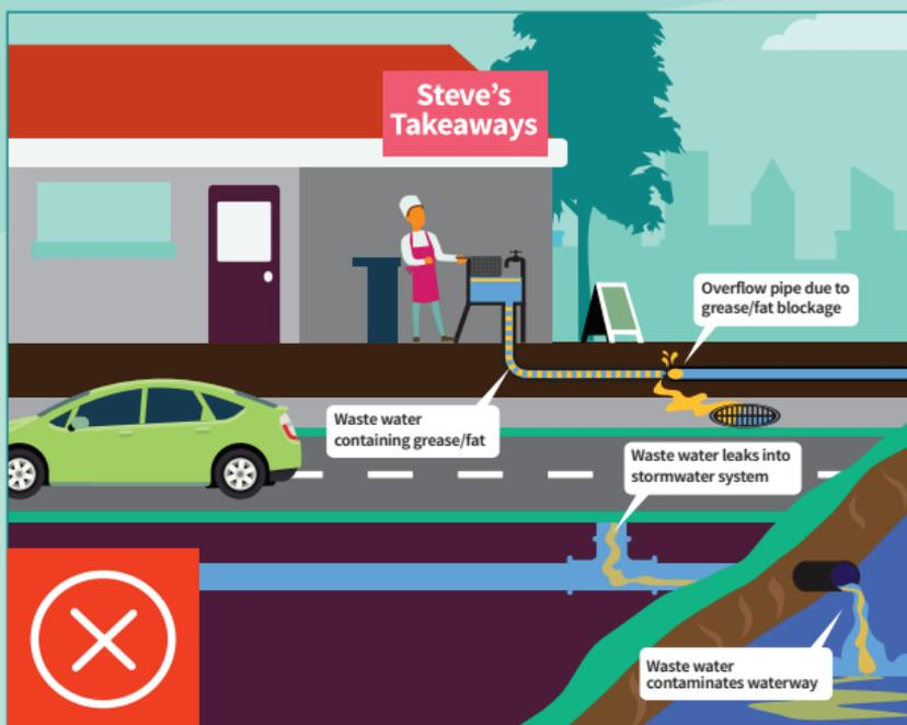
Steve's Takeaways don't have a grease trap. This has caused a large blockage in the city's sewer which also flooded Steve's building. Additionally, the blockage led to a waste overflow into the Avon River. This cost the city money to fix and clean up; costs which Steve's Takeaways had to repay.
