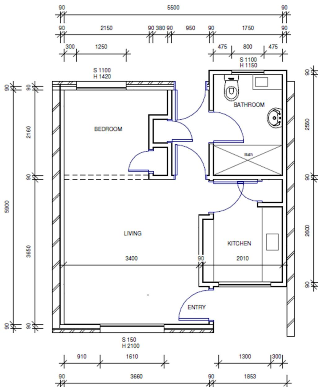
Figure 4: Floor Plan of a Residential Unit.
