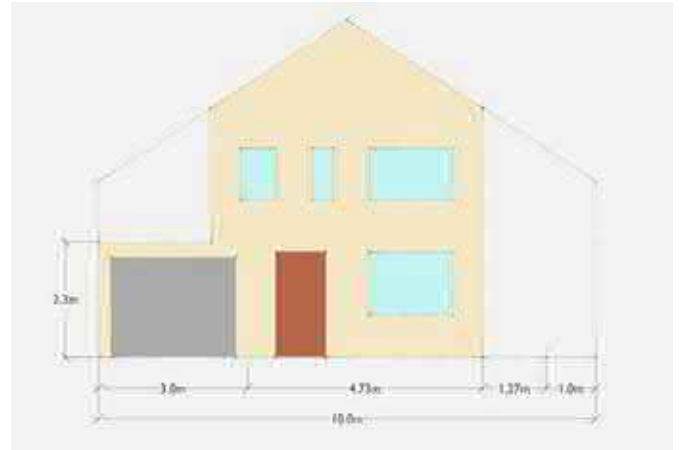
Building envelope for a standalone, two storey house on a 10m wide N-S orientated lot.
