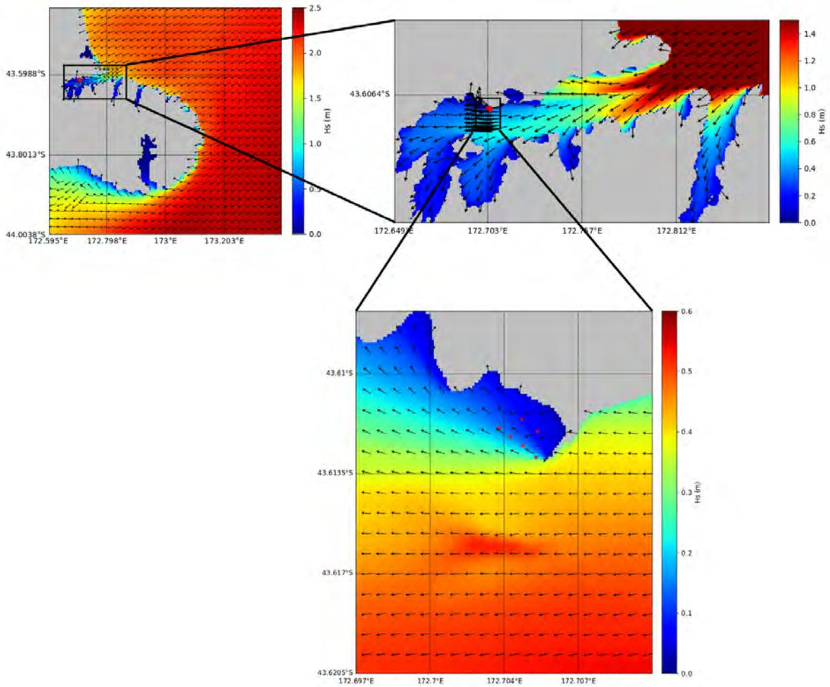
Figure 2.1 Example of modelled  $H_s$  field output for waves incoming from the NE sector for the 3 last SWAN nests. Vectors represent modelled wave direction.
