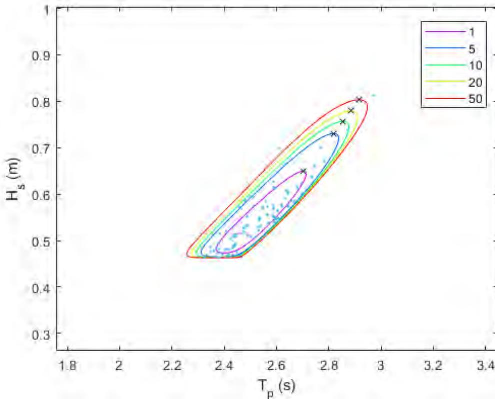
Figure 2.4 Contour plot of omni-directional bi-variate ( $H_s$ - $T_p$ ) return period values for 1, 5, 10, 20 and 50-year ARIs. The dark crosses correspond to the estimated deterministic  $H_s$  and associated  $T_p$  return period values for each ARI indicated in the legend at P0.
