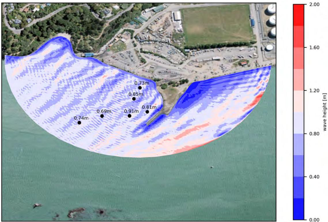
Figure 3.9 Surface elevation modelled for existing layout with South-westerly waves:  $H_s=0.73\text{m}$ ;  $T_p=3\text{s}$ , (5-year return period, top panel) and  $H_s=0.8\text{m}$ ,  $T_p=3\text{s}$  (50 year return period, bottom panel).
