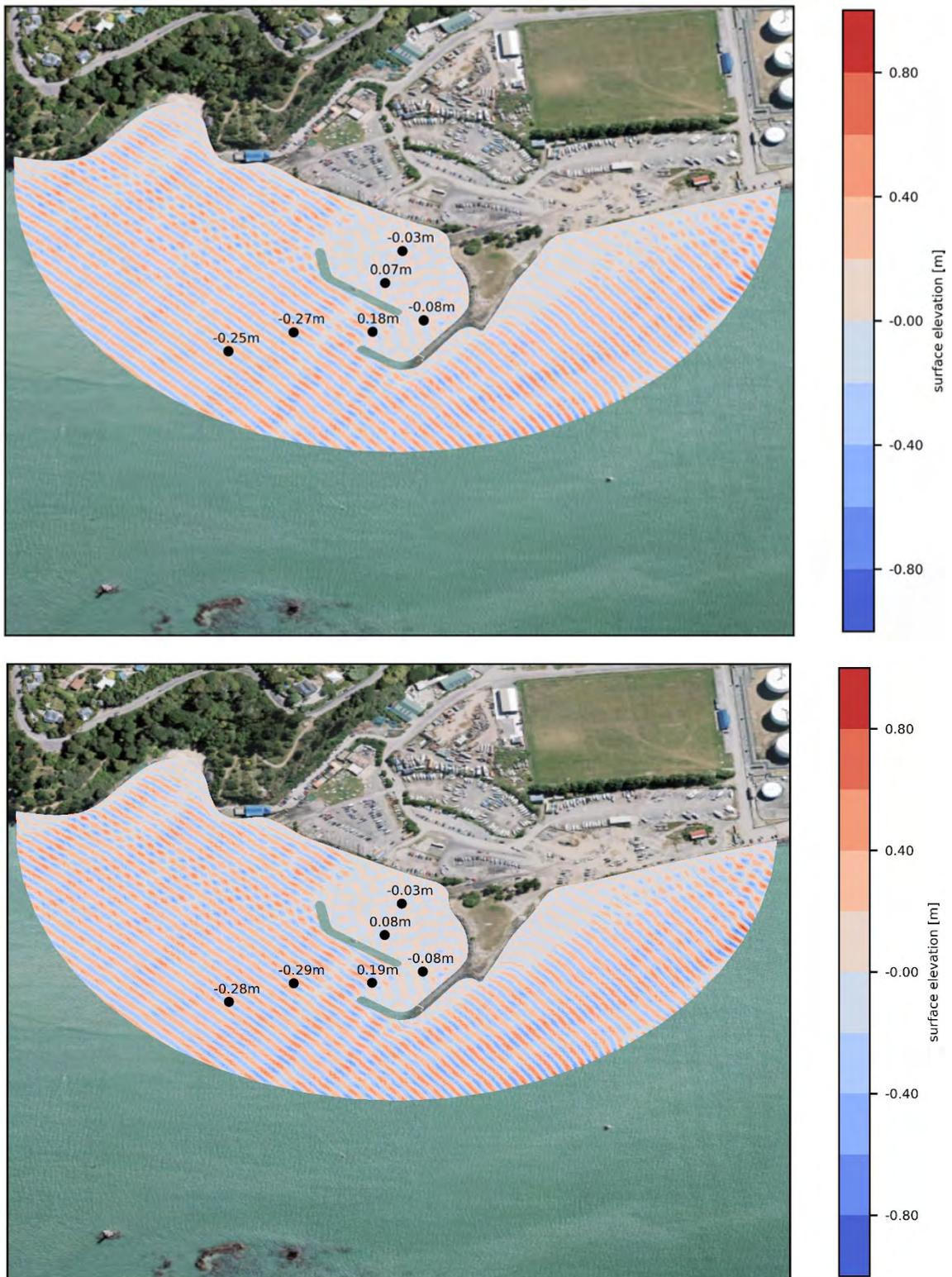
Figure 3.23 Surface elevation modelled for design layout 2 with South-westerly waves:  $H_s=0.73\text{m}$ ;  $T_p=3\text{s}$  (5 year return period, top panel) and  $H_s=0.80\text{m}$ ,  $T_p=3\text{s}$  (50 year return period, bottom panel).
