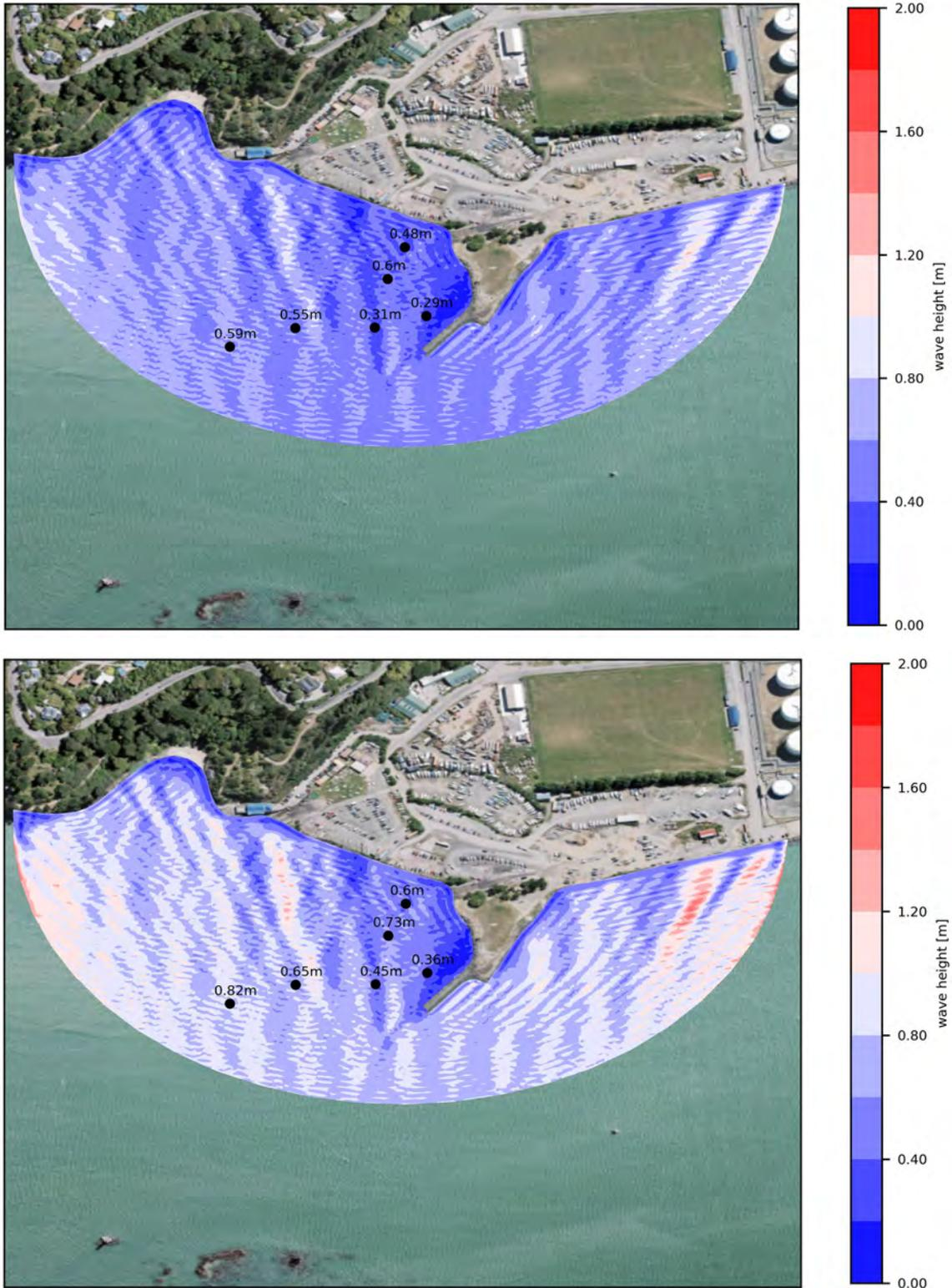
Figure 3.7 Wave height modelled for existing layout with Southerly waves:  $H_s=0.53\text{m}$ ;  $T_p=3\text{s}$  (5-year return period, top panel) and  $H_s=0.72\text{m}$ ,  $T_p=3\text{s}$  (50-year return period, bottom panel).
