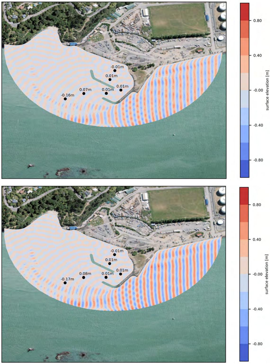
Figure 7.17 Surface elevation modelled for design layout 2 with Easterly waves:  $H_s=0.83\text{m}$ ;  $T_p=4\text{s}$  (5-year return period, top panel) and  $H_s=0.98\text{m}$ ,  $T_p=4\text{s}$  (50-year return period, bottom panel).
