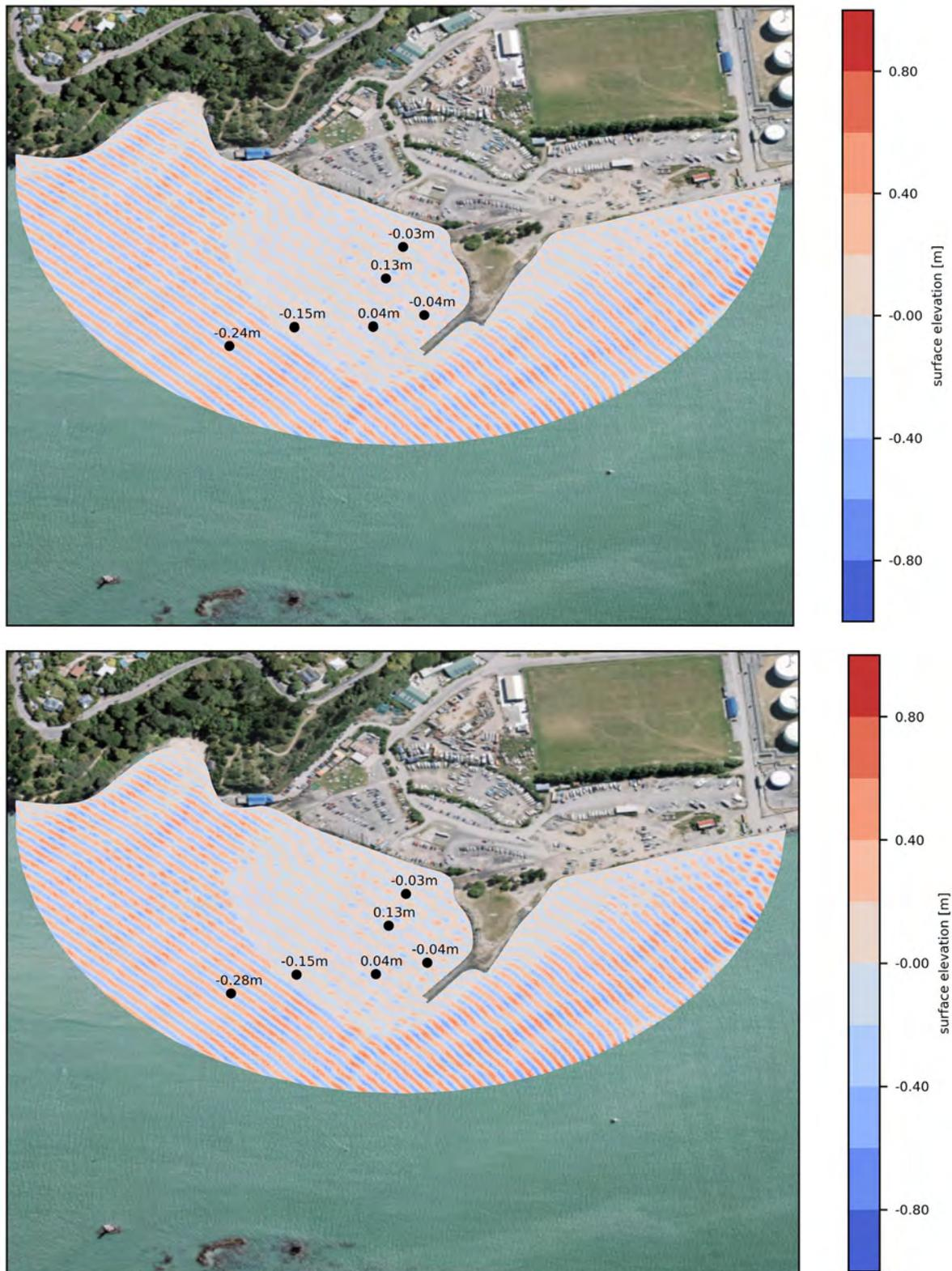
Figure 3.16 Surface elevation modelled for design layout 1 with South-westerly waves:  $H_s=0.73\text{m}$ ;  $T_p=3\text{s}$  (5 year return period, top panel) and  $H_s=0.80\text{m}$ ,  $T_p=3\text{s}$  (50 year return period, bottom panel).
