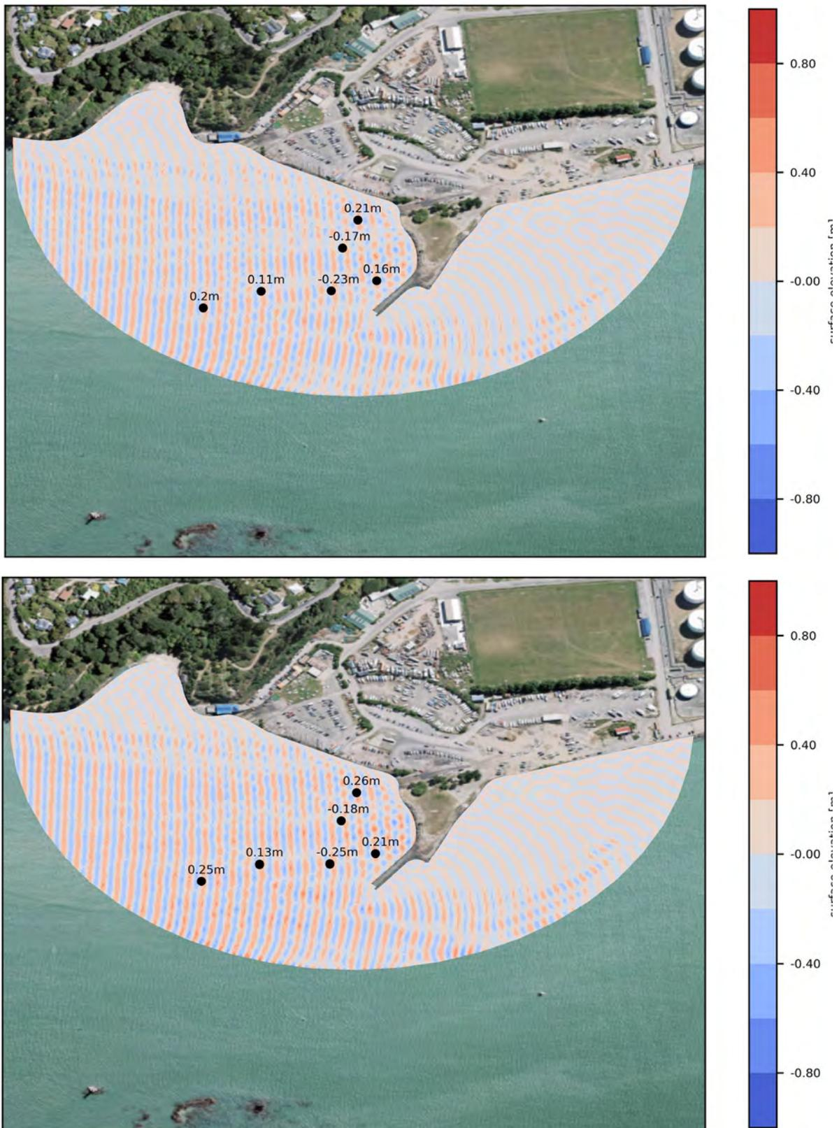
Figure 3.10 Surface elevation modelled for existing layout with Westerly waves:  $H_s=0.54\text{m}$ ;  $T_p=3\text{s}$  (5 year return period, top panel) and  $H_s=0.65\text{m}$ ,  $T_p=3\text{s}$  (50 year return period, bottom panel).
