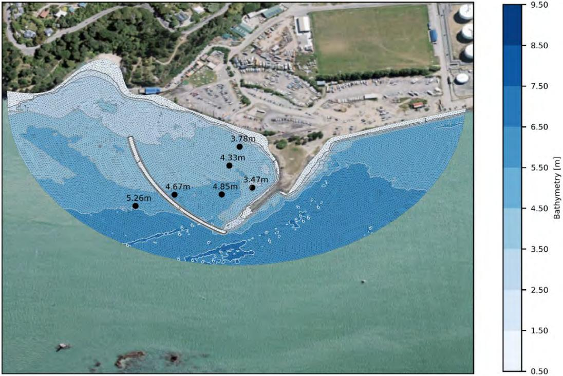
Figure 3.2 The computational domain and bathymetry used for the design layout 1 with a wave attenuator (length =265m, width= 5m, draft =1.5m; transmission coefficient = 0.3)
