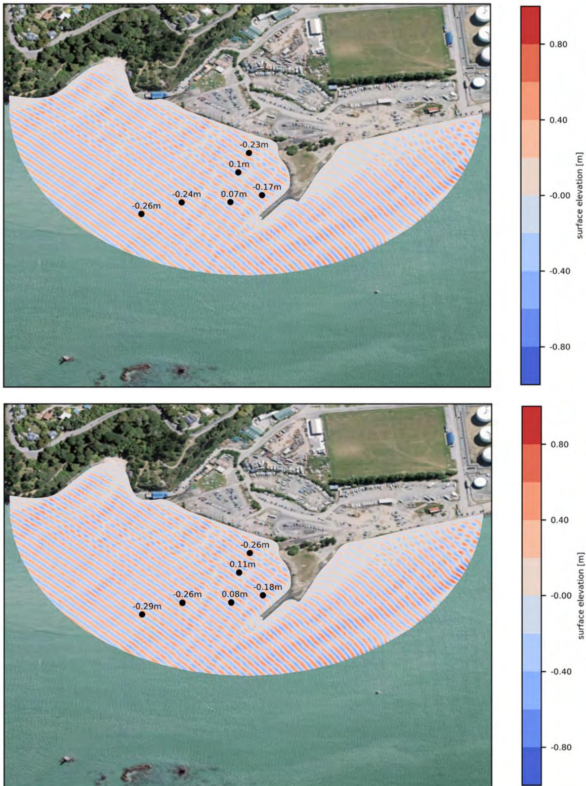
Figure 3.8 Surface elevation modelled for existing layout with South-westerly waves:  $H_s=0.73\text{m}$ ;  $T_p=3\text{s}$  (5-year return period, top panel) and  $H_s=0.8\text{m}$ ,  $T_p=3\text{s}$  (50-year return period, bottom panel).
