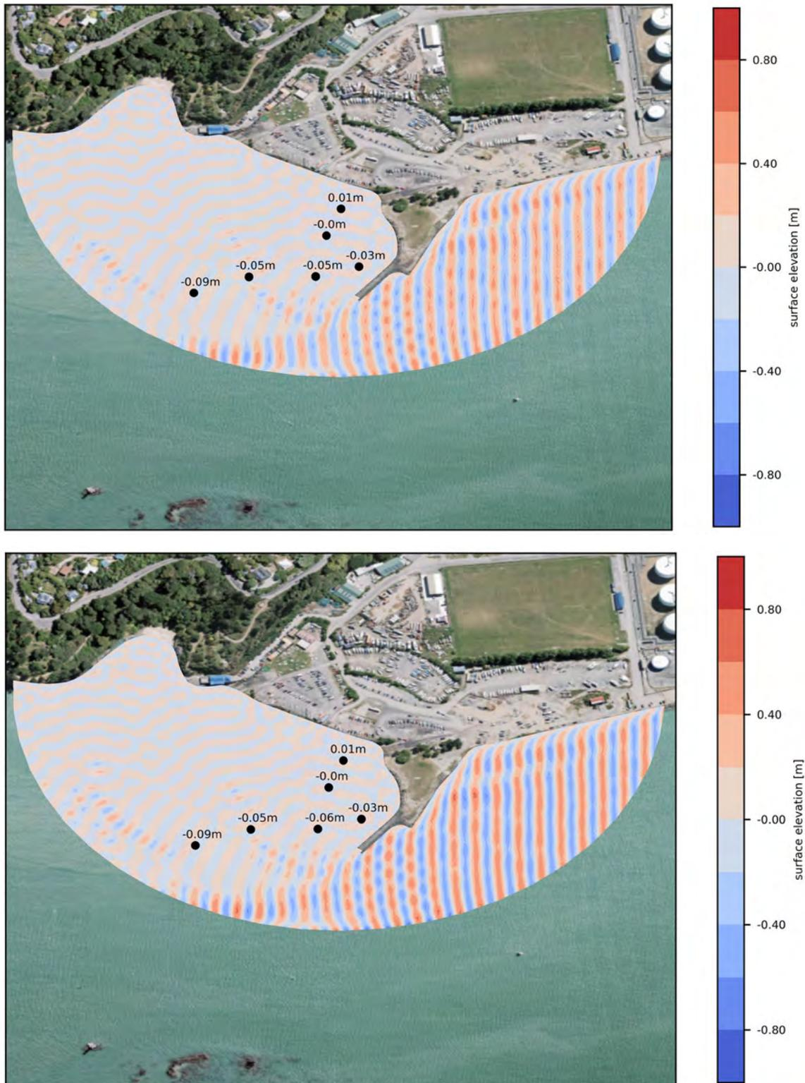
Figure 3.12 Surface elevation modelled for design layout 1 with Easterly waves:  $H_s=0.83\text{m}$ ;  $T_p=4\text{s}$  (5 year return period, top panel) and  $H_s=0.98\text{m}$ ,  $T_p=4\text{s}$  (50 year return period, bottom panel).
