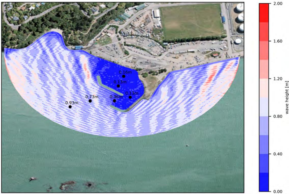
Figure 3.22 Wave height modelled for design layout 2 with Southerly waves:  $H_s=0.53\text{m}$ ;  $T_p=3\text{s}$  (5 year return period, top panel) and  $H_s=0.72\text{m}$ ,  $T_p=3\text{s}$  (50 year return period, bottom panel).
