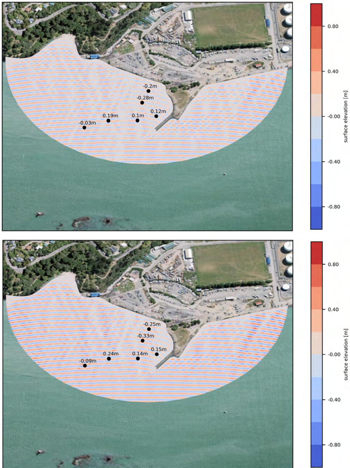
Figure 3.6 Surface elevation modelled for existing layout with Southerly waves:  $H_s=0.53m$ ,  $T_p=3s$  (5-year return period, top panel) and  $H_s=0.72m$ ,  $T_p=3s$  (50-year return period, bottom panel).
