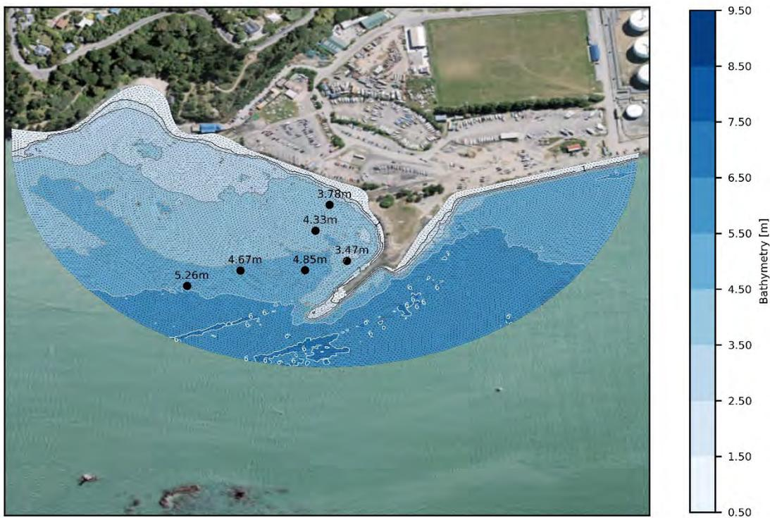
Figure 3.1 The computational mesh and bathymetry for the existing layout
