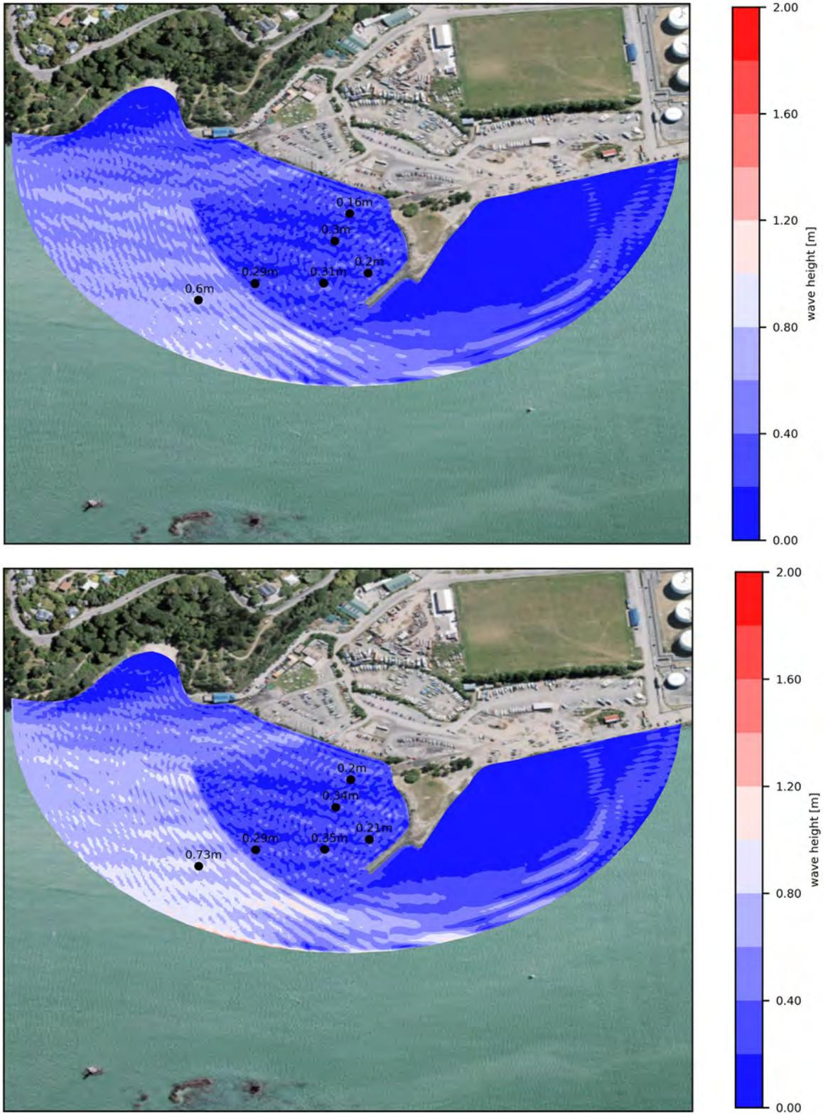
Figure 3.19 Surface elevation modelled for design layout 1 with Westerly waves:  $H_s=0.54\text{m}$ ;  $T_p=3\text{s}$  (5 year return period, top panel) and  $H_s=0.65\text{m}$ ,  $T_p=3\text{s}$  (50 year return period, bottom panel).
