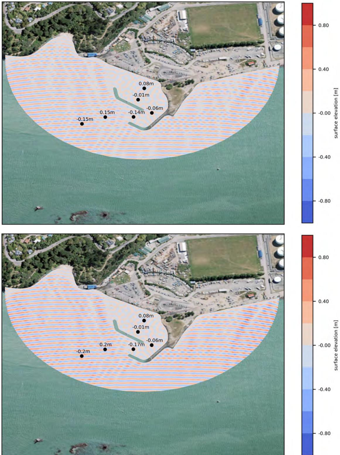
Figure 3.21 Surface elevation modelled for design layout 2 with Southerly waves:  $H_s=0.53\text{m}$ ;  $T_p=3\text{s}$  (5 year return period, top panel) and  $H_s=0.72\text{m}$ ,  $T_p=3\text{s}$  (50 year return period, bottom panel).
