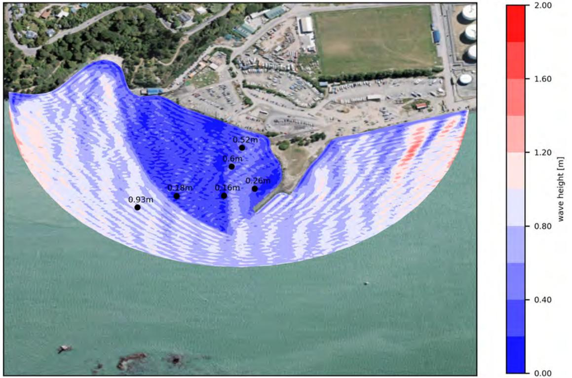
Figure 3.15 Surface elevation modelled for design layout 1 with Southerly waves:  $H_s=0.53\text{m}$ ,  $T_p=3\text{s}$  (5 year return period, top panel) and  $H_s=0.72\text{m}$ ,  $T_p=3\text{s}$  (50 year return period, bottom panel).
