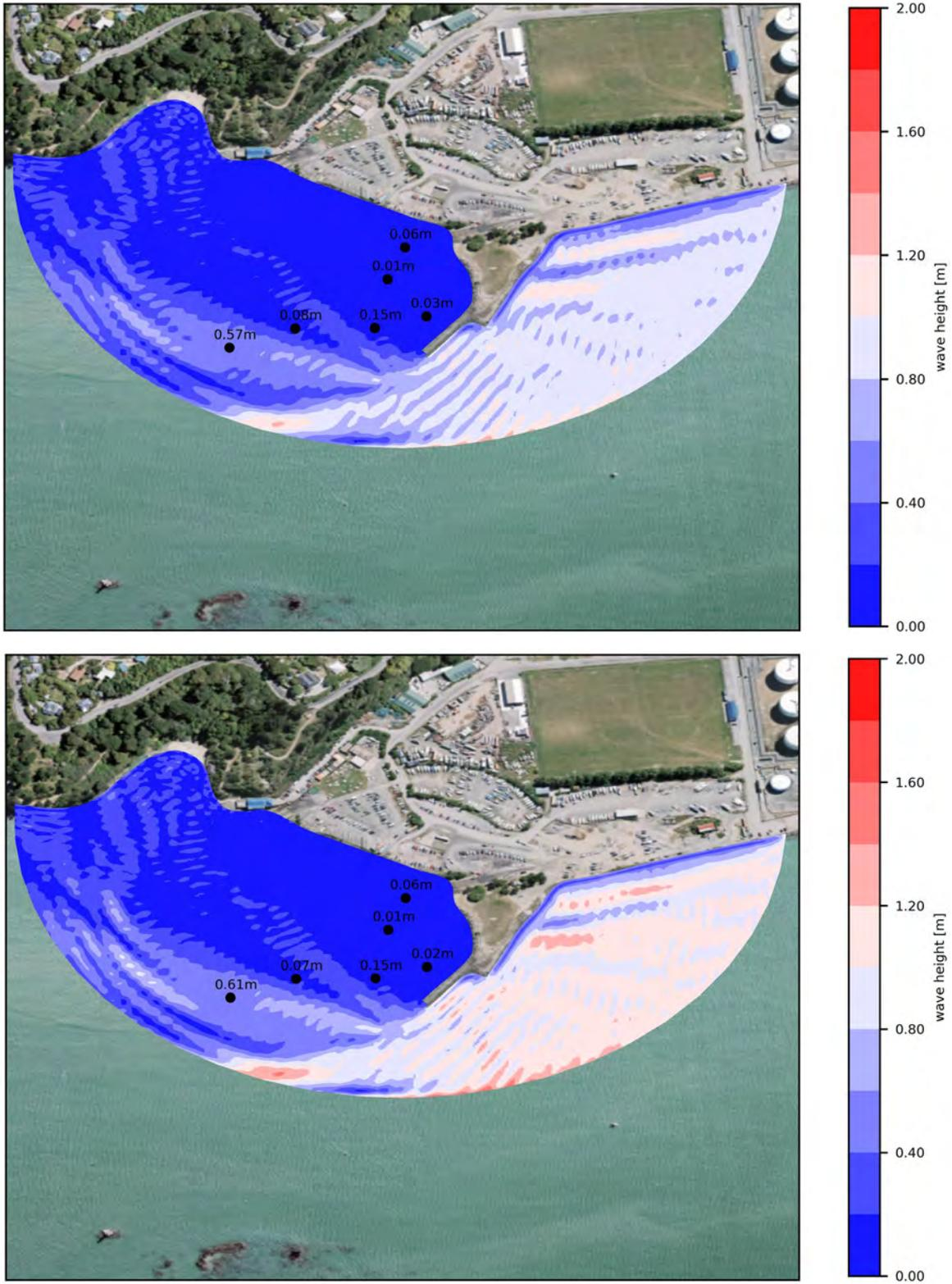
Figure 3.5 Wave height modelled for existing layout with Easterly waves:  $H_s=0.83\text{m}$ ;  $T_p=4\text{s}$  (5-year return period, top panel) and  $H_s=0.98\text{m}$ ,  $T_p=4\text{s}$  (50 year return period, bottom panel).
