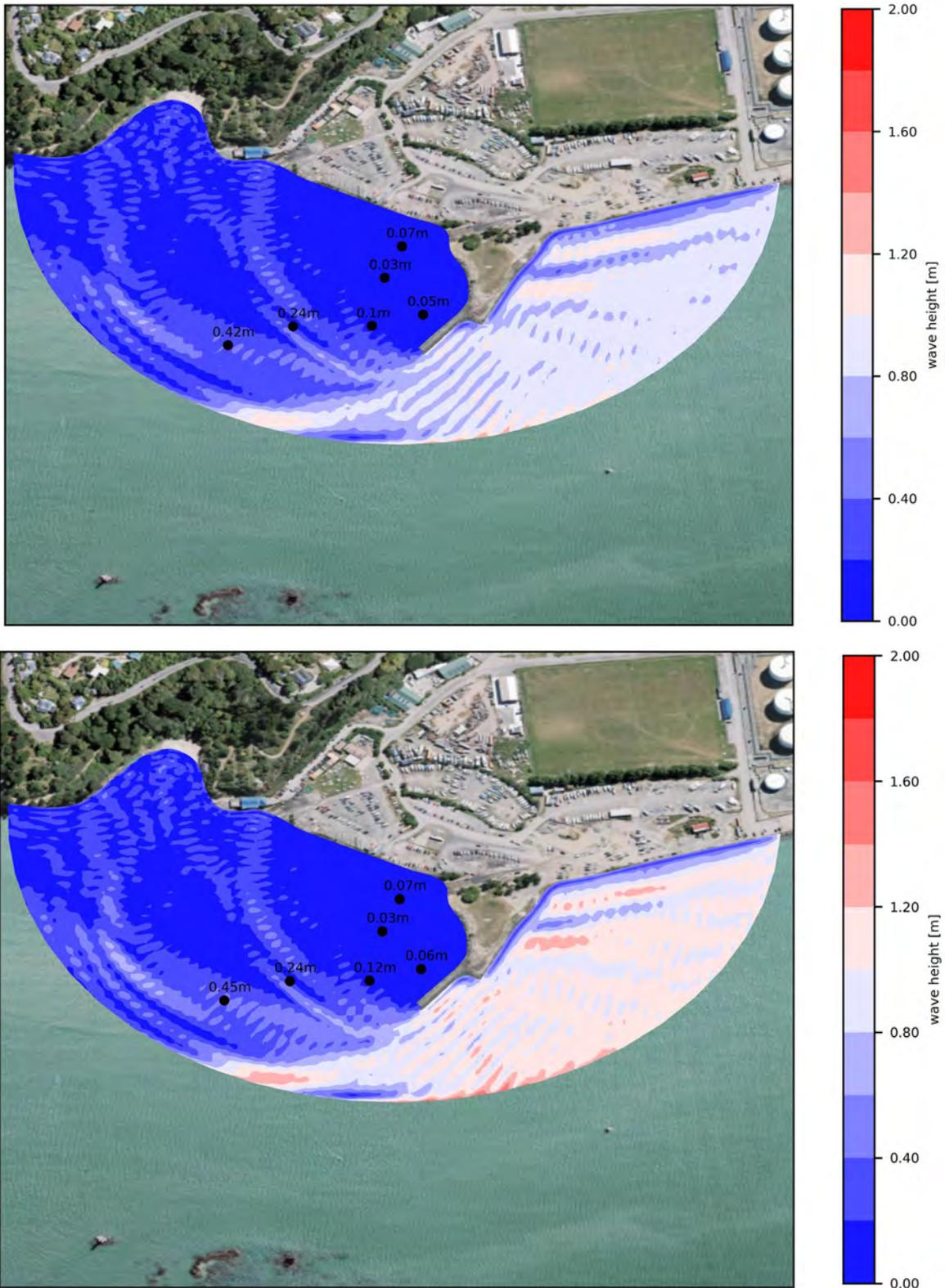
Figure 3.13 Wave height modelled for design layout 1 with Easterly waves:  $H_s=0.83\text{m}$ ;  $T_p=4\text{s}$  (5 year return period, top panel) and  $H_s=0.98\text{m}$ ,  $T_p=4\text{s}$  (50 year return period, bottom panel).
