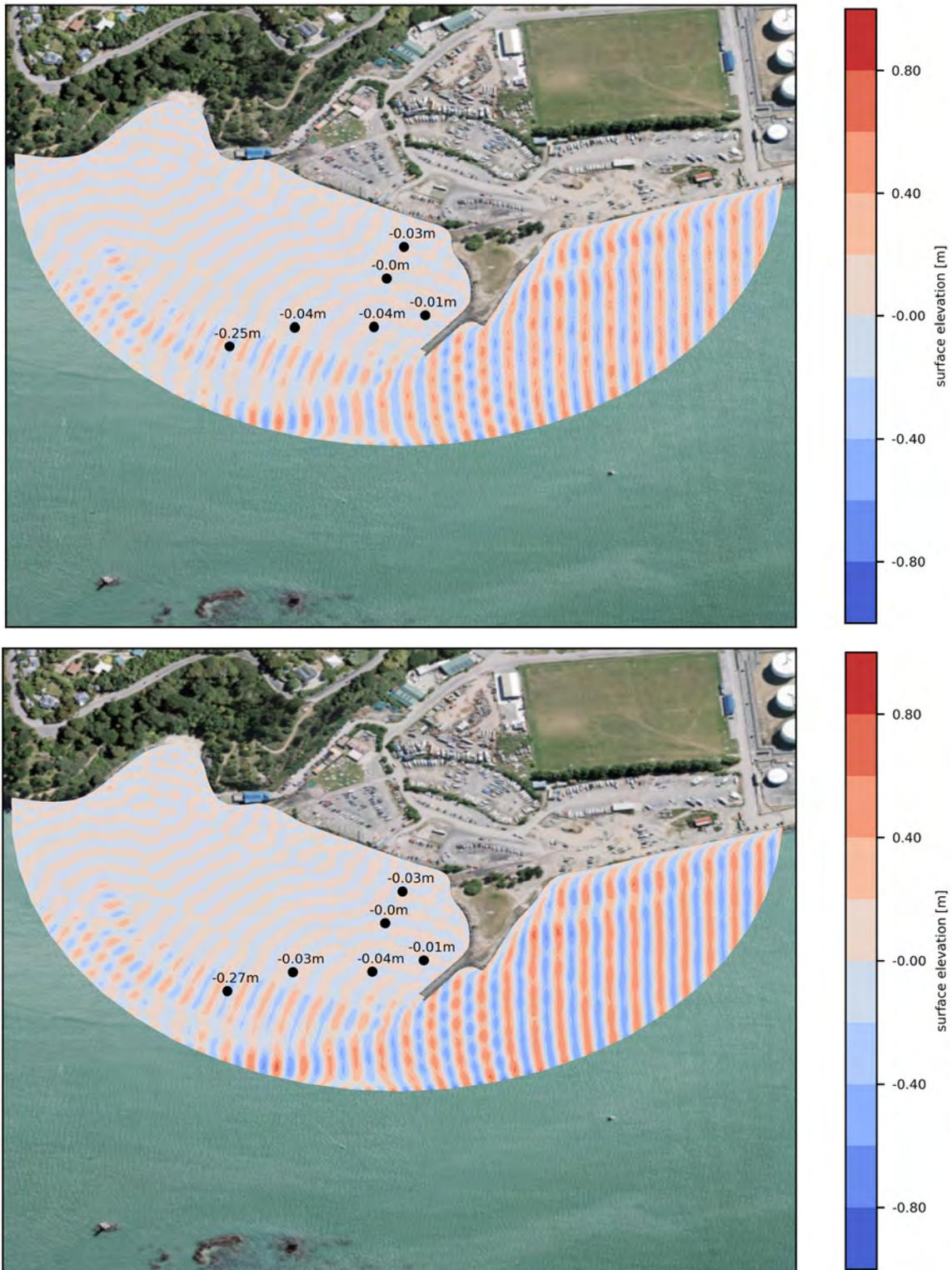
Figure 3.4 The surface elevation modelled for existing layout with Easterly waves:  $H_s=0.83\text{m}$ ;  $T_p=4\text{s}$  (5-year return period, top panel) and  $H_s=0.98\text{m}$ ,  $T_p=4\text{s}$  (50 year return period, bottom panel).
