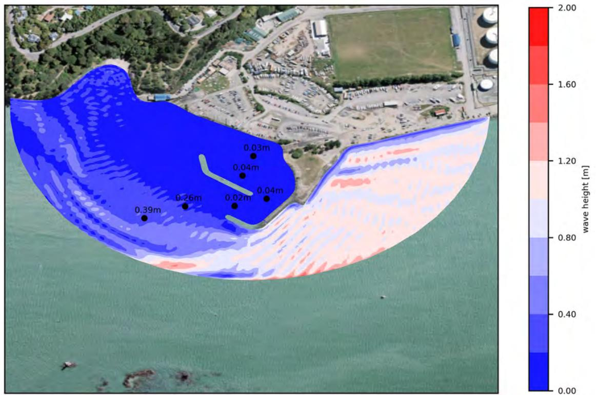
Figure 3.20 Wave height modelled for design layout 2 with Easterly waves:  $H_s=0.83\text{m}$ ;  $T_p=4\text{s}$  (5 year return period, top panel) and  $H_s=0.98\text{m}$ ,  $T_p=4\text{s}$  (50 year return period, bottom panel).
