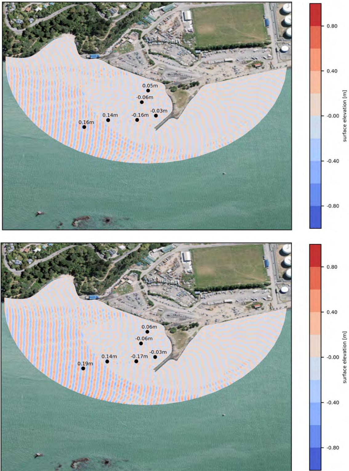
Figure 3.18 Surface elevation modelled for design layout 1 with Westerly waves:  $H_s=0.54\text{m}$ ;  $T_p=3\text{s}$  (5 year return period, top panel) and  $H_s=0.65\text{m}$ ,  $T_p=3\text{s}$  (50 year return period, bottom panel).
