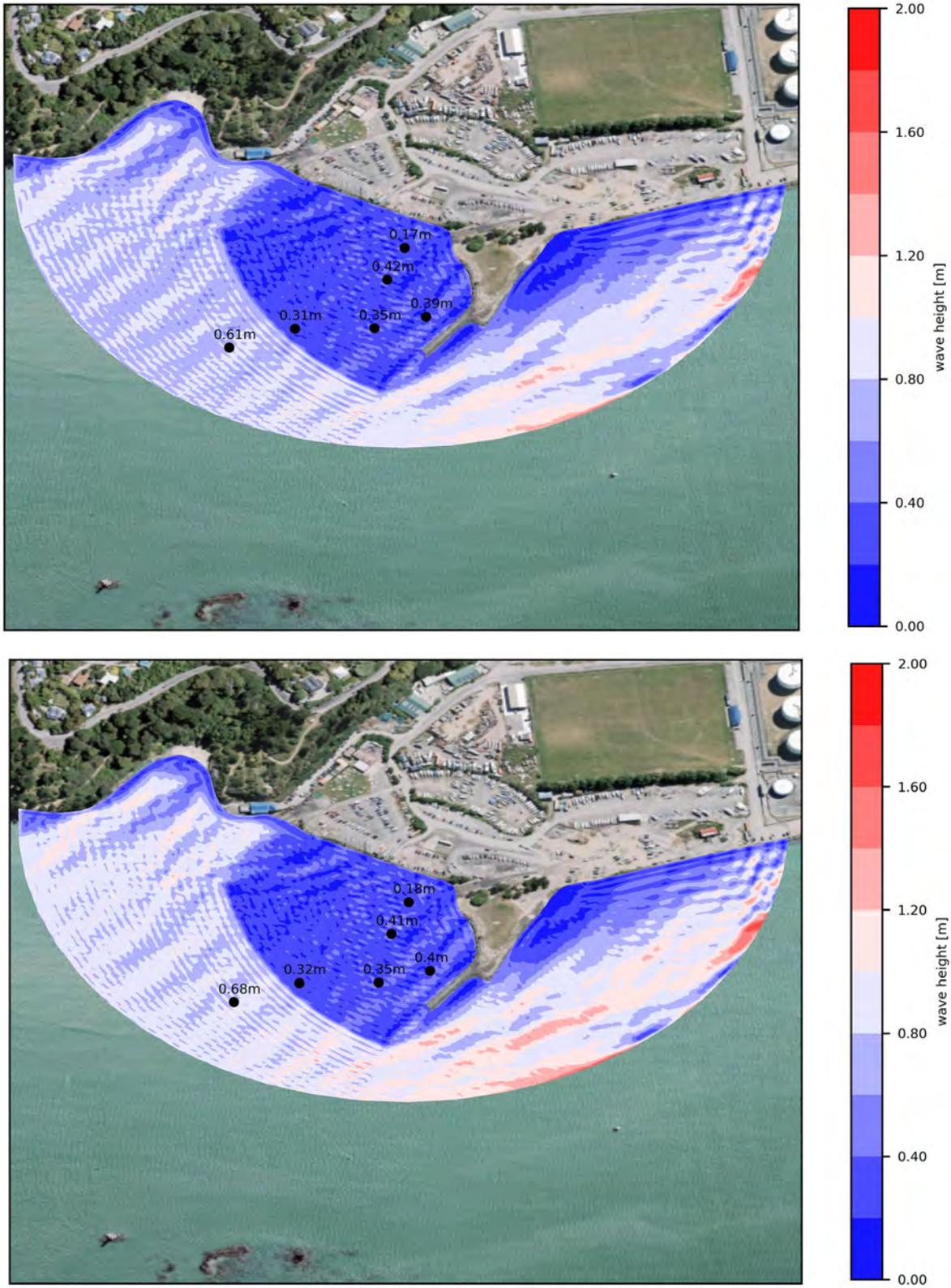
Figure 3.17 Wave height modelled for design layout 1 with South-westerly waves:  $H_s=0.73m$ ;  $T_p=3s$  (5 year return period, top panel) and  $H_s=0.80m$ ,  $T_p=3s$  (50 year return period, bottom panel).
