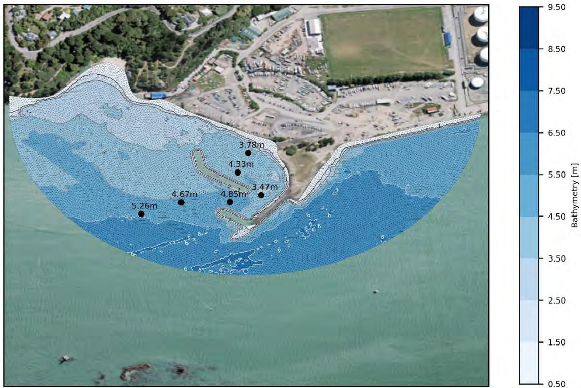
Figure 3.3 The computational domain and bathymetry used for design layout 2 (with two rock breakwaters)
