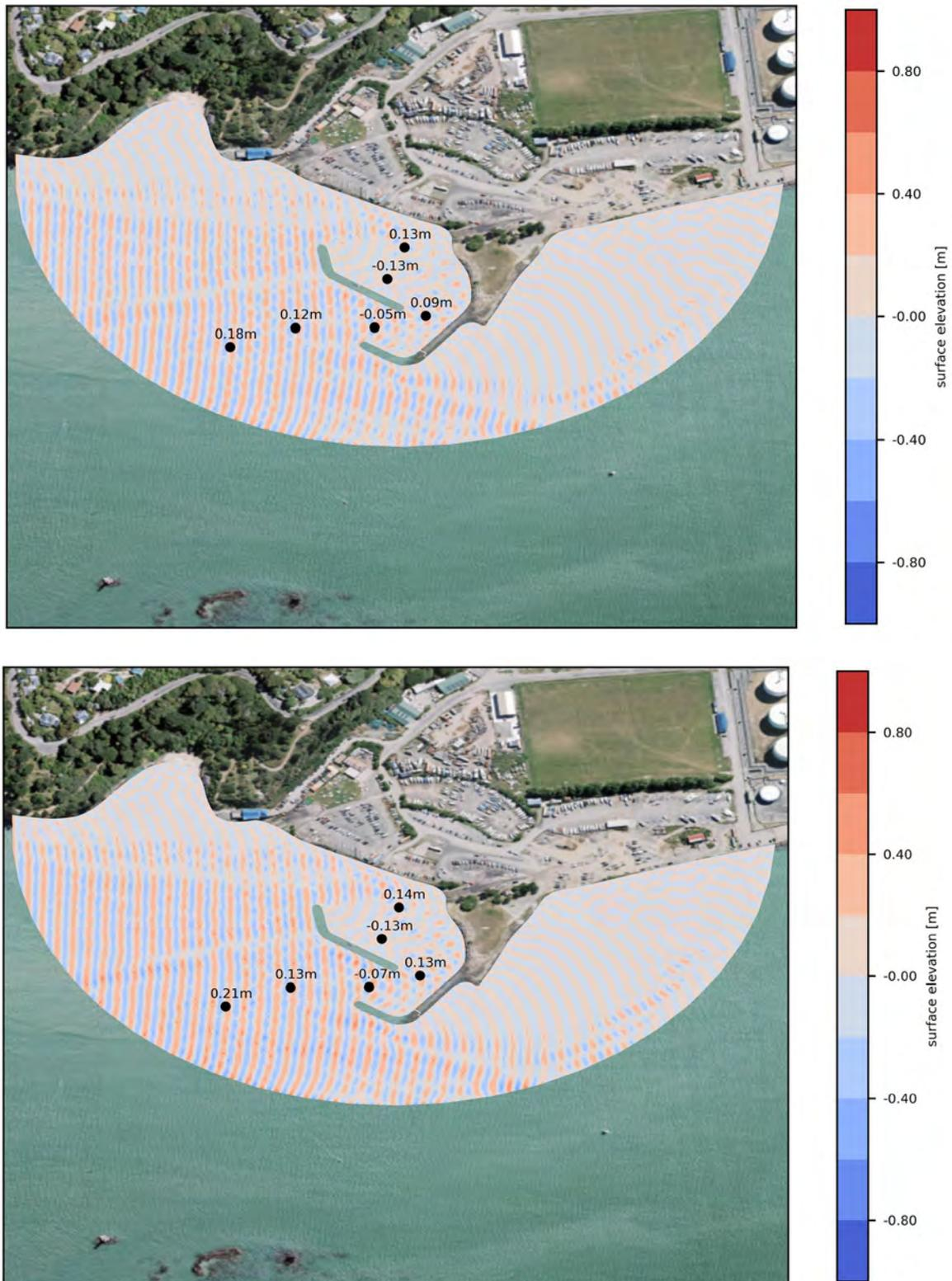
Figure 3.25 Surface elevation modelled for design layout 2 with Westerly waves:  $H_s=0.54\text{m}$ ;  $T_p=3\text{s}$  (5 year return period, top panel) and  $H_s=0.65\text{m}$ ,  $T_p=3\text{s}$  (50 year return period, bottom panel).
