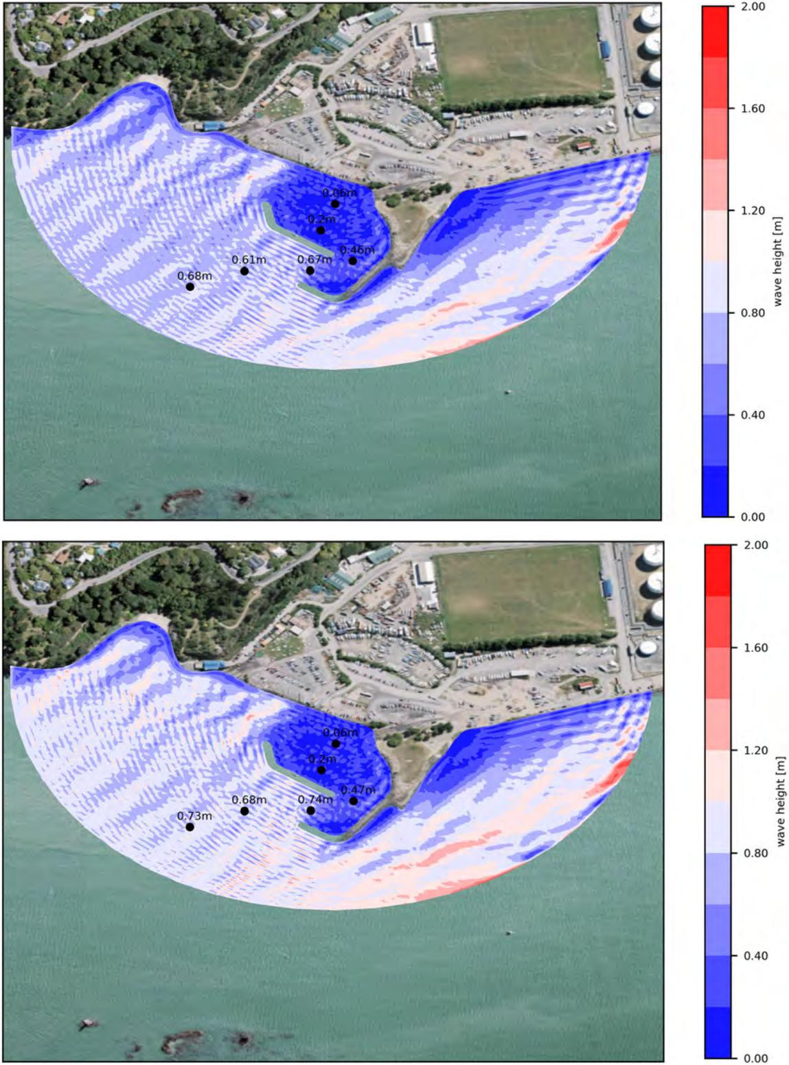
Figure 3.24 Wave height modelled for design layout 2 with South-westerly waves:  $H_s=0.73\text{m}$ ;  $T_p=3\text{s}$  (5 year return period, top panel) and  $H_s=0.80\text{m}$ ,  $T_p=3\text{s}$  (50 year return period, bottom panel),
