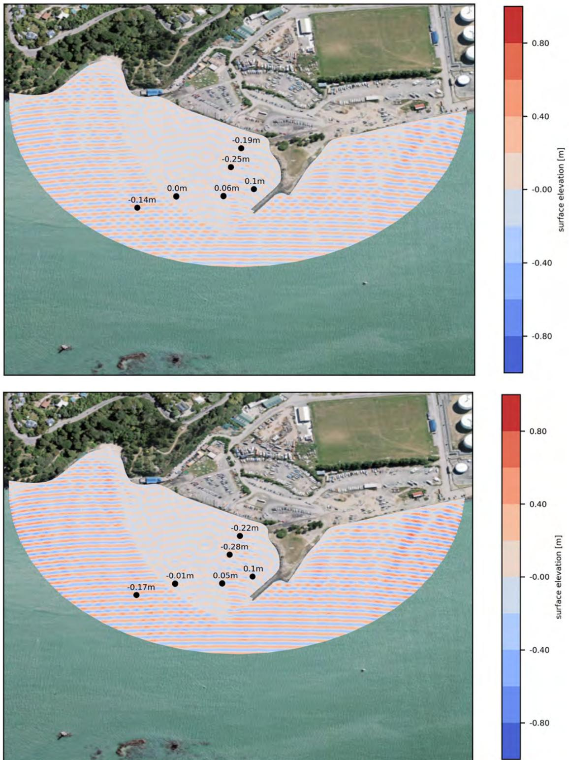
Figure 3.14 Surface elevation modelled for design layout 1 with Southerly waves:  $H_s=0.53\text{m}$ ;  $T_p=3\text{s}$  (5 year return period, top panel) and  $H_s=0.72\text{m}$ ,  $T_p=3\text{s}$  (50 year return period, bottom panel).
