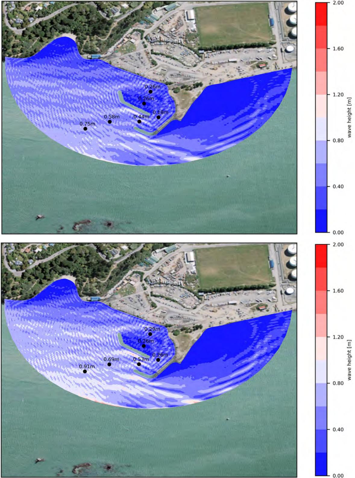
Figure 3.26 Wave height modelled for design layout 2 with Westerly wave s:  $H_s=0.54\text{m}$ ;  $T_p=3\text{s}$  (50 year return period, top panel) and  $H_s=0.65\text{m}$ ,  $T_p=3\text{s}$  (50 year return period, bottom panel).
