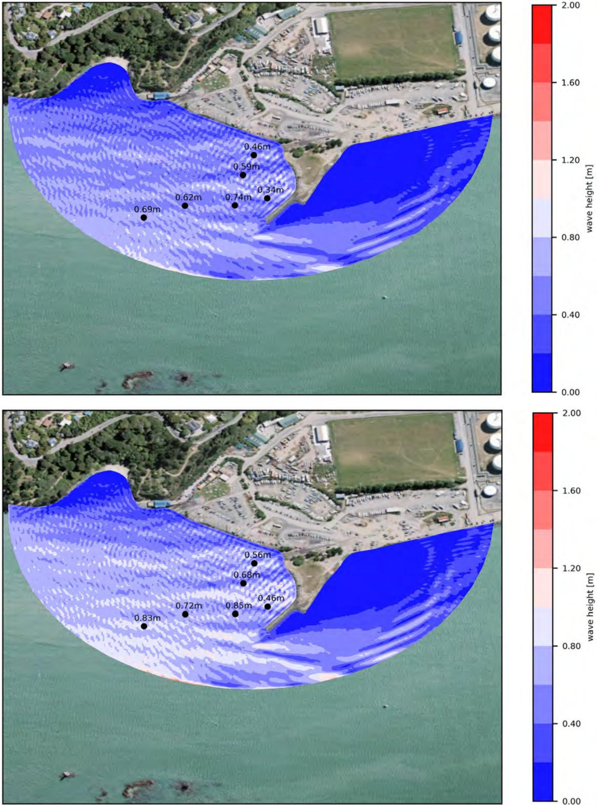
Figure 3.11 Wave height modelled for existing layout with Westerly waves:  $H_s=0.54\text{m}$ ;  $T_p=3\text{s}$  (5 year return period, top panel) and  $H_s=0.65\text{m}$ ,  $T_p=3\text{s}$  (50 year return period, bottom panel).
