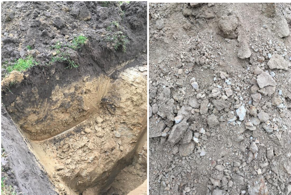
Figure 19: Test Pit G - test pit (left) and material indicative of subsoil (right).
