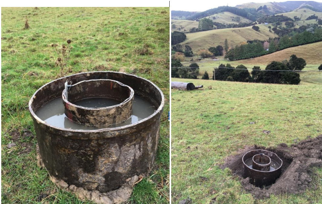
Figure 5: Infiltration Test ITG (left) and subsurface Test ITG.5 (right) within Paul le Lievre land.
