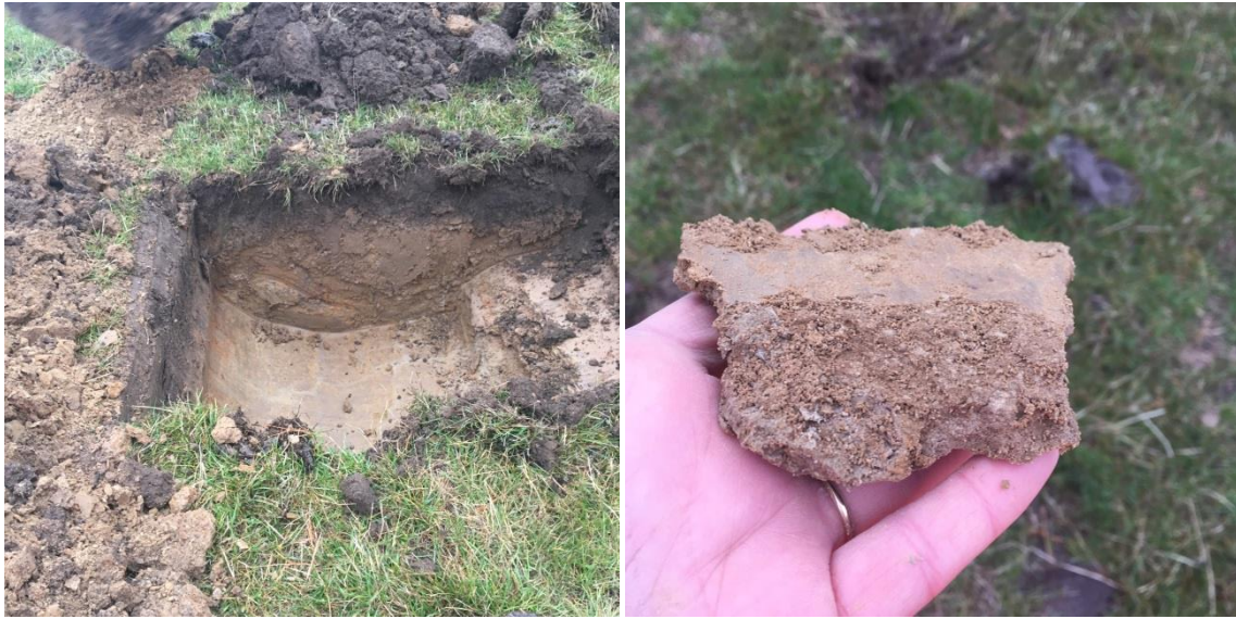
Figure 14: Test Pit 1 – test pit (left) and very firm layer at 1.3 m bgl (right).
