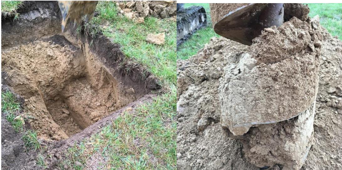
Figure 16: Test Pit 3 – test pit (left) and light grey material at 4.1 m bgl (right).
