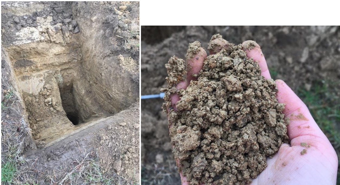
Figure 15: Test Pit 2 - test pit (left) and nutty/crumby silt material indicative of subsoil (right).
