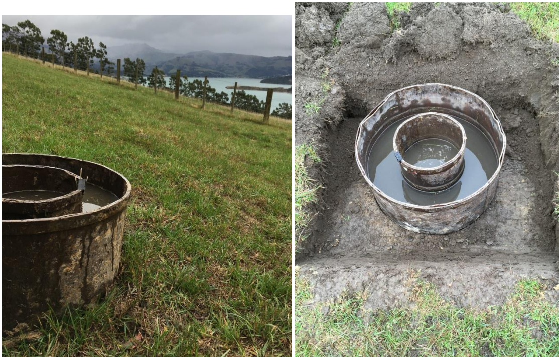
Figure 3: Infiltration Test IT3 (left) and subsurface Test IT3.5 (right) within CCC road corridor.
