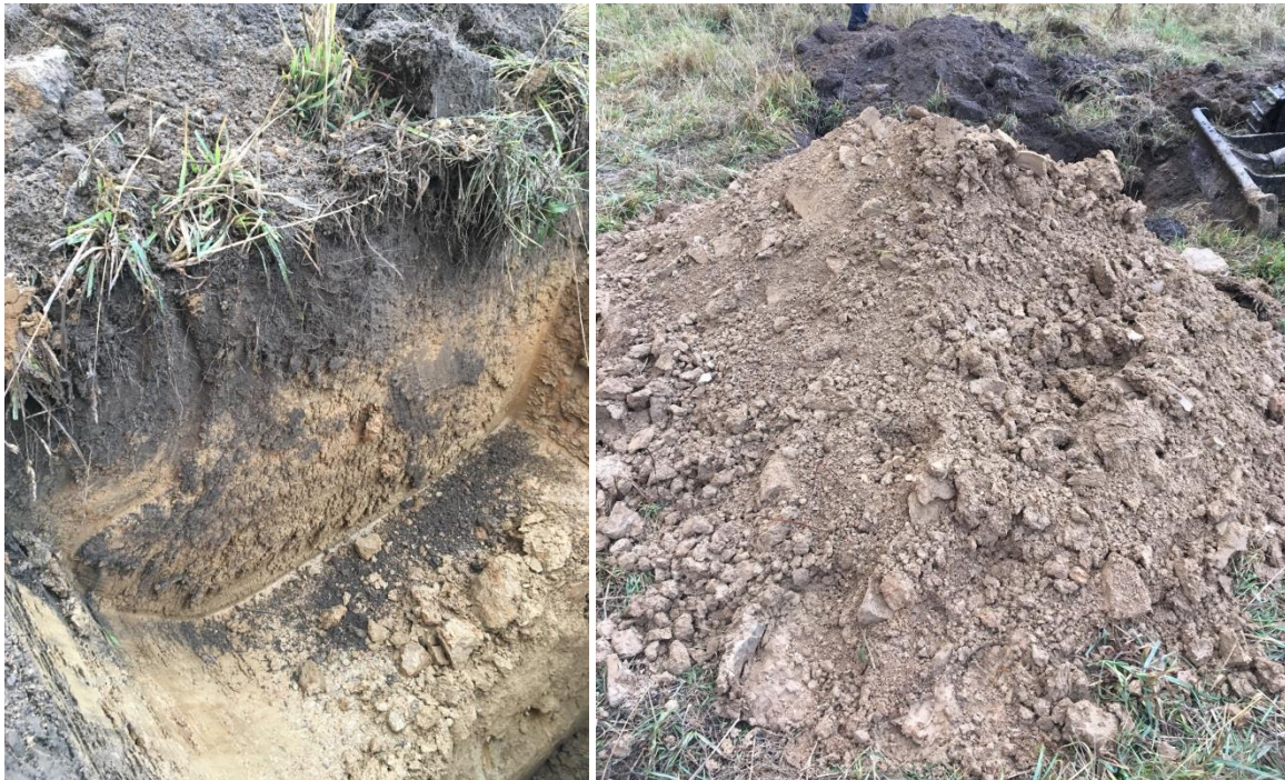
Figure 17: Test Pit 4 - test pit (left) and nutty/crumby silt material indicative of subsoil (right).
