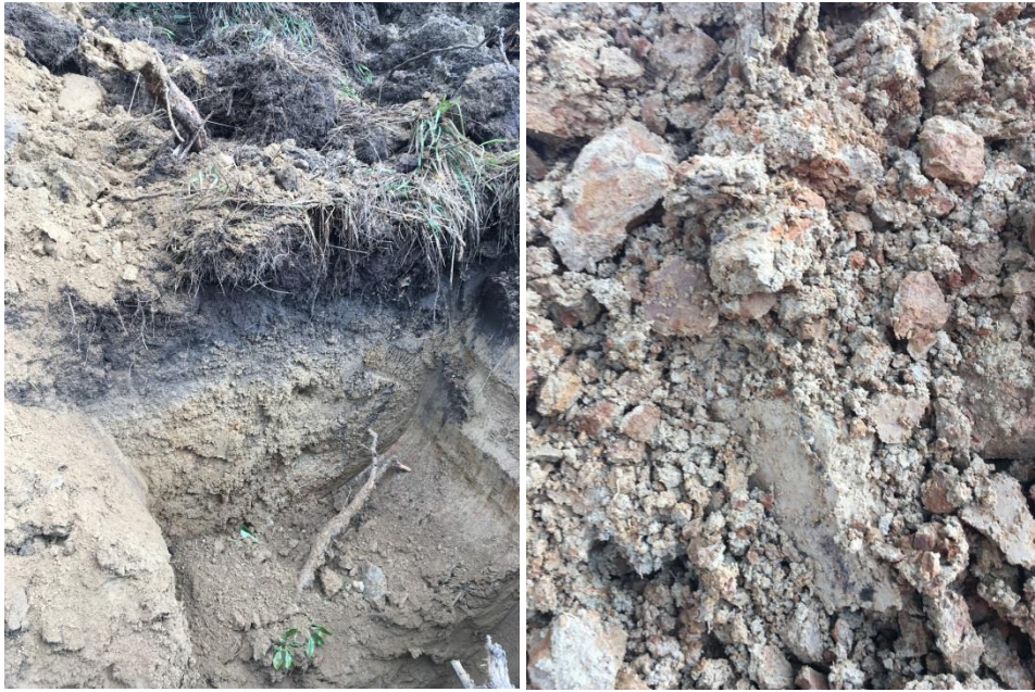
Figure 18: Test Pit 6 - test pit (left) and nutty/crumby silt material indicative of subsoil (right).
