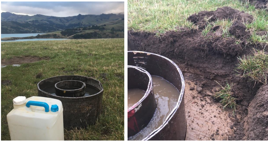
Figure 2: Infiltration Test IT1 (left) and subsurface Test IT1.5 (right) within Children's Bay land.
