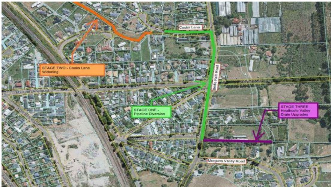
**Stage One** Pipeline diversion from Heathcote Valley drain down Bridle Path Road and into Cooks Lane waterway - this is currently being completed.
