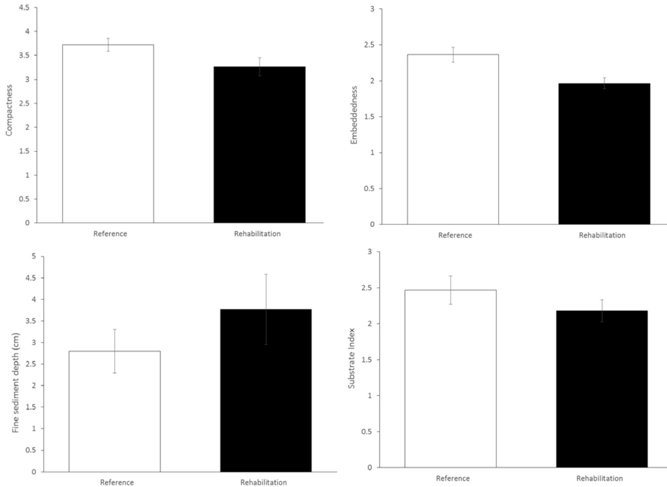
**Figure 3.** Average compactness (top, opposite page), embeddness (bottom, opposite page), Substrate Index (top, this page) and fine sediment depth (cm) (bottom, this page) recorded at the reference and rehabilitation sites along the Avon River. Error bars are  $1 \pm SE$ .
