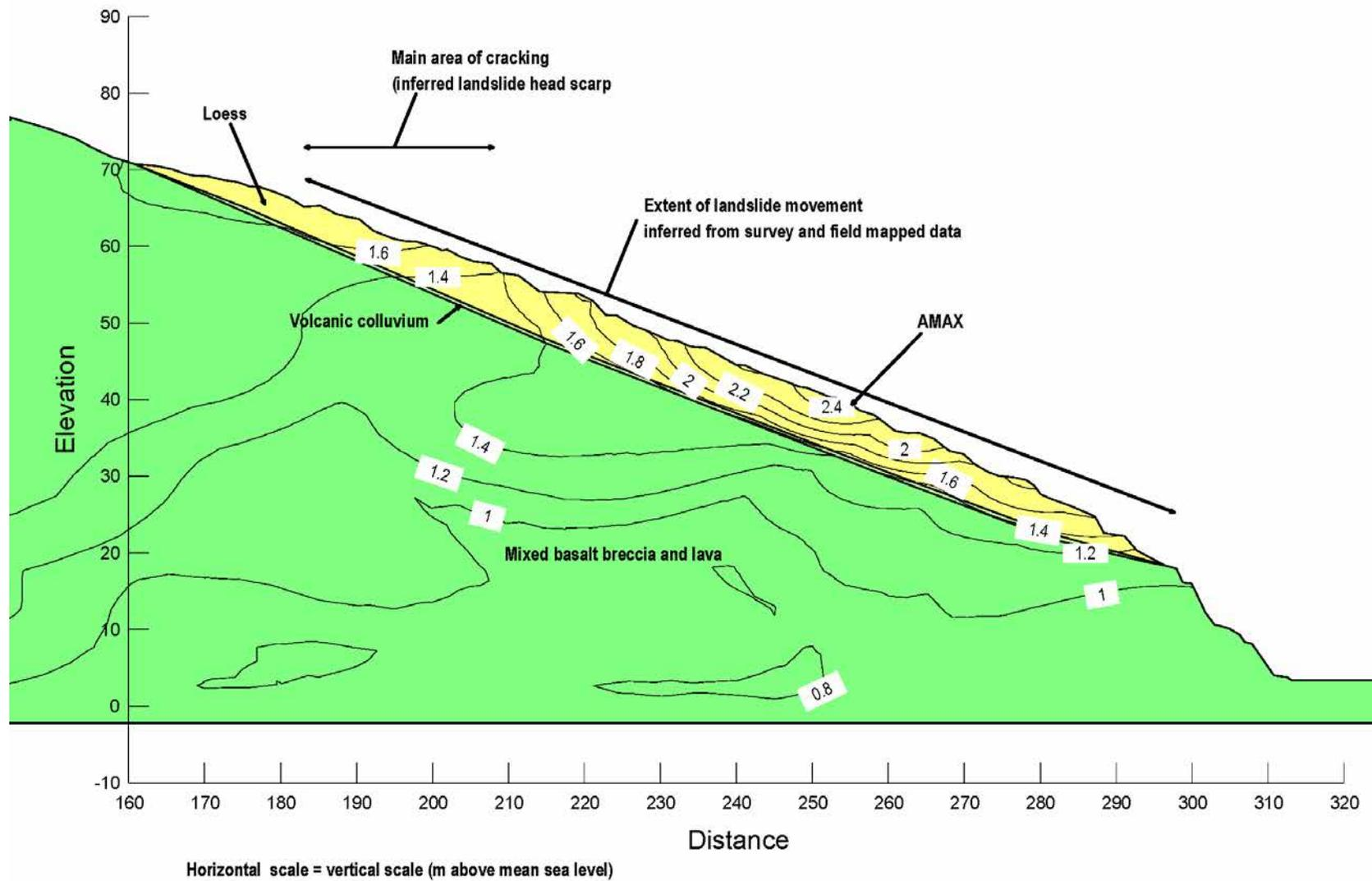
**Figure A4.2** Modelled peak horizontal ground acceleration contours for the 22 February 2011 earthquake at Maffey's Road, cross-section 4.
