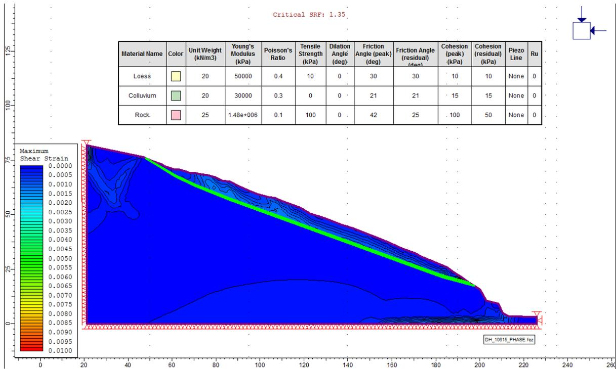
**Figure 18** Failure mechanism 2. Example of limit equilibrium and finite element modelling results for cross-section 1, representing source area 1, for failure through the colluvium layer.
