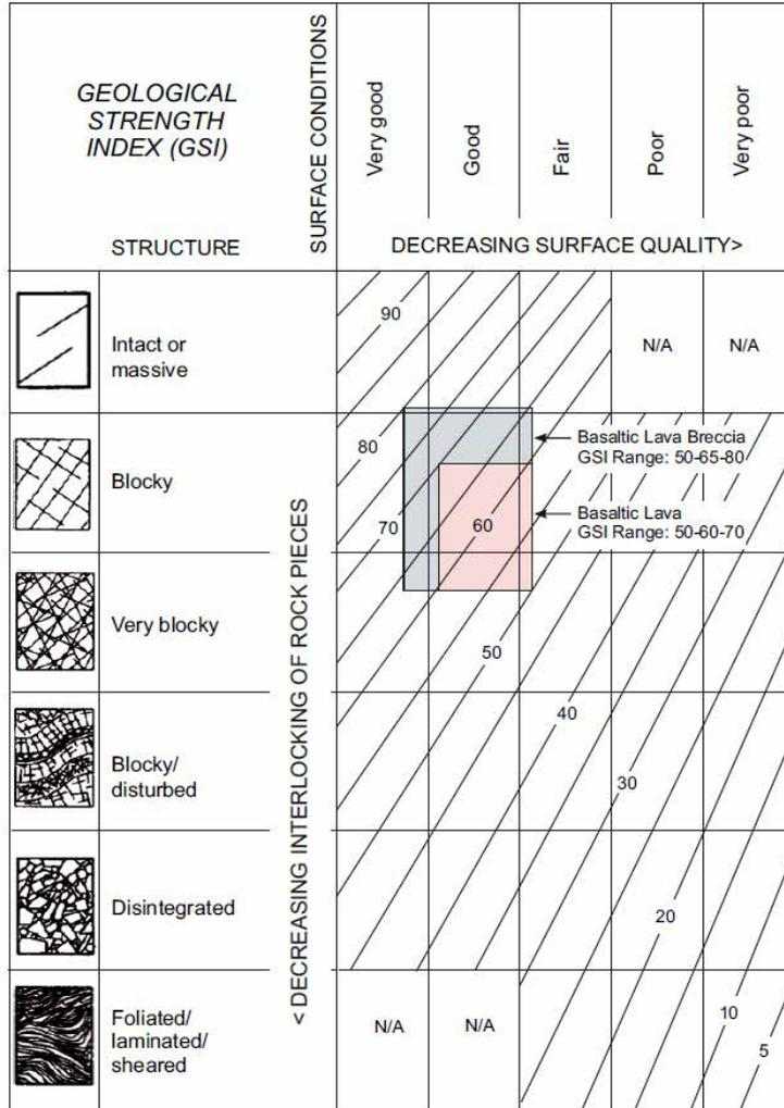
Figure 13 Geological strength index plot for volcanic breccia at Deans Head (modified after Hoek, 1999).
