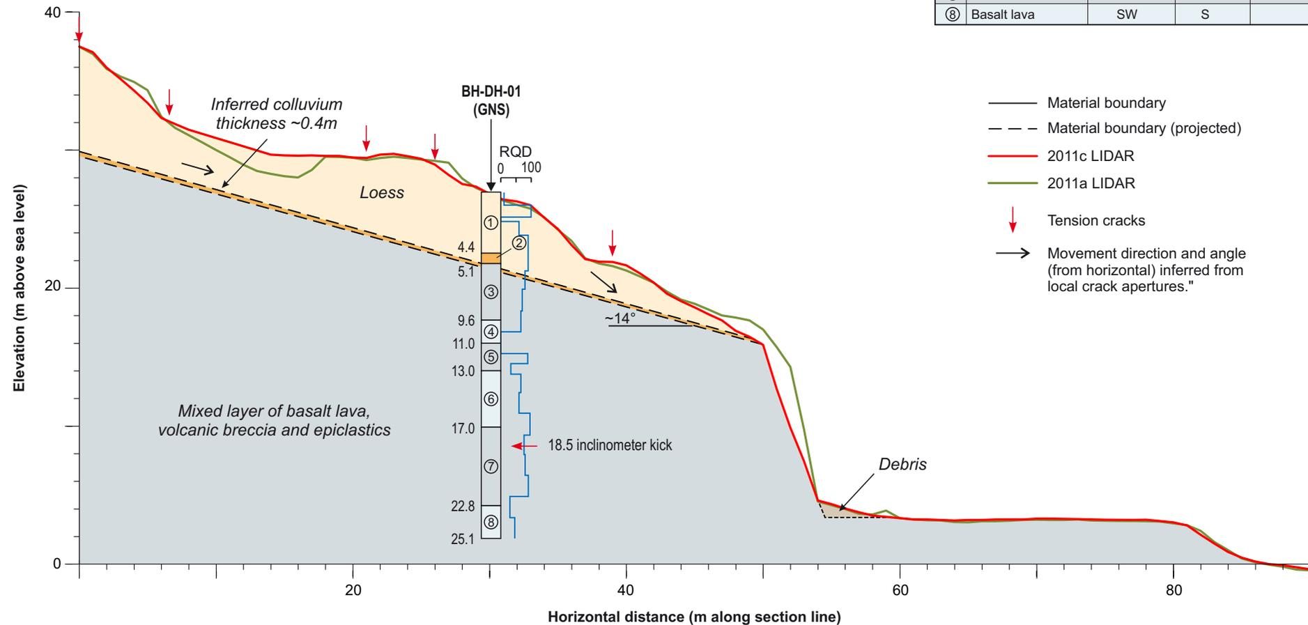
Weathering (adopting NZGS (2005) terminology): CW completely weathered; HW highly weathered; MW moderately weathered; SW slightly weathered; UW unweathered.
