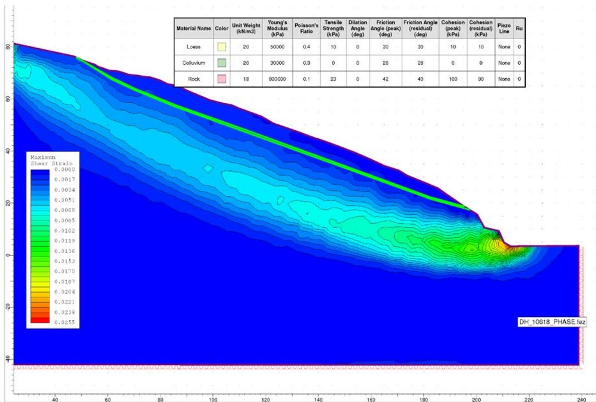
**Figure 19** Failure mechanism 3. Example of limit equilibrium and finite element modelling results for cross-section 1, representing source area 1, for failure mechanism through the rock.
