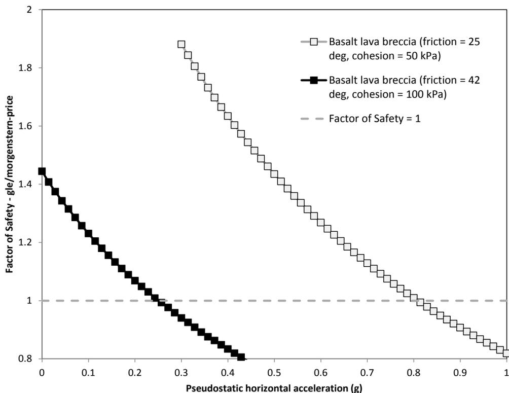
**Figure 28** Yield acceleration of the slope based on variable fill parameters and loess parameters shown in Table 11. Yield acceleration calculated adopting the pseudostatic method (Kramer, 1996).
