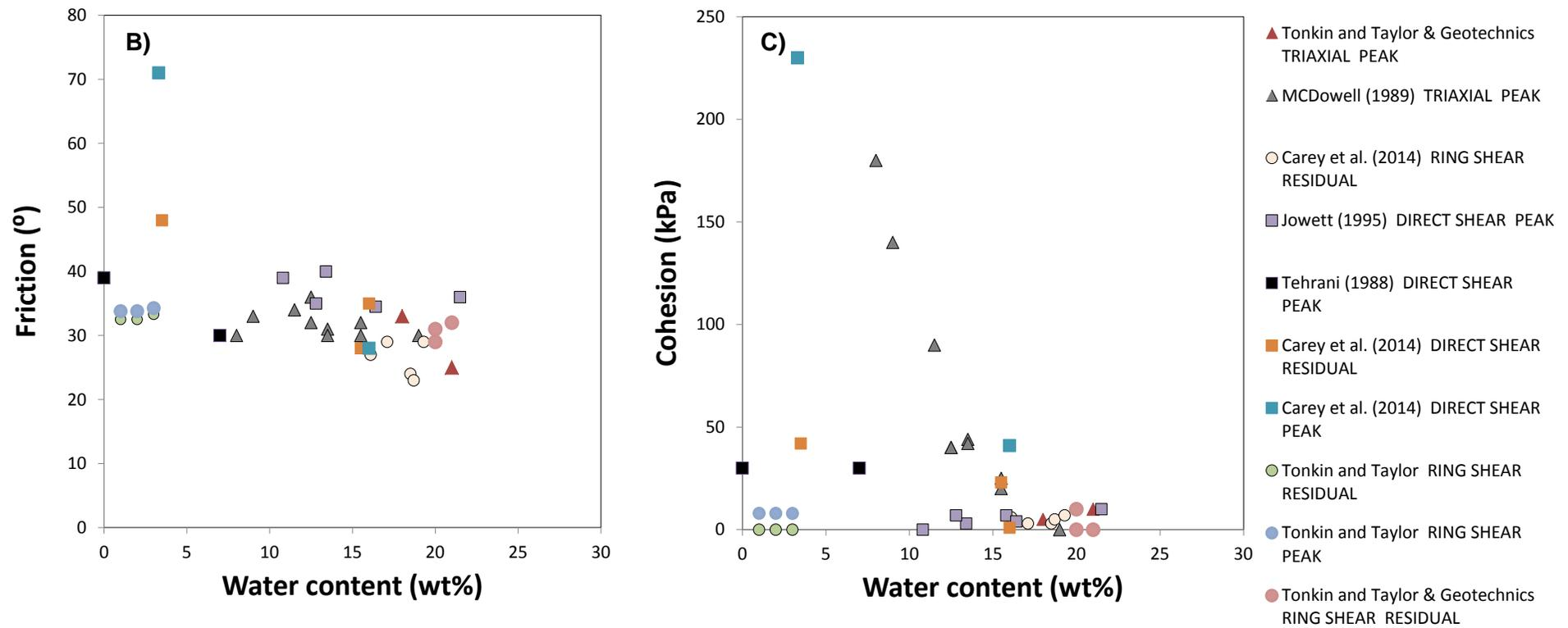
**Figure 10** Loess residual shear strength results (from Table 8 and Table 9). A) Cohesion and friction laboratory results plotted for loess. B) Loess residual cohesion plotted against water content. C) Loess residual friction plotted against water content.
