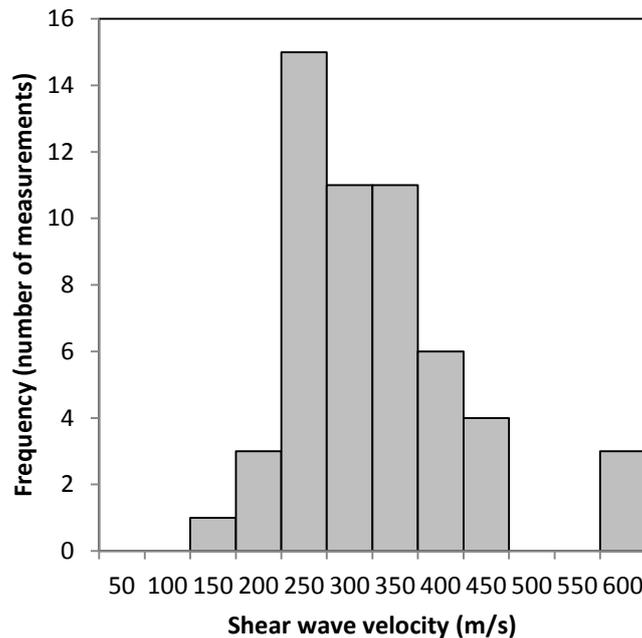
**Figure 12** Loess and colluvium shear wave velocity results from dynamic probing reported by Tonkin and Taylor (2012a) for the loess at Clifton Terrace.
