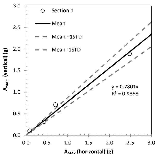
**Figure A4.3** Relationship between the modelled horizontal and vertical maximum accelerations modelled at the convex break in slope ( $A_{MAX}$ ) for cross-section 1, using the synthetic free-field rock outcrop motions for the Deans Head site by Holden et al. (2014) as inputs to the assessment. The mean and standard deviation trend lines are fitted for  $A_{MAX}$  all data. Errors are shown as the mean  $\pm$  one standard deviation (1 STD).
