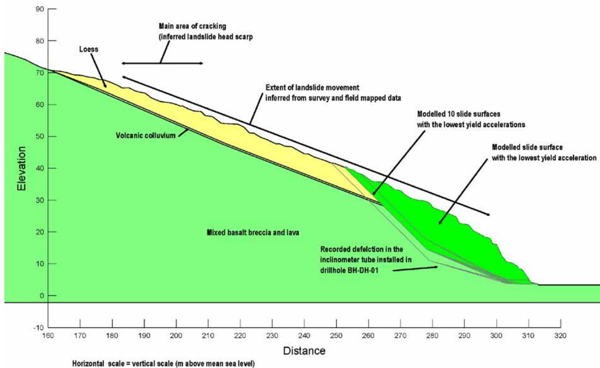
**Figure 26** Results from the seismic slope stability assessment for failure mechanism 3, cross-section 1, for the 22 February 2011 earthquake.
