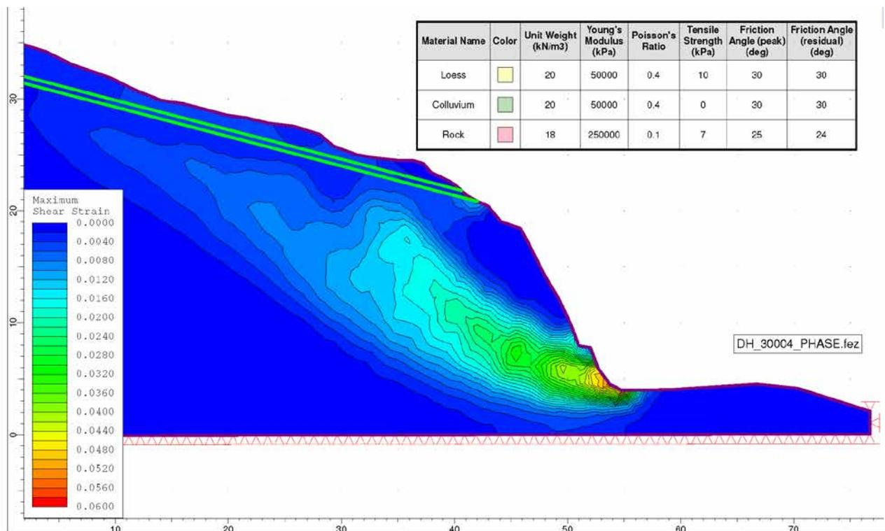
**Figure 20** Failure mechanism 3. Example of limit equilibrium and finite element modelling results for cross-section 3, for failure mechanism through the rock.
