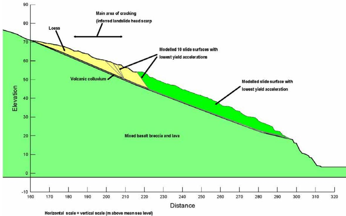
**Figure 25** Results from the seismic slope stability assessment for failure mechanism 2, cross-section 1, for the 22 February 2011 earthquake.
