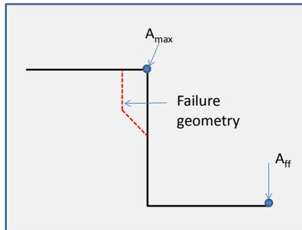
**Figure A4.1** Amplification relationship between the synthetic free-field rock outcrop input motions ( $A_{FF}$ ) and the modelled cliff crest maximum accelerations ( $A_{MAX}$ ) for cross-section 1. A schematic diagram showing the locations of the various recorded accelerations is shown.
