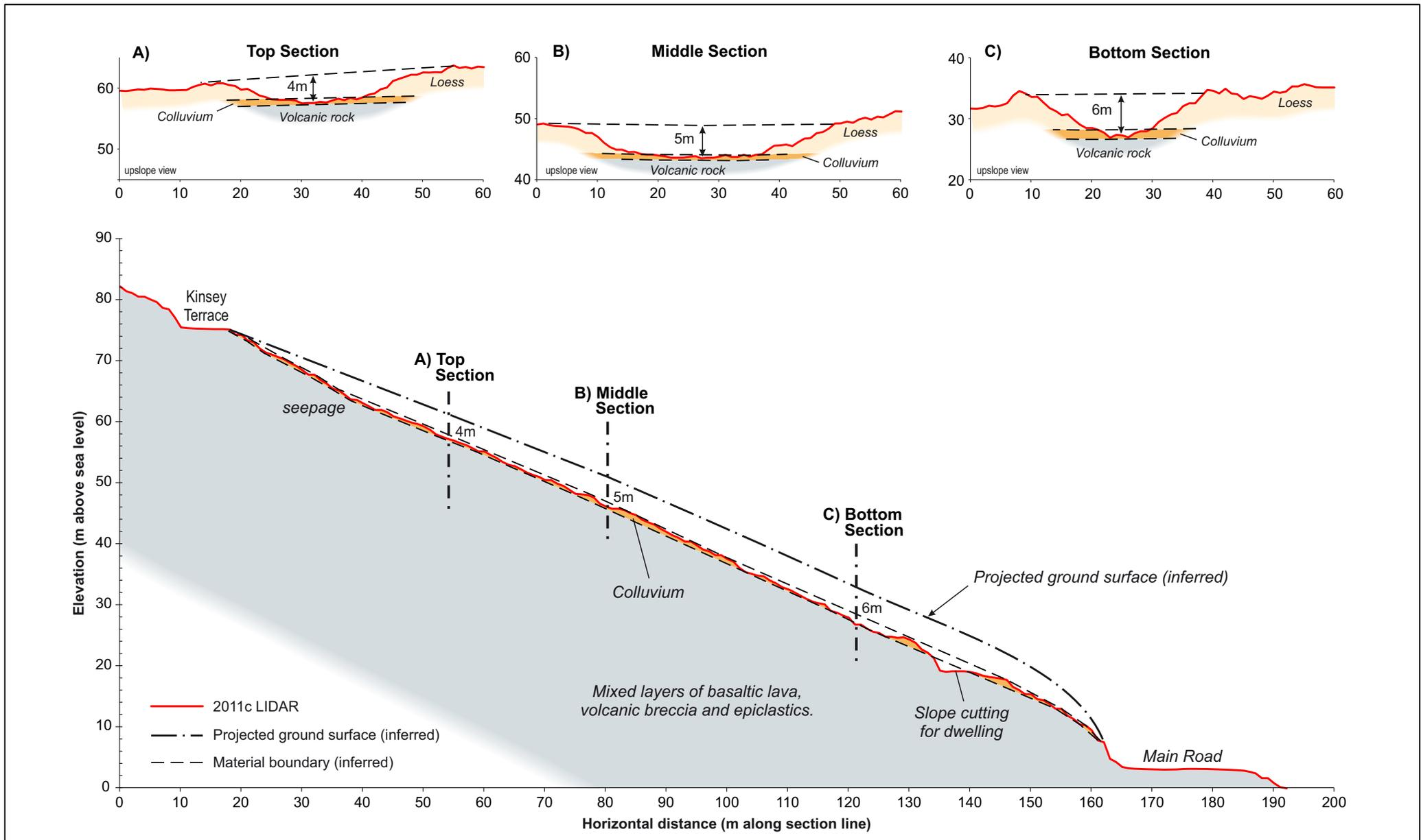
1) Projected ground surface is inferred by projecting ground surface from section A), B) and C)
