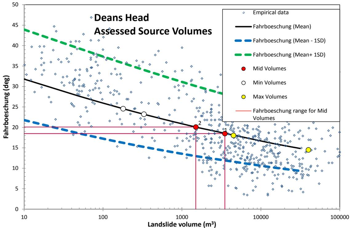
**Figure 30** Estimation of debris flow fahrboeschung angles based on empirical runout data presented in Massey and Carey (2012).
