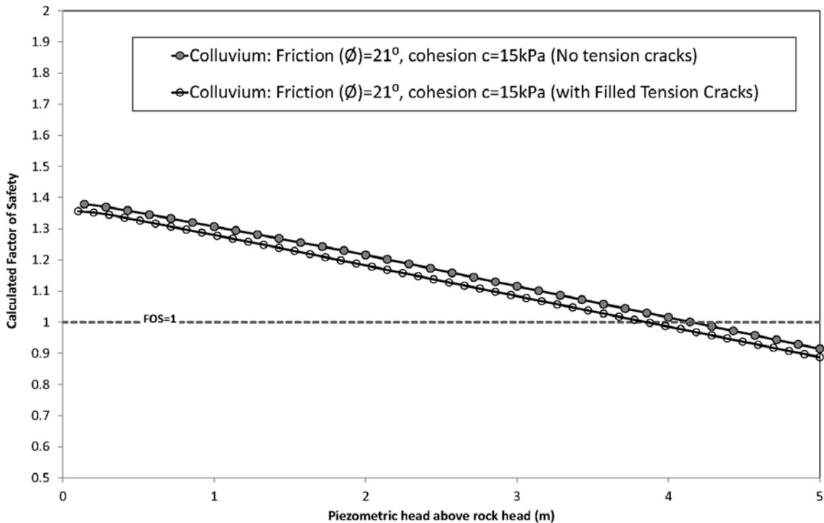
**Figure 22** Sensitivity assessment of the slope factor of safety (source area 1) in response to including filled tension cracks in the model. Tension cracks were assumed to be 100% filled.
