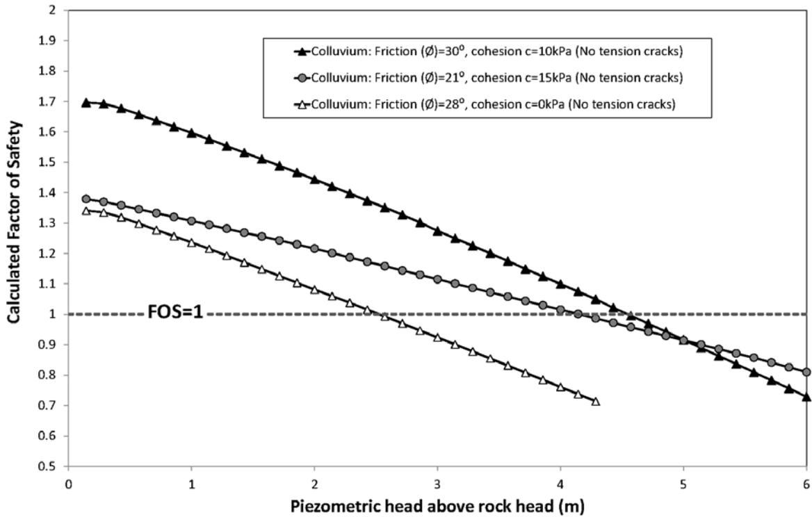
**Figure 21** Sensitivity assessment of the slope factor of safety (source area 1) in response to changing piezometric head levels above rock head for a range of colluvium strength parameters.
