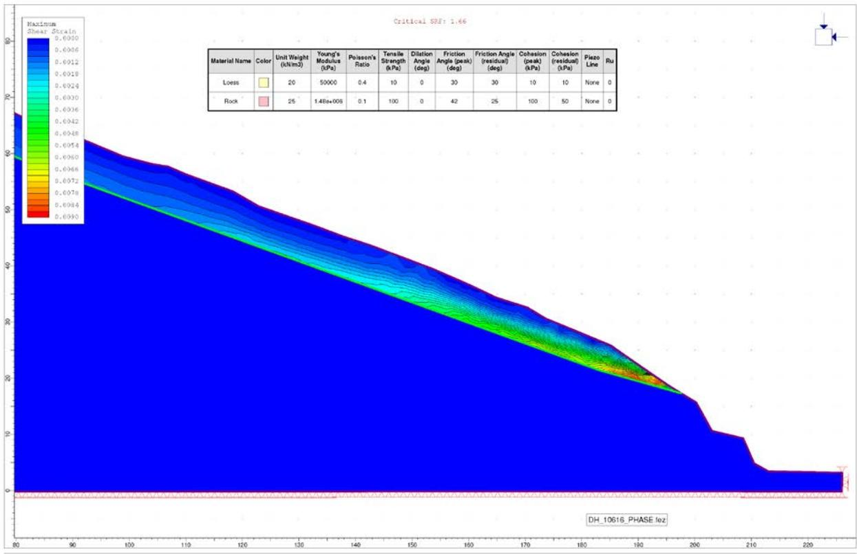
**Figure 17** Failure mechanism 1. Example of limit equilibrium and finite element modelling results for cross-section 1, representing failure of loess in source area 1.
