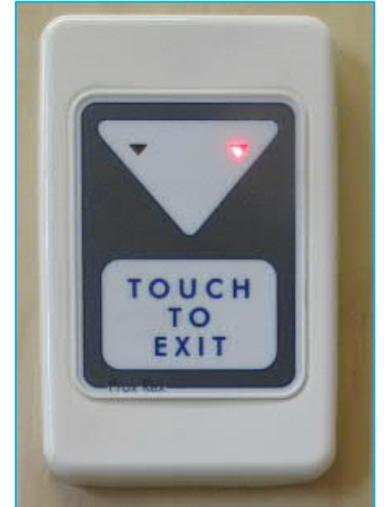
**EMERGENCY TYPE** – Use this only in an emergency, this type has a local alarm and will become noisy once pushed. This is not connected to the alarm system and can be deactivated by using a special tool.
