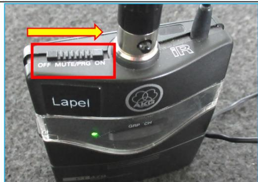
2. Turn on the lapel unit by sliding the switch all the way forward and the green light will illuminate to show it has turned on successfully
