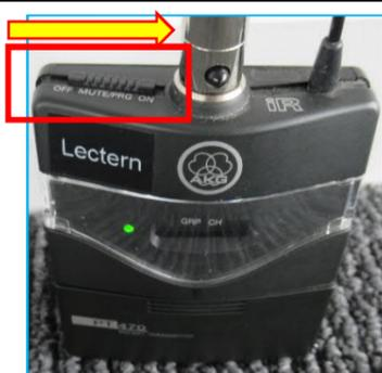
2. Turn on the "Lectern Pocket Transmitter Unit" by sliding the switch all the way forward and the green light will illuminate to show it has turned on successfully
