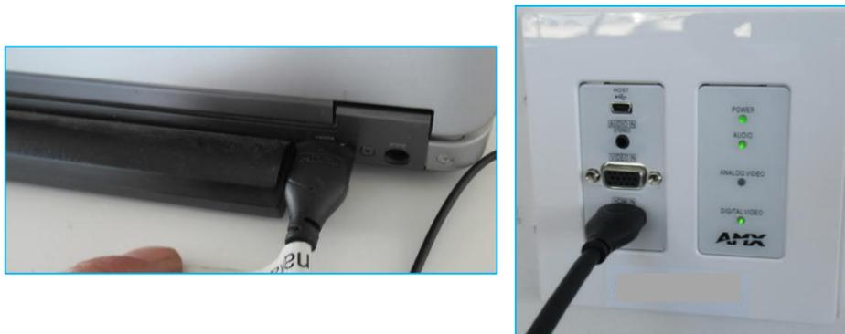
3. Connect the device to your HDMI cable and plug it into the "Wallplate"
