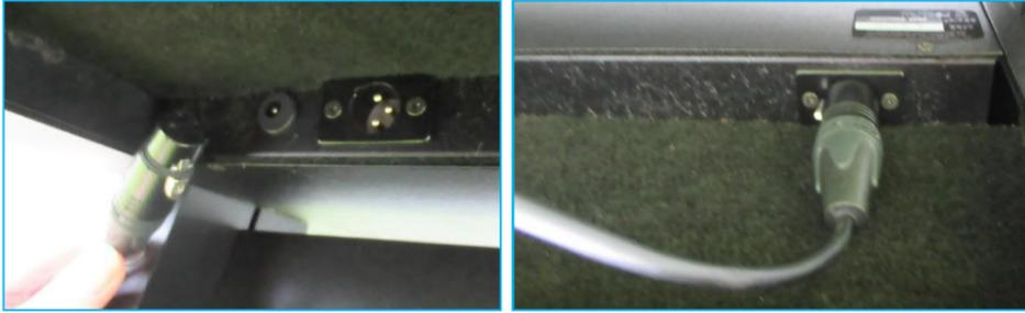
9. Connect the "Lectern Cable" to the underside of the lectern (If you want the mic on the RH side connect the cable to that side and vice versa if the LH side is required)
