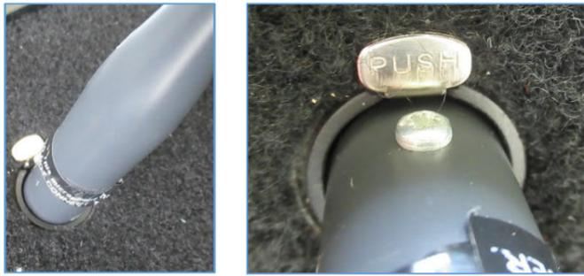
10. When you have finished, turn off the "Lectern Pocket Transmitter Unit" & remove the "Lectern mic" from the lectern by pushing the silver button marked "PUSH" at the base of the microphone. **Return all items to the service desk**
