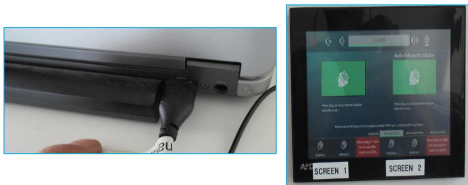
3. Connect the device to your HDMI cable and plug it into the chosen “Wallplate”
