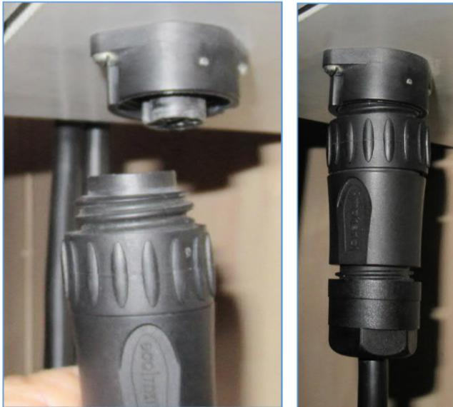
6. Insert plug-end into the socket and then screw the collar in until finger tight (Do not over tighten) this plug will only fits in one-way, move it around to find its seating position.
