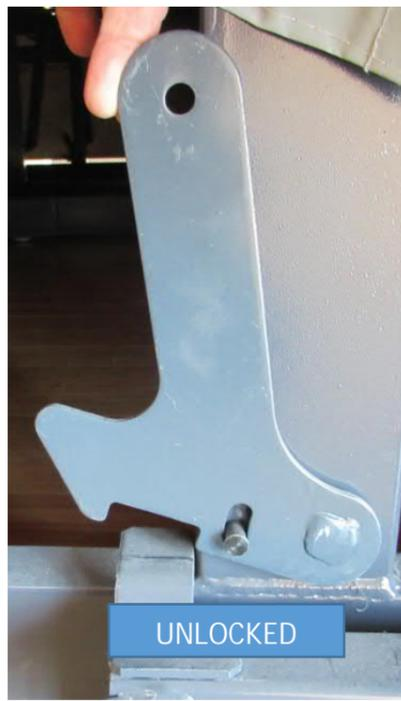
7. There are a series of brakes that automatically lock as the seating is extending. These are located on both sides of the seating. Please check these are in the locked position. If not repeat process of retracting and extending.
